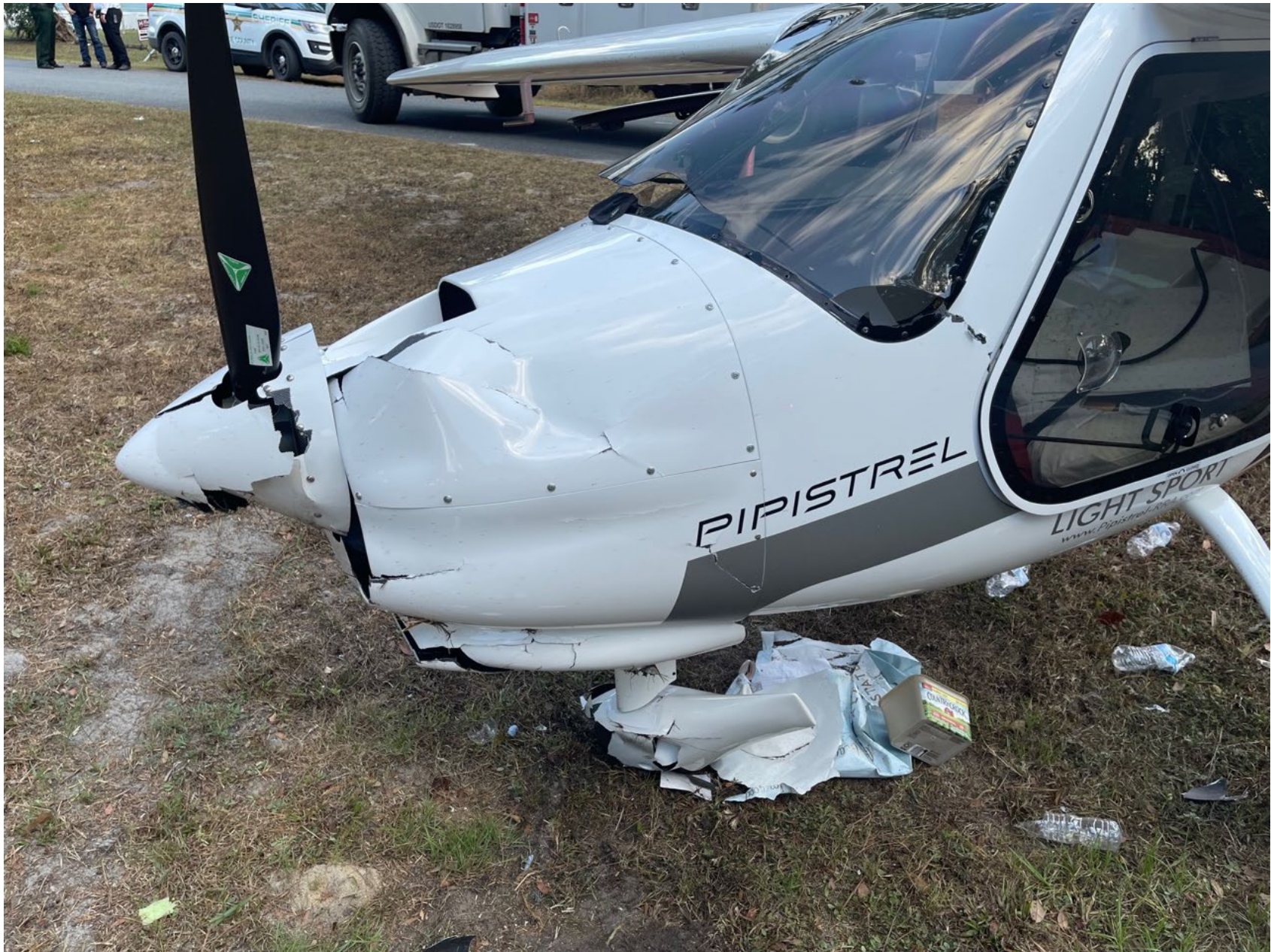
Photo 3 – Fuselage Damage (FAA Photo)
