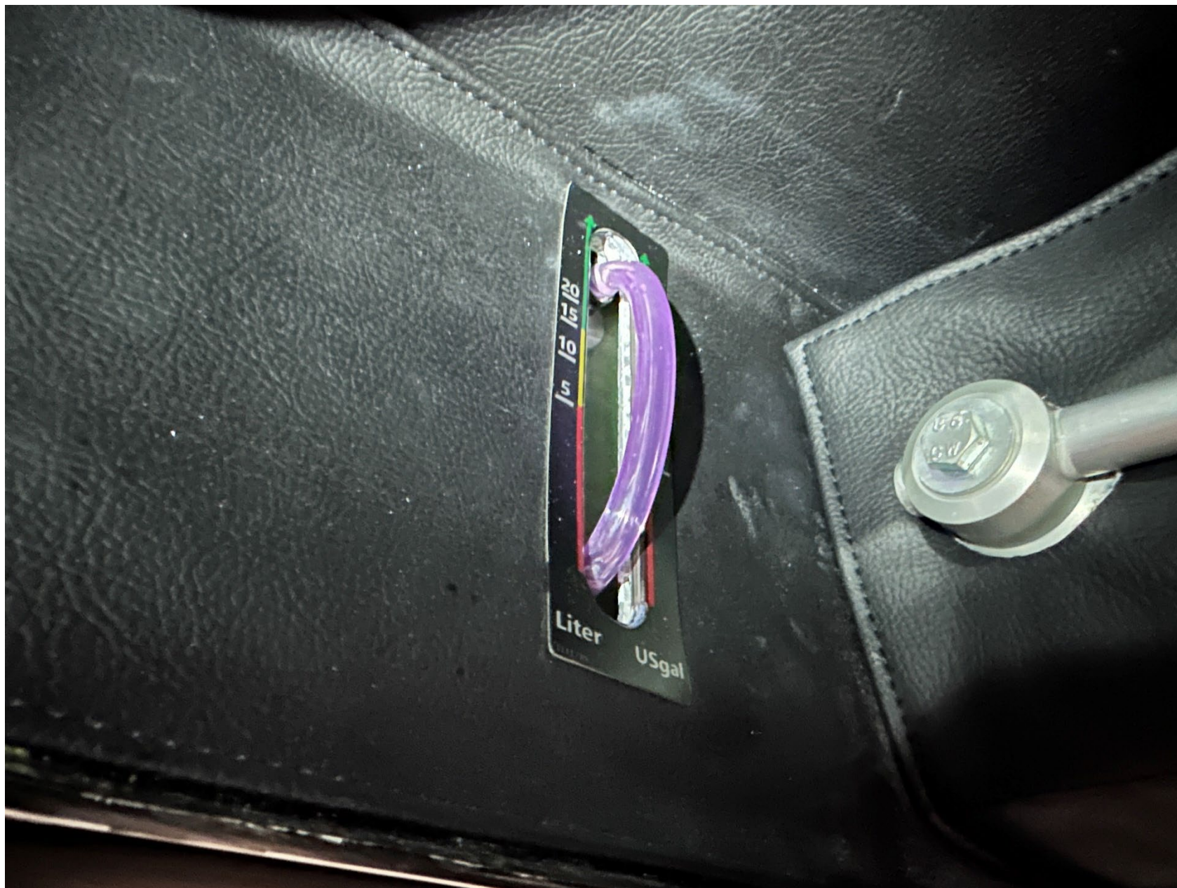
Photo 5 – Fuel Gauge Showing No Fuel (Right Rudder Aviation Photo)
