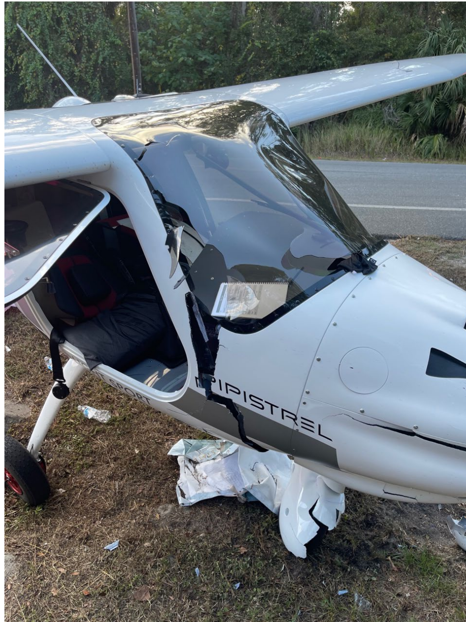
Photo 2 - Fuselage Damage (FAA Photo)
