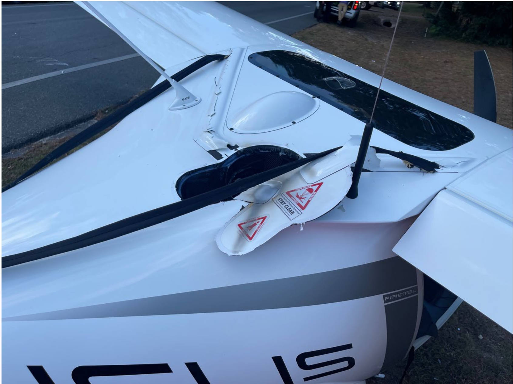
Photo 4 - Airframe Parachute Compartment and Mount (FAA Photo)
