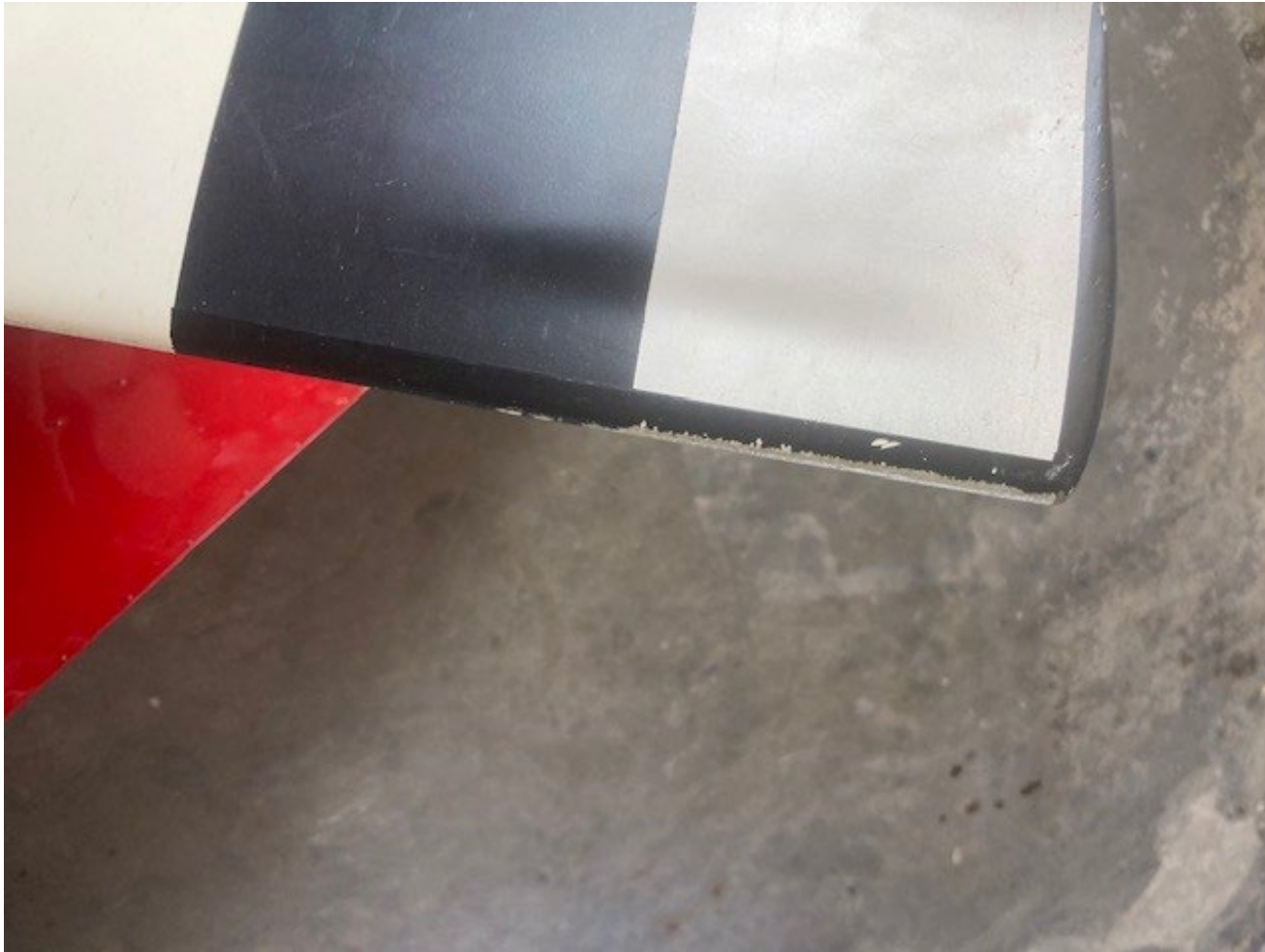
Photograph 2 - View of Tail Rotor Blade with Dent (Courtesy of Pilot)
