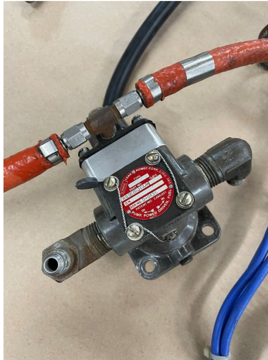
Figure 5: Fuel pump prior to functional testing.
