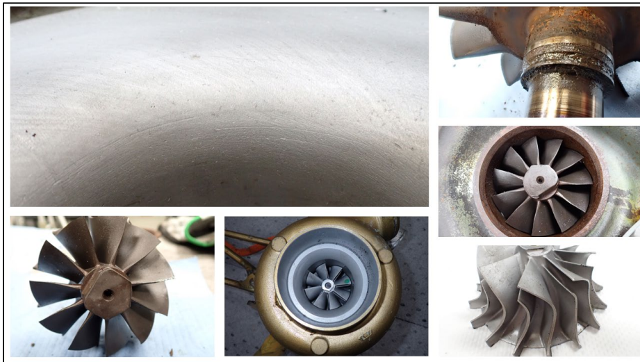
Figure 12: Turbo examination photographs. Note rotational scoring in top left.
