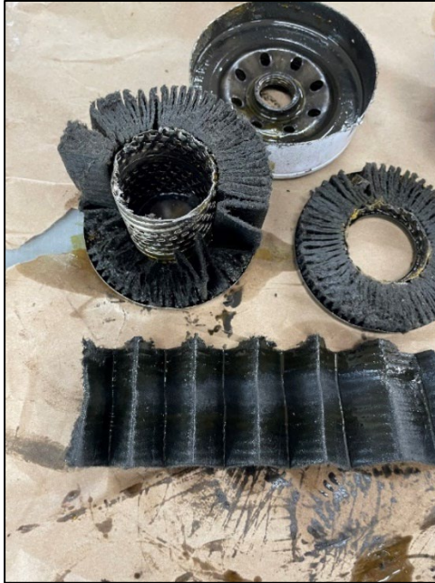
Figure 9: Opened oil filter and pleats.
