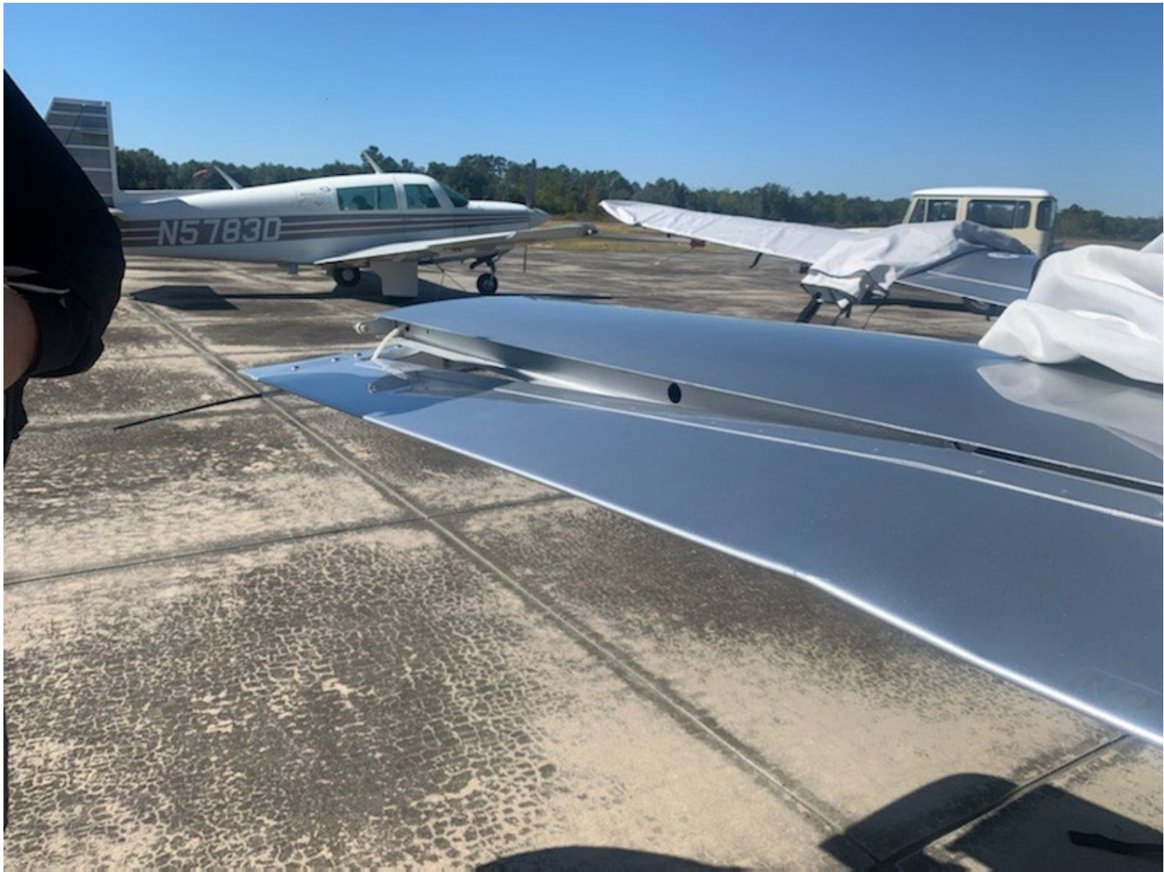
Photo 1 – Damage to left elevator (Pilot Photo)
