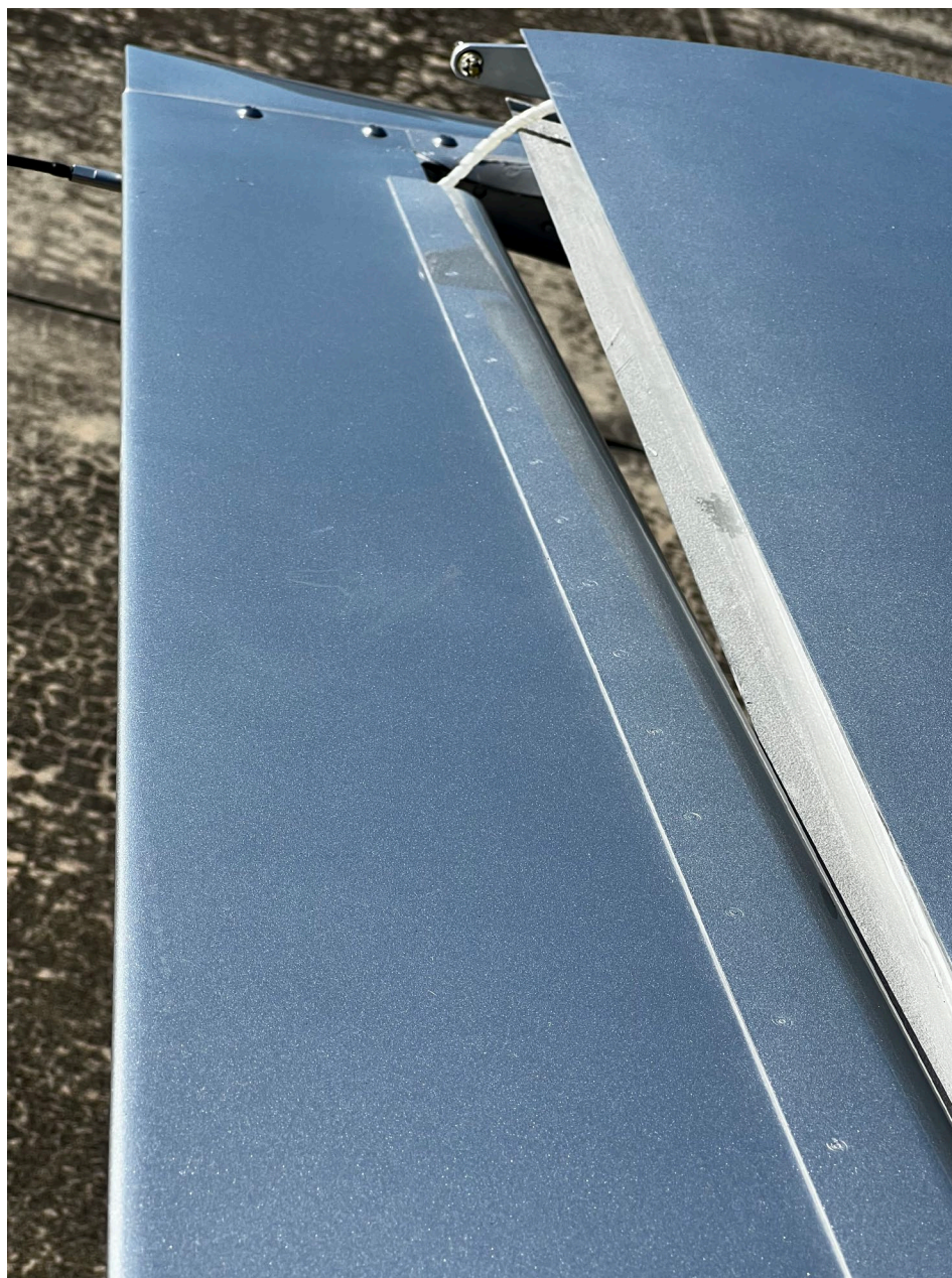
Photo 2 - Damage to left elevator (Pilot Photo)
