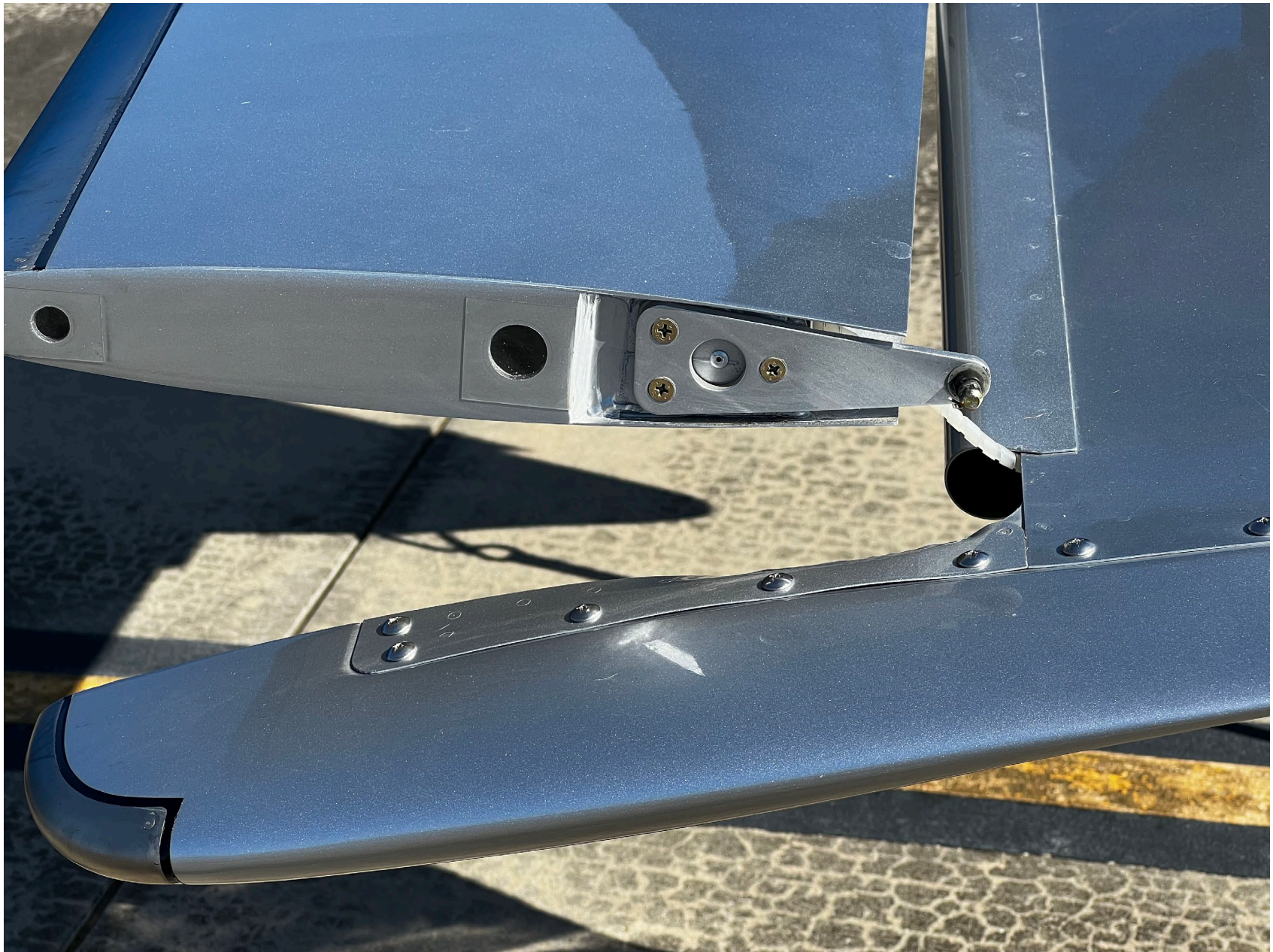
Photo 3 - Damage to left elevator (Pilot Photo)
