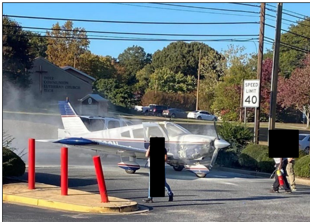
Figure 1: View of airplane shortly after landing showing the thermal damage (Photo Courtesy of FAA).
