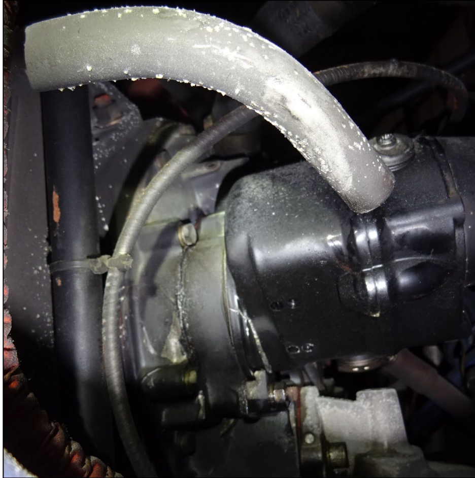
Figure 4: View the left magneto displaced from its attachment area.
