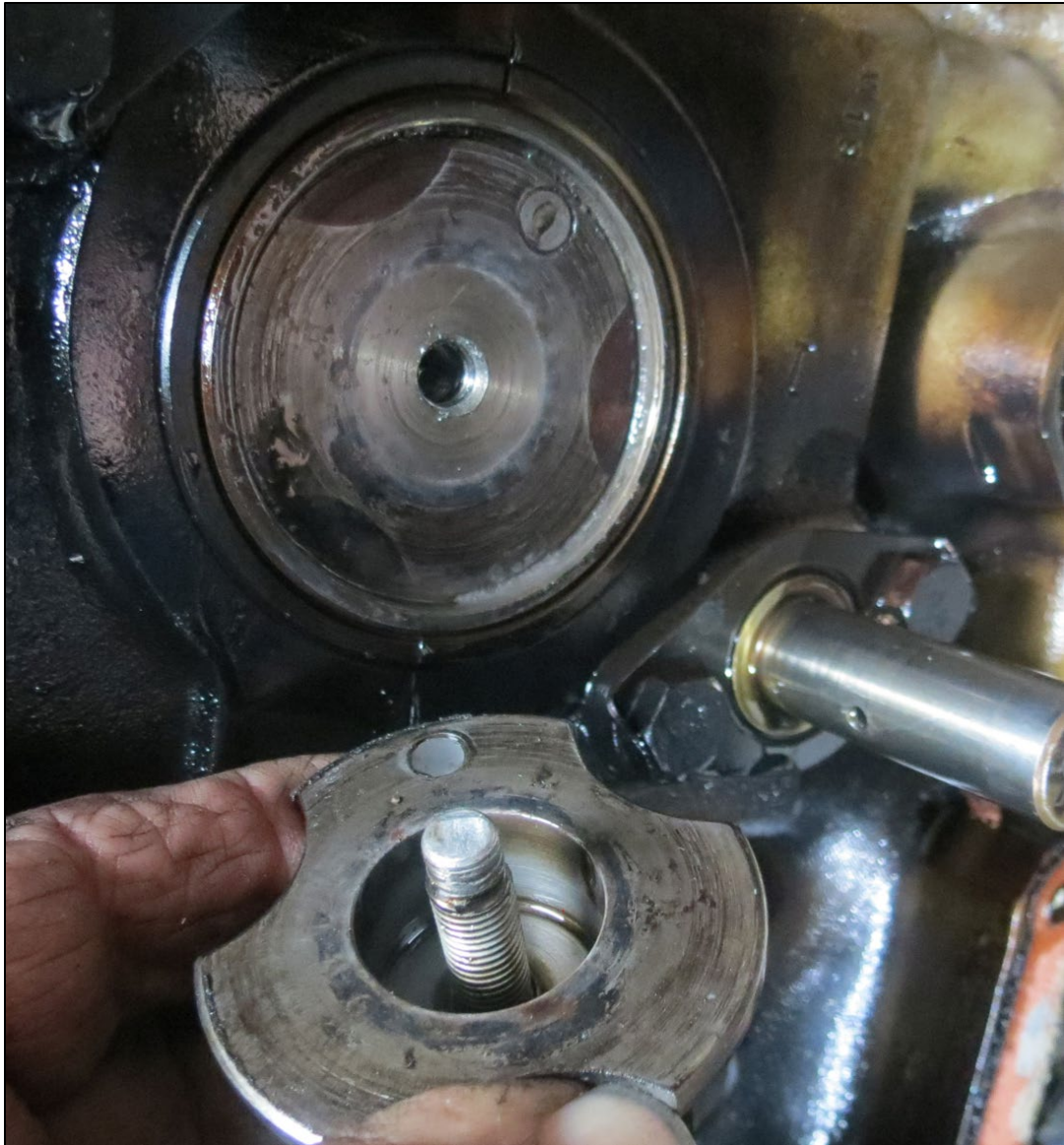
Figure 9: Crankshaft drive gear bolt removed. Note the dowel pin had sheared.
