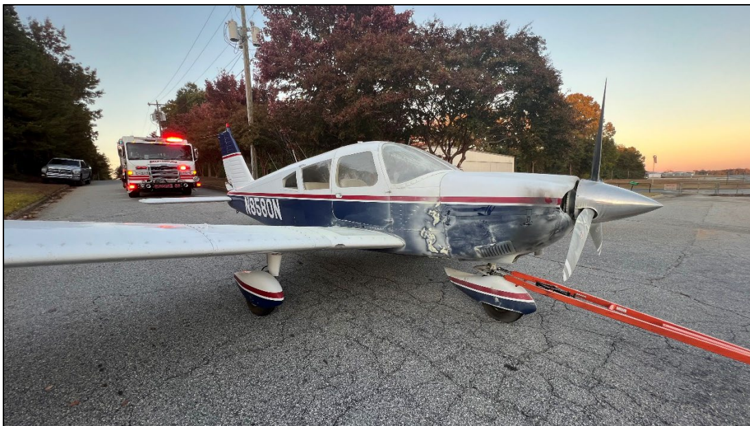
Figure 3: View of the thermally damaged engine compartment and cowling area (Photo Courtesy of FAA).
