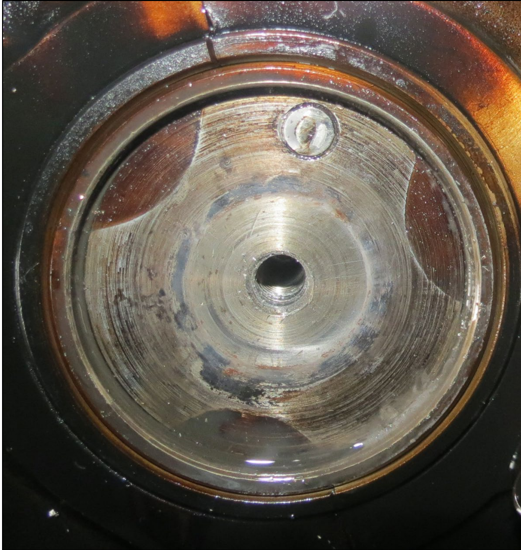
Figure 10: View of the dowel pin and crankshaft drive gear attachment area.
