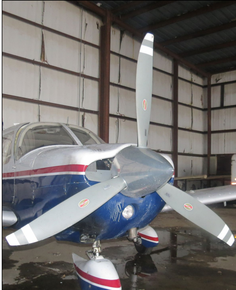
Figure 11: Thermal damage noted to the propeller oriented upward.
