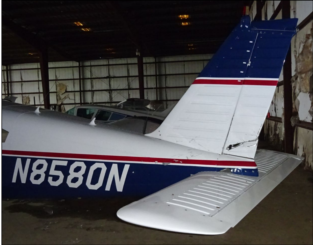
Figure 6: View of the substantially damaged rudder.
