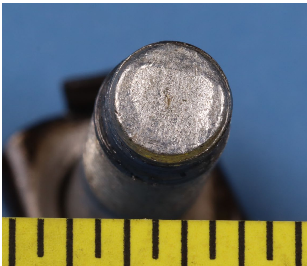
Figure 4. Close-up photo showing the end face of the crankshaft drive gear bolt.
