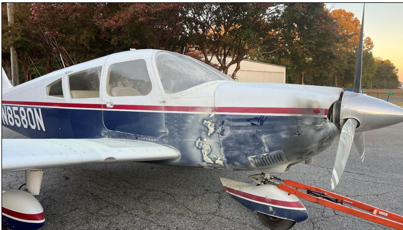
Photograph 2 - Image of the thermally damaged cowling (Courtesy of FAA)
