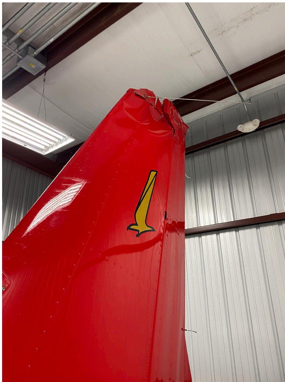
Photo 7 – Vertical stabilizer and rudder damage (FAA Photo)
