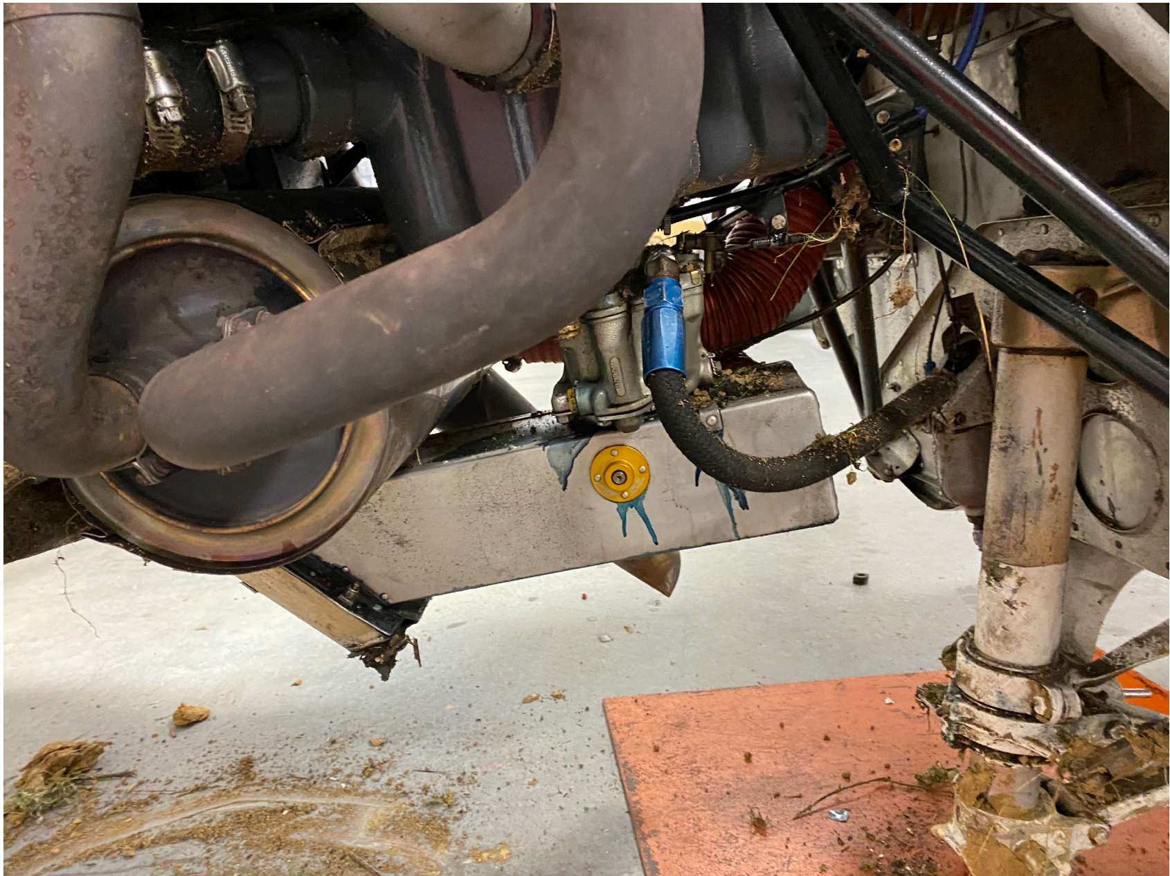
Photo 3 – Engine Mount Damage (FAA Photo)
