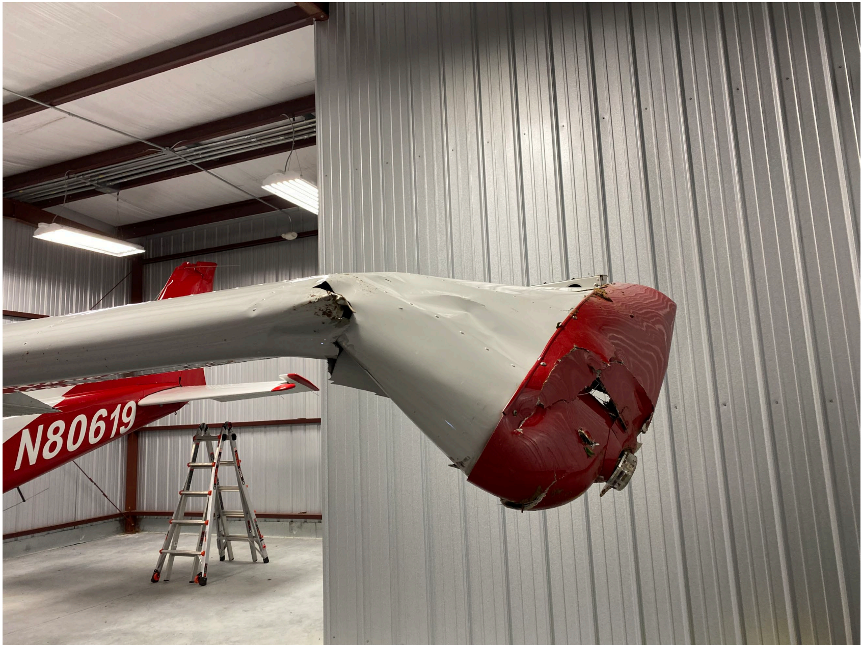
Photo 4 – Left wing damage (FAA Photo)
