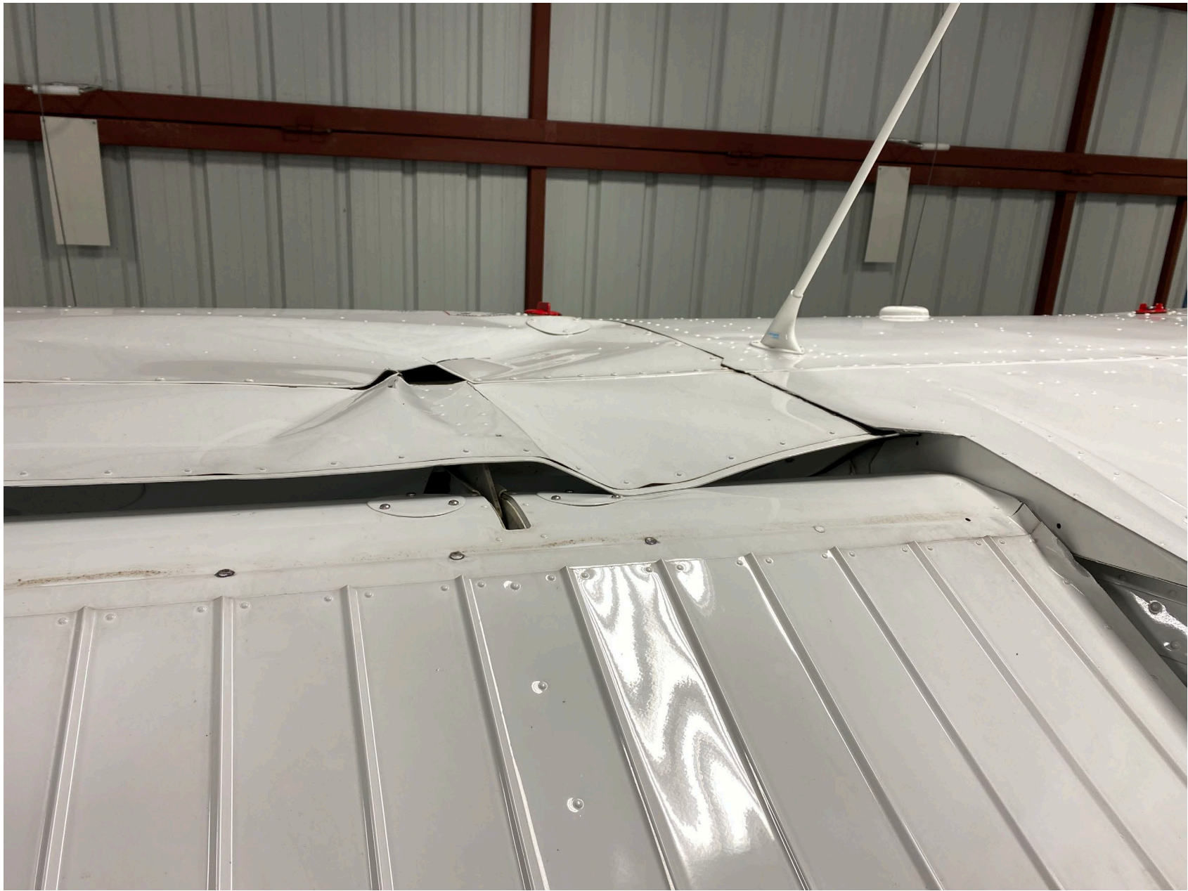
Photo 6 – Left wing damage (FAA Photo)
