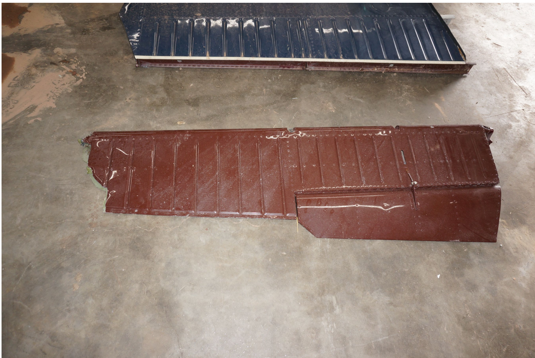
Photograph 4 - Damaged ruddervator (NTSB)
