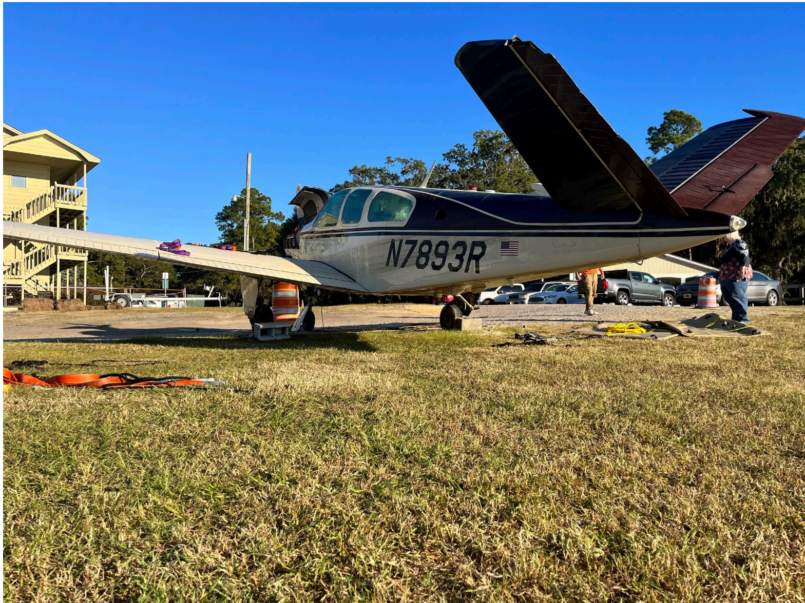
Photograph 2 - Airplane from aft left, note damage to ruddervator (Courtesy of FAA)
