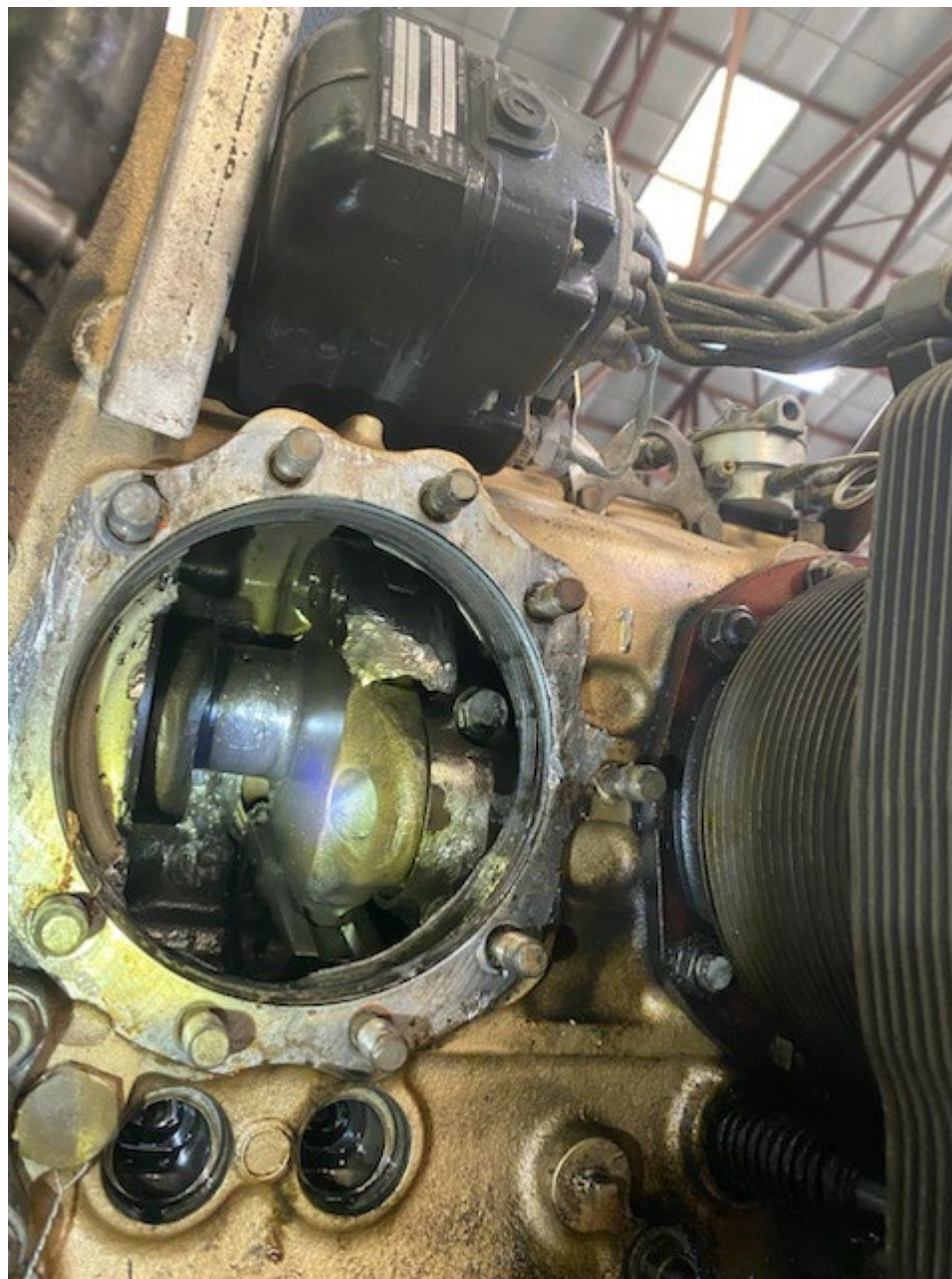
Photo 3 – Discolored crankshaft (FAA)
