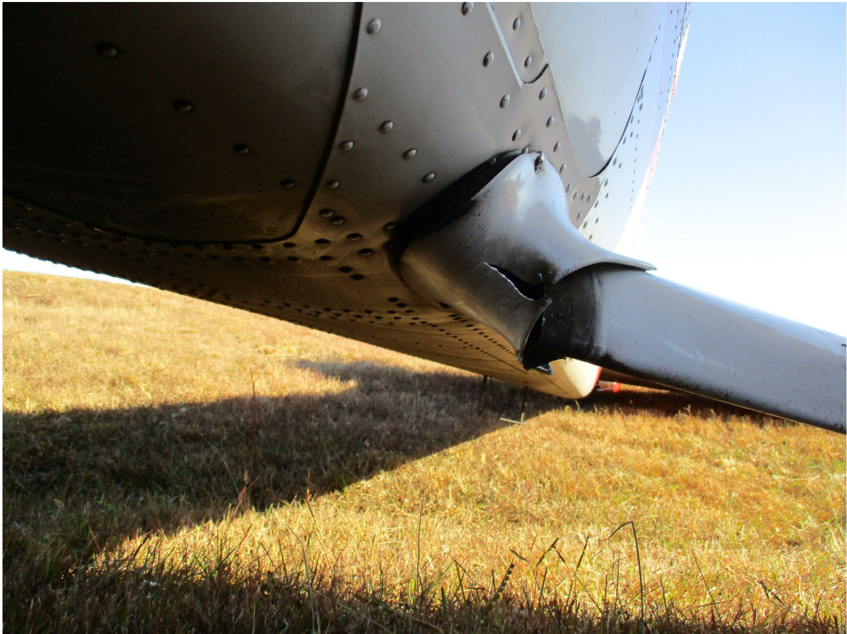
Photo 6 – Closeup View of Damage to Left Main Landing Gear (Courtesy of FAA)
