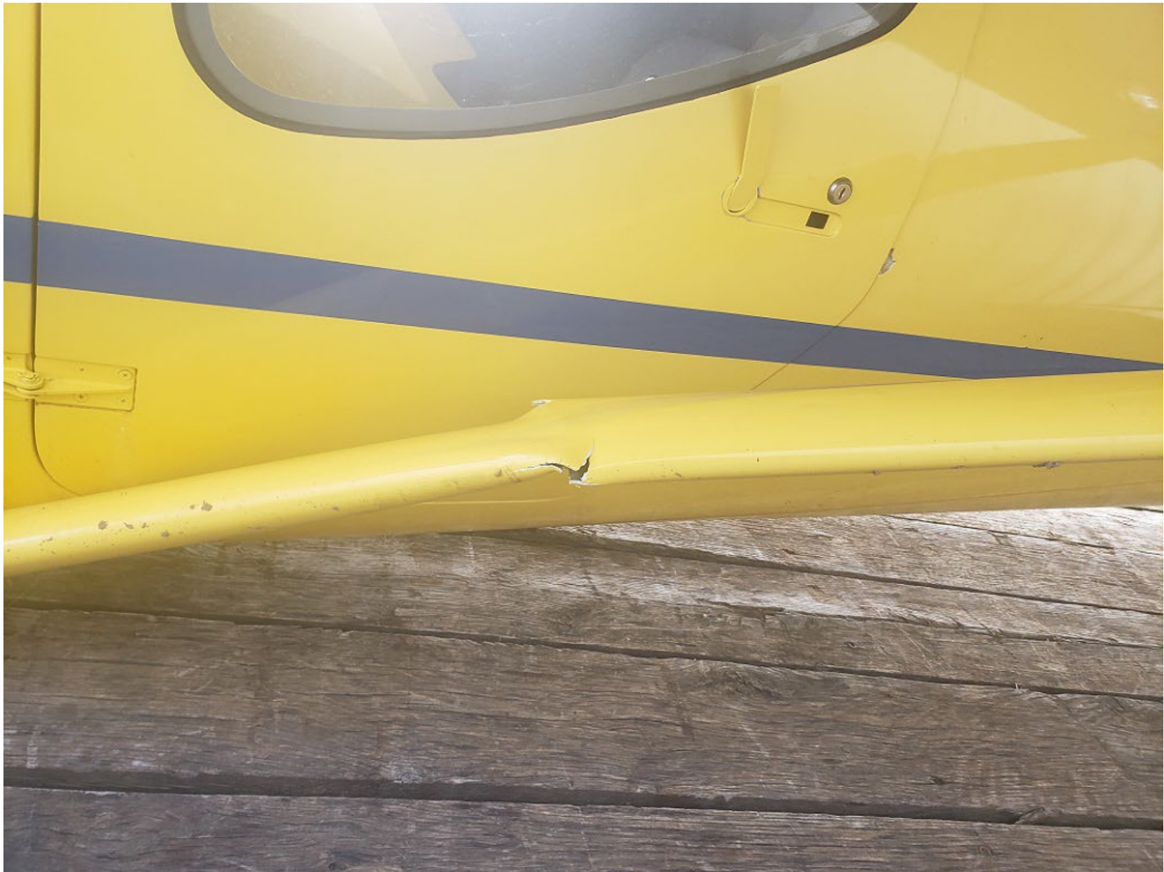
Photo 2 – Left Wing Strut Damage (photo courtesy of FAA)
