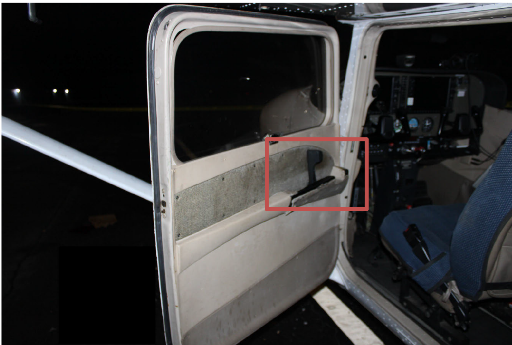
Photograph 5 - Close Up of Left Door Handle (Courtesy of Bulloch County Sheriff's Office)
