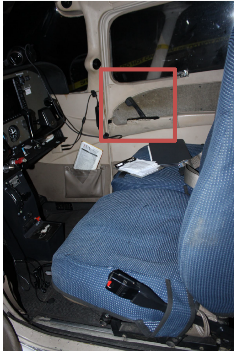
Photograph 6 - Close Up of Right Door Handle (Courtesy of Bulloch County Sheriff's Office)
