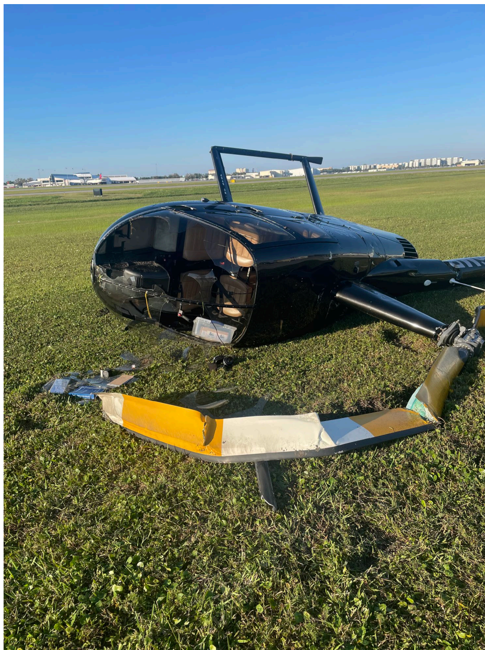
Photo 1 – View of helicopter resting on right side showing damage to main rotors and tail boom.
