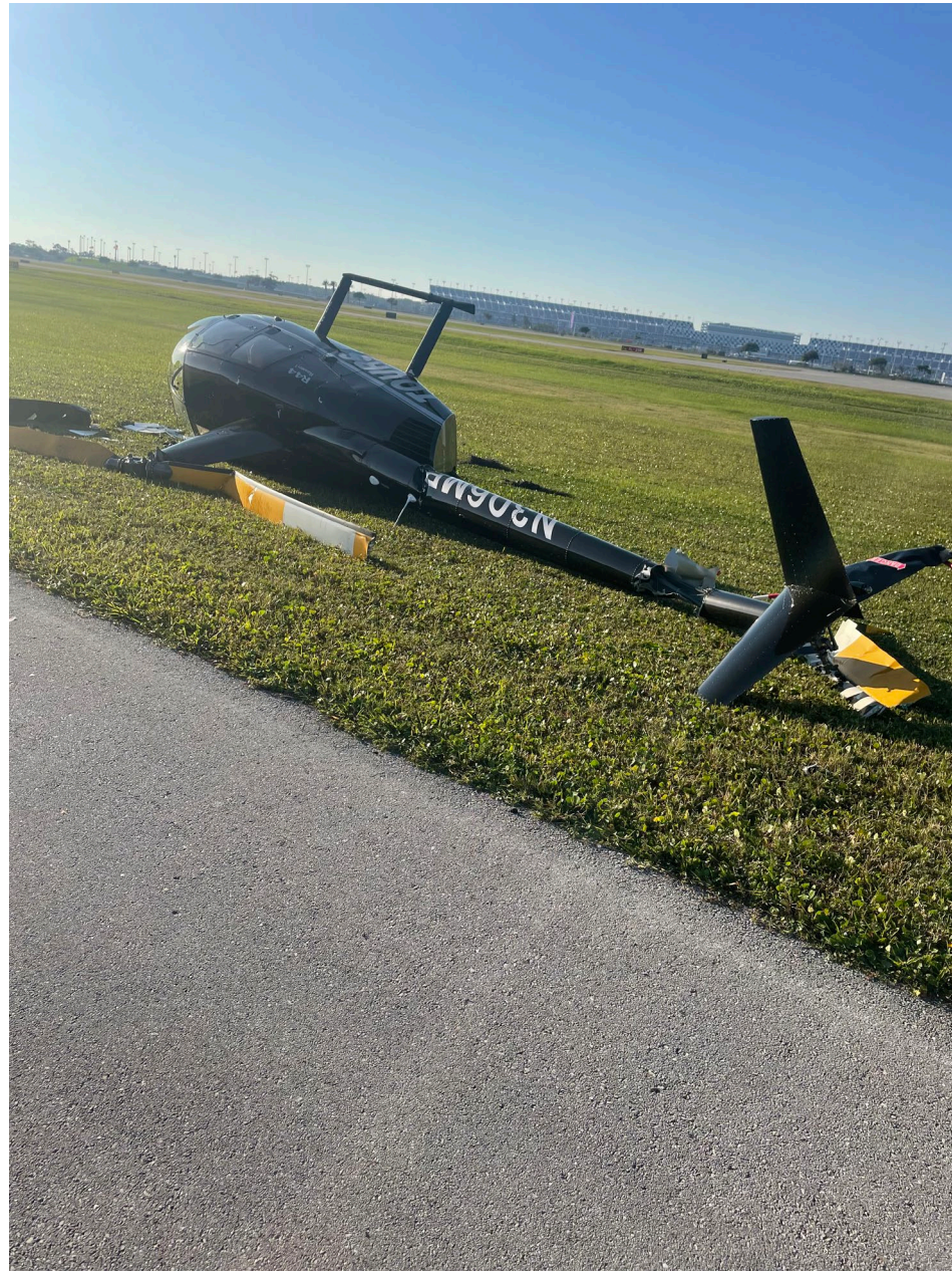
Photo 2 – View of aft of helicopter resting right side showing buckled tail boom.
