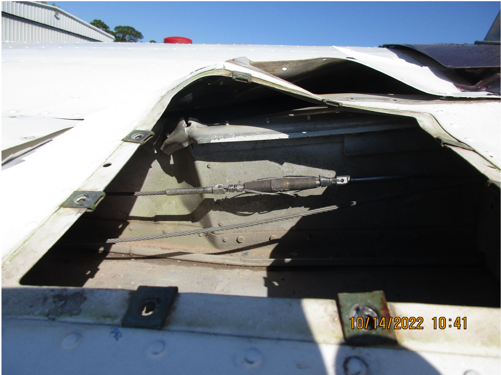
Photo 3 – FAA Digital Photograph. View Showing the Internal Structural Damage to the Left Wing.
