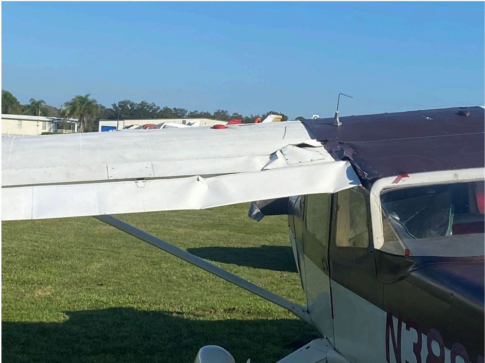
Photo 2 – FAA Digital Photograph. View Taken Behind Left Wing Near Wing Root Looking Forward. Note Structural Damage to the Left Wing.
