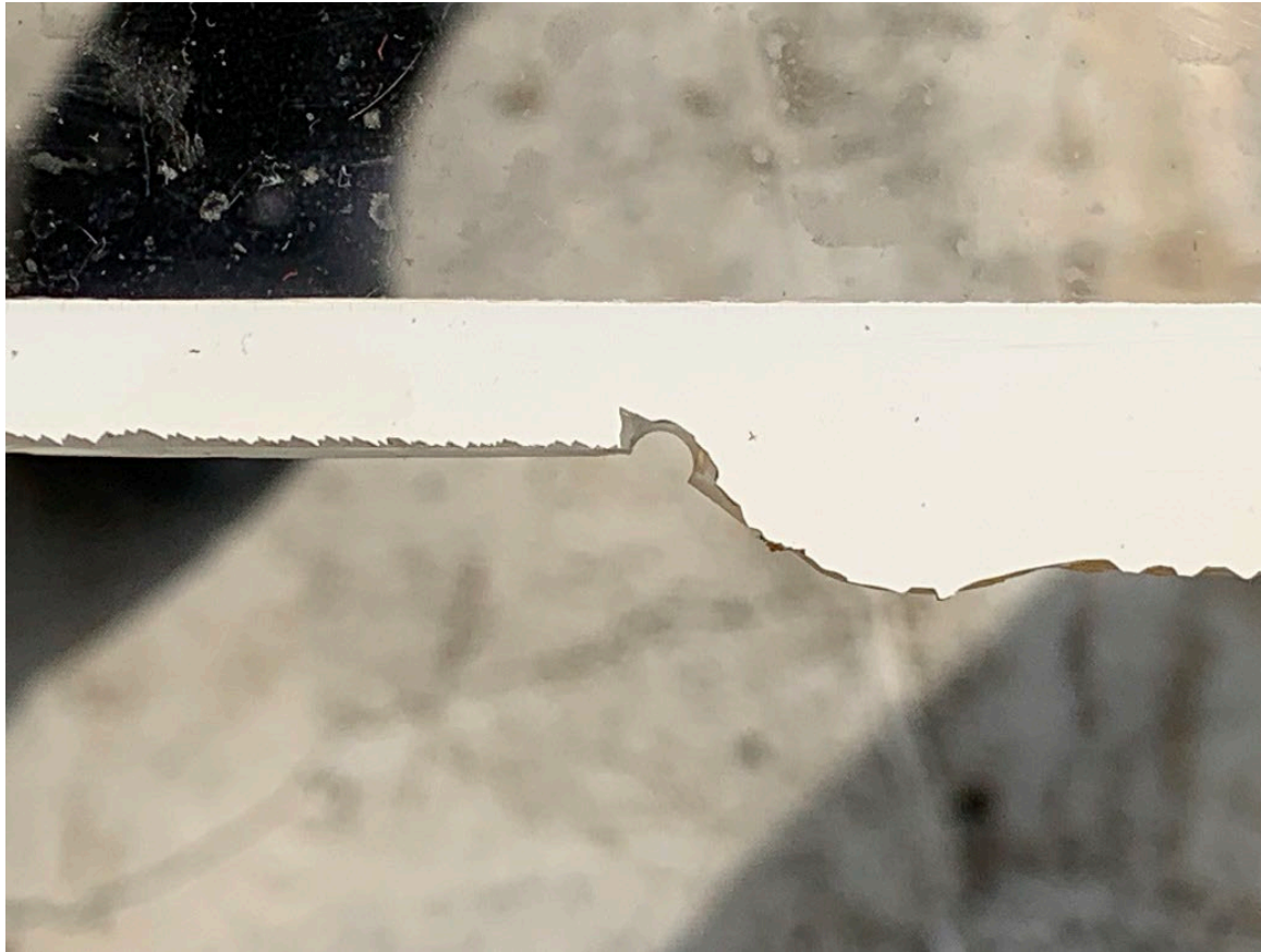
Photograph 4 - Stop Drill Hole (Courtesy of FAA)
