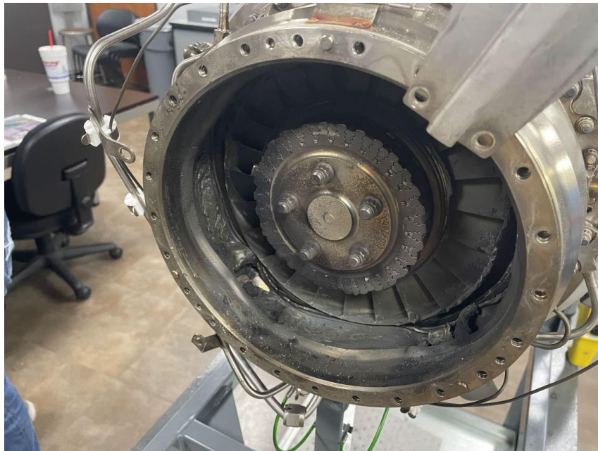
Photo 1: Free Turbine Blade Shedding (Overspeed Protection)
