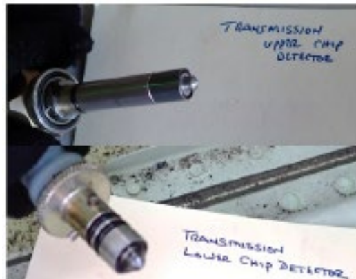
Photo 3: Transmission Chip Detectors (Courtesy Bell Helicopter Textron)
