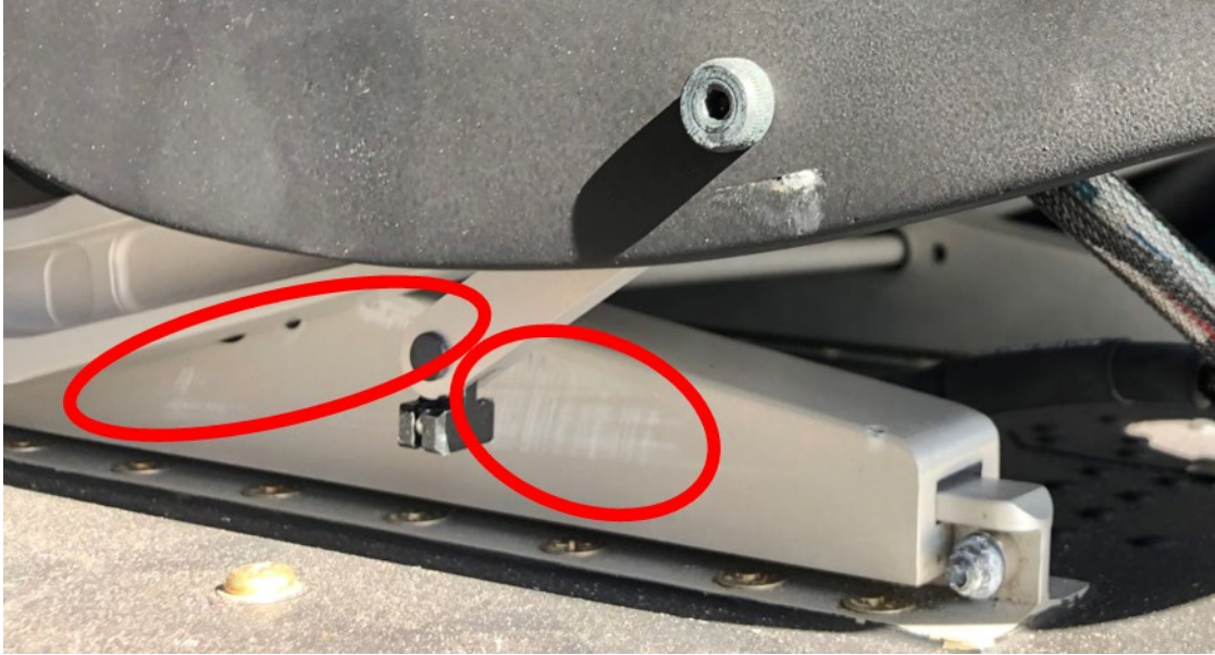
Figure 16. Fretting marks between the pilot right hand seat leg and EA device.
