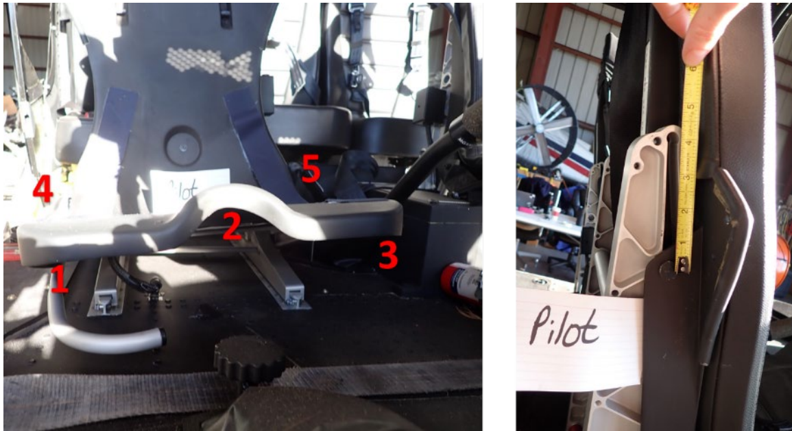
Figure 20. Five points measured on the seat bucket bottom and vertical displacement of seat bucket guide pins.
