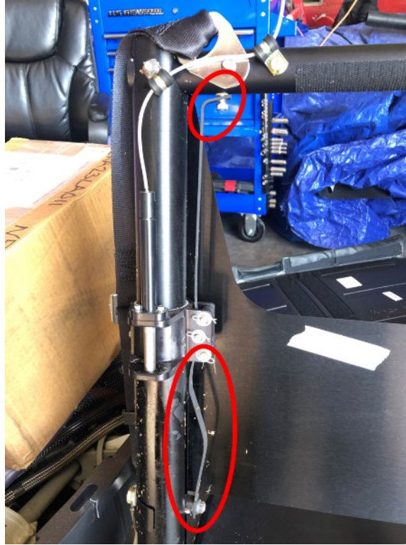
Figure 28. EA Device strip flange bending at the top and buckling below the rollers.
