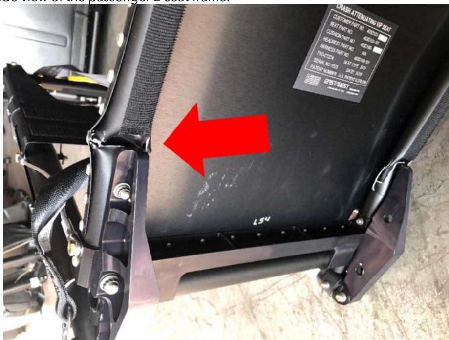
Figure 26. Bottom of passenger seat 2 showing tubular fractures forward of the reinforcing structure.
