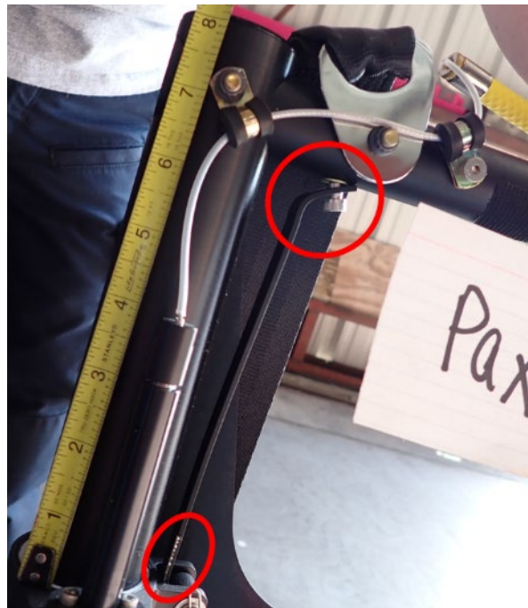
Figure 24. EA device strip showing flange bending at the top and fretting marks towards the bottom.
