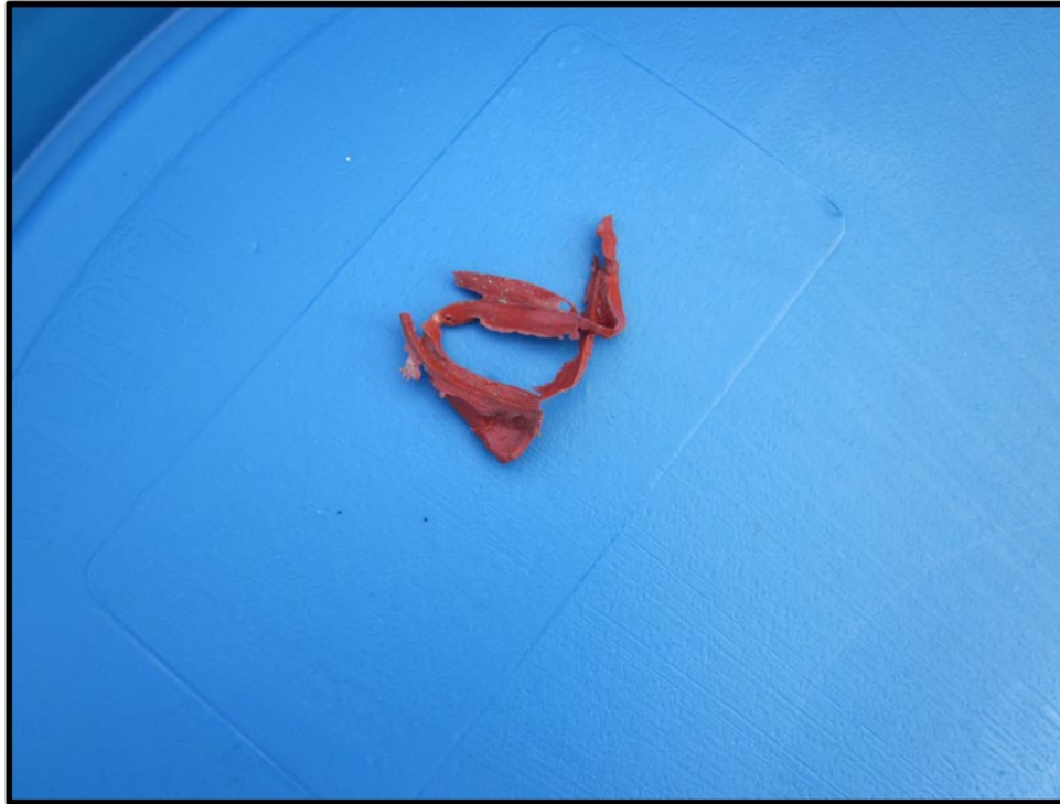
Figure 3: View of Foreign Object Removed From Header Fuel Tank.
