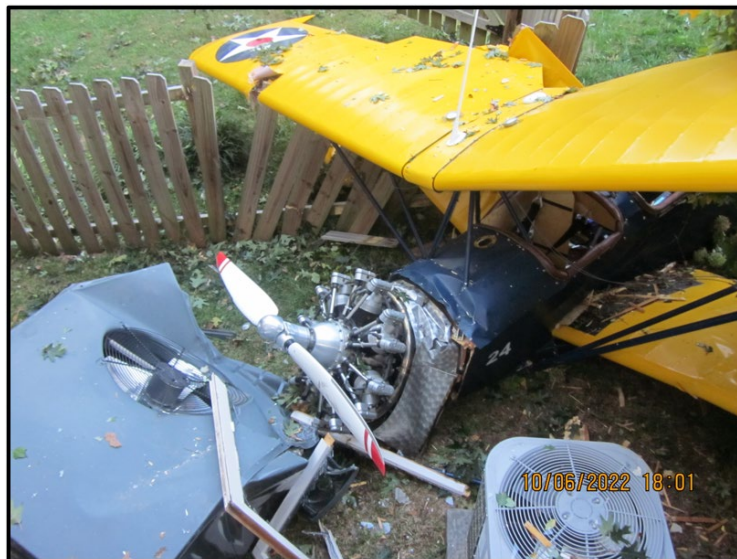
Figure 8: Displaced Engine with Attached Propeller.
