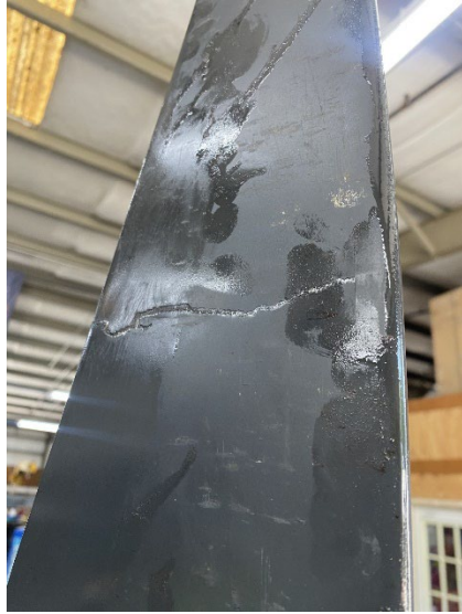
Figure 6: View of Chordwise Crack in One Propeller Blade.
