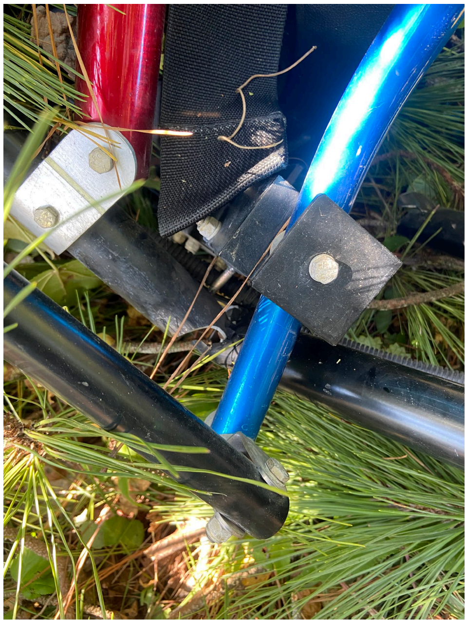
Photo 3 – Airframe tubing damage (FAA Photo)
