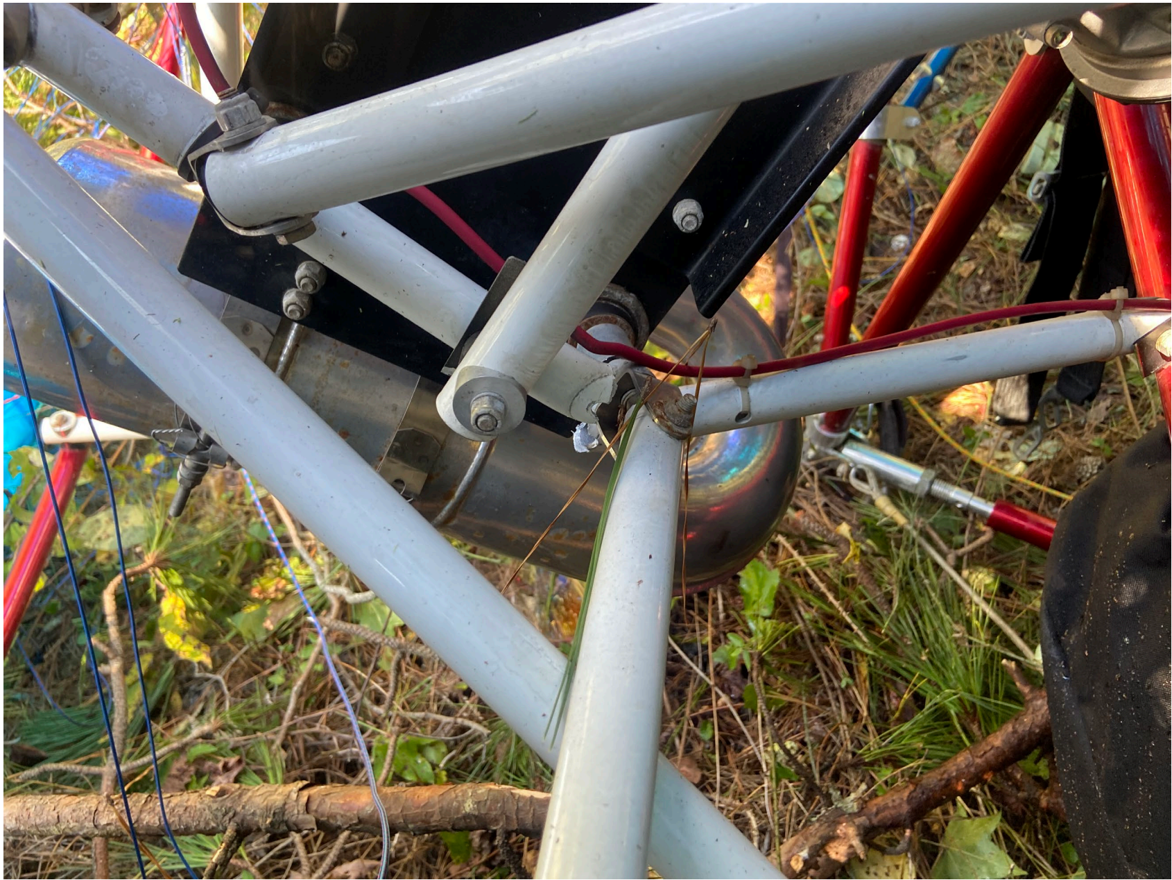
Photo 2 – Airframe tubing damage (FAA Photo)
