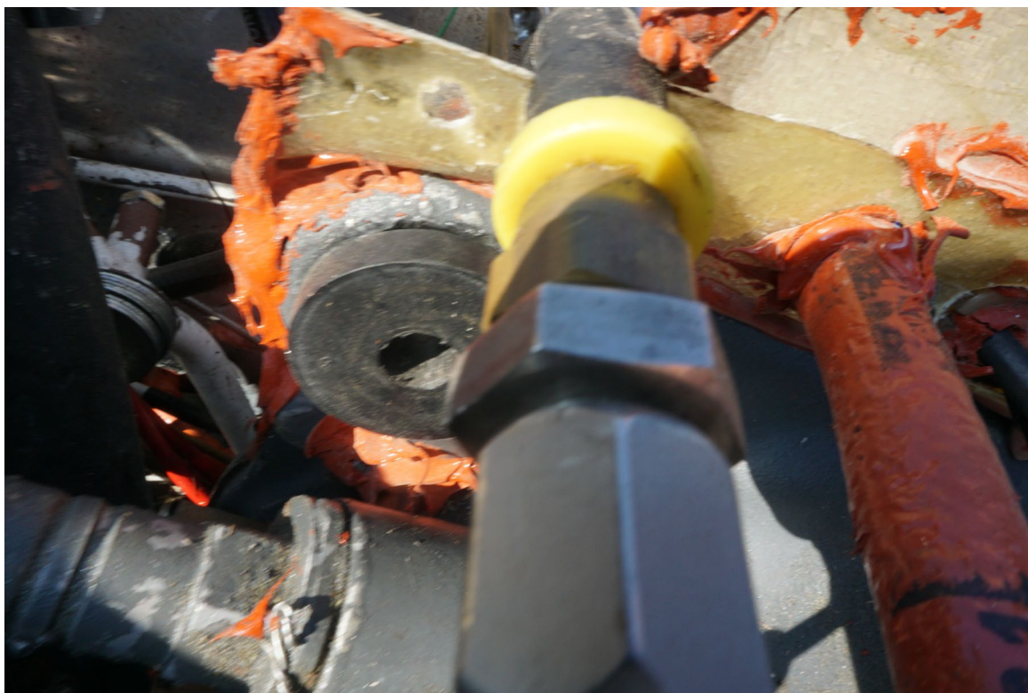
Photograph 5 -Left engine upper bushing (Courtesy of NTSB)
