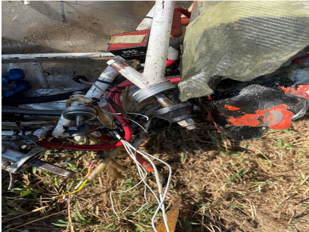
Photograph 4 - Engine mounts with non-standard washers (Courtesy of NTSB)
