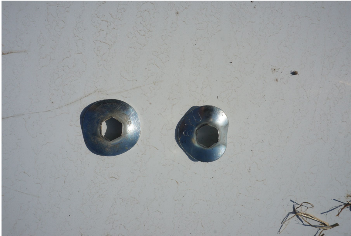
Photograph 7 - Nonstandard upper engine mount washers (Courtesy of NTSB)
