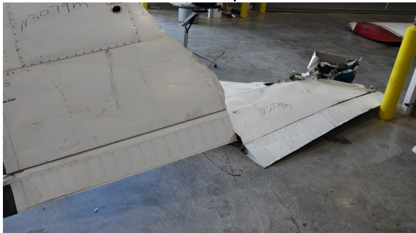
Photo 2 - View of outboard right wing (cut for recovery). (Photo courtesy of Piper Aircraft)
