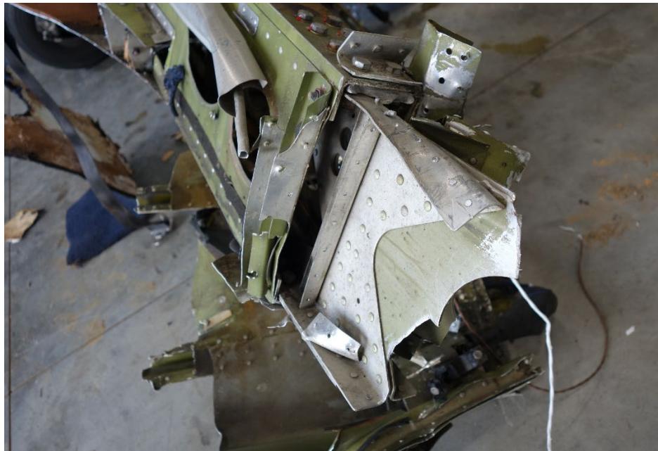
Photo 5 - View of fractured main wing spar. (Photo courtesy of Piper Aircraft)
