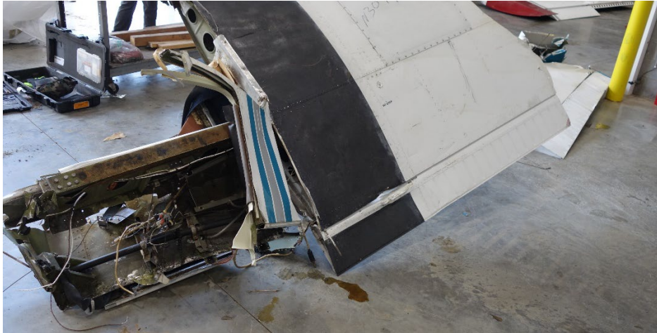
Photo 1 - View of inboard right wing (cut for recovery) and main spar. (Photo courtesy of Piper Aircraft)
