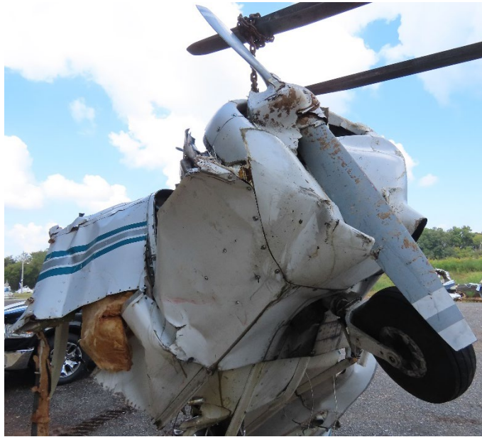
Photo 14 - View of hoisted engine and propeller before examination. (Photo courtesy of Lycoming Engines)
