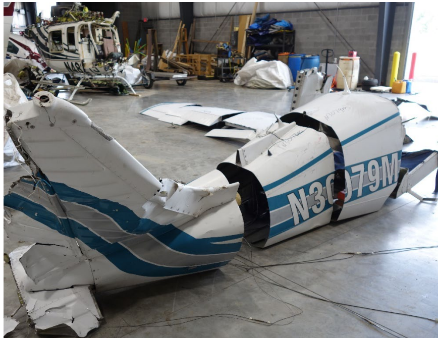
Photo 7 - View of empennage and aft fuselage (cut for recovery). (Photo courtesy of Piper Aircraft)
