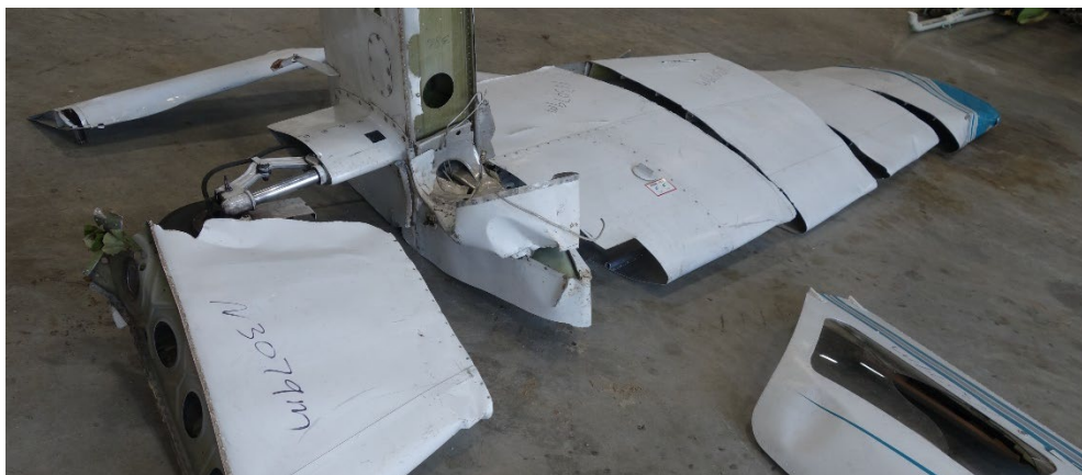
Photo 3 - View of left wing and cockpit door (cut for recovery). (Photo courtesy of Piper Aircraft)
