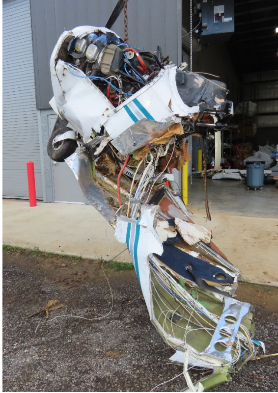
Photo 12 - View of hoisted engine section with forward cockpit and lower fuselage. (Photo courtesy of Lycoming Engines)
