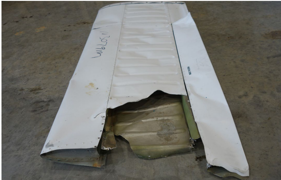
Photo 9 - View of right side of fractured stabilator. (Photo courtesy of Piper Aircraft)
