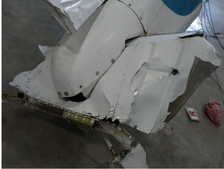
Photo 8 - View of fractured stabilator on tail cone. (Photo courtesy of Piper Aircraft)
