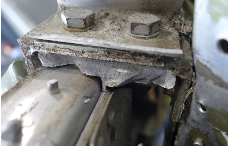
Photo 6 - Close-up view of fractured wing spar. (Photo courtesy of Piper Aircraft)
