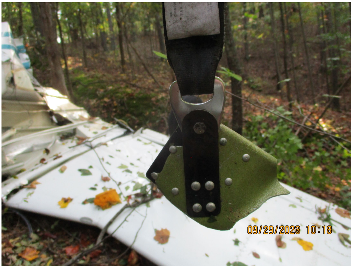
Photograph 4 - Seatbelt attachment point where torn from fuselage
