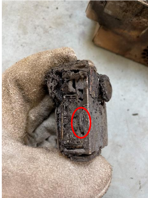
Figure 2. Device's internal memory unit (red box).
