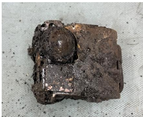
Figure 1. The GoPro Hero (Device 1), as received from the wreckage site. No data was recovered from the device.
