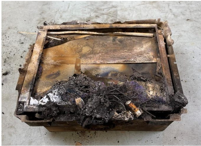
Figure 8. The Avidyne MFD, as received from the wreckage site.
