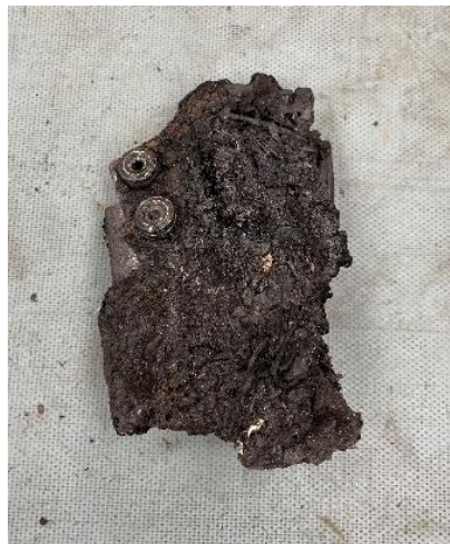
Figure 5. The Android phone, as received from the wreckage site.
