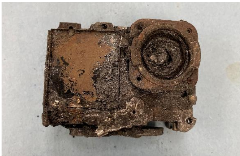
Figure 3. The GoPro Hero (Device 2), as received from the wreckage site.
