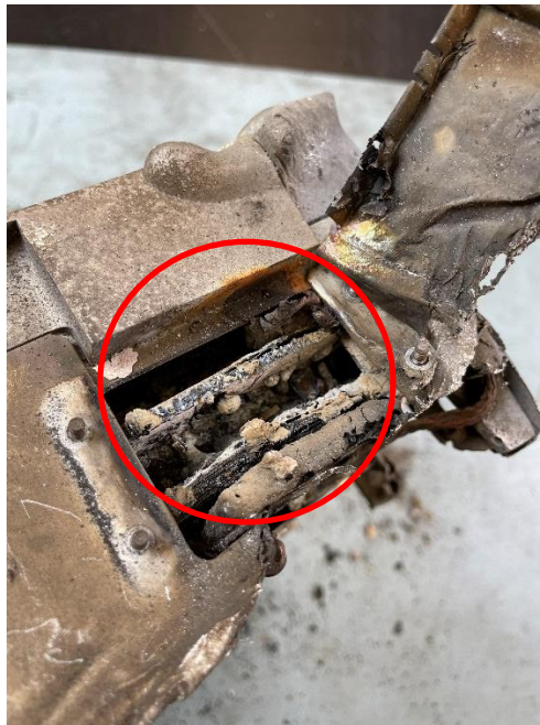
Figure 9. The Avidyne MFD CF card location. The CF card is circled in red. The CF card was destroyed.
