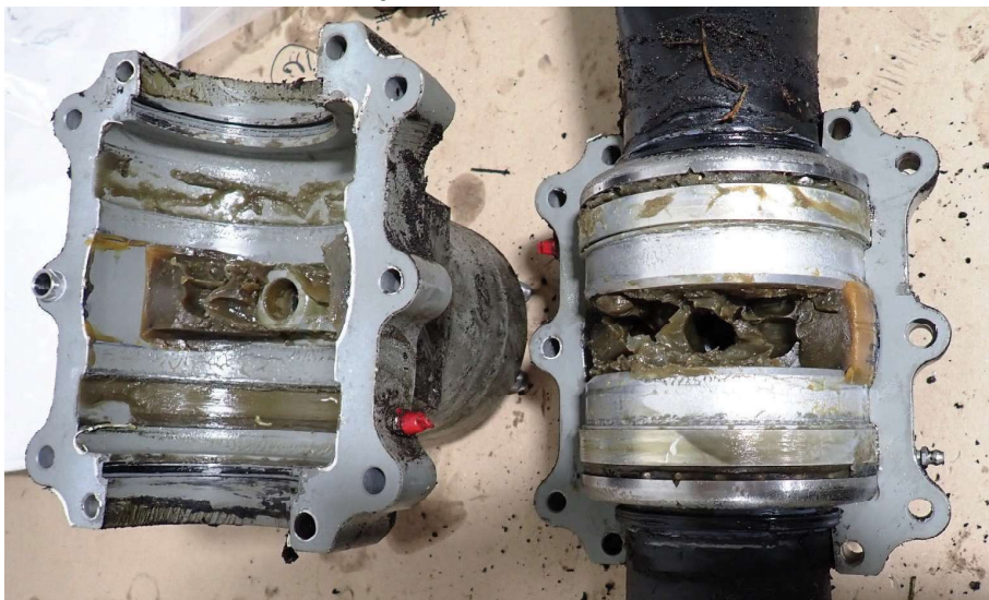
Photo #6 - Hub internal condition
