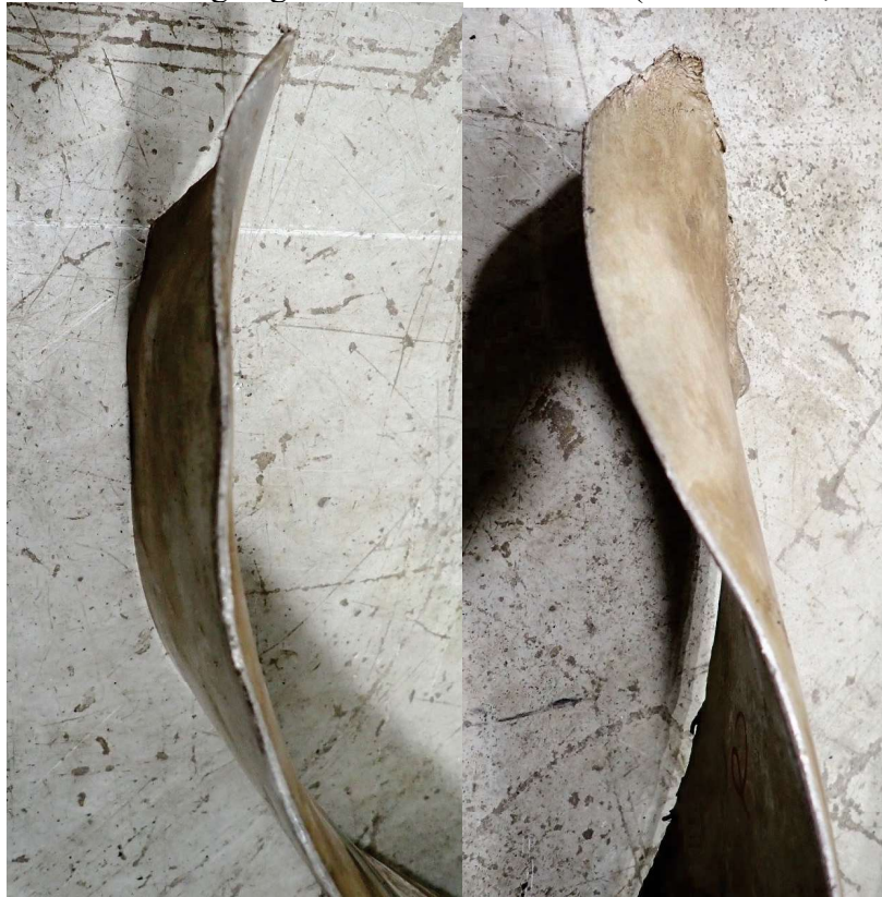
Photo #12 – Leading edge wave/tree strike bends (Blade #1 left, #2 right)
