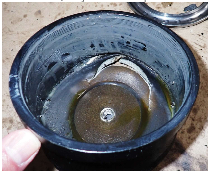
Photo #3 – Cylinder crushed/punctured
