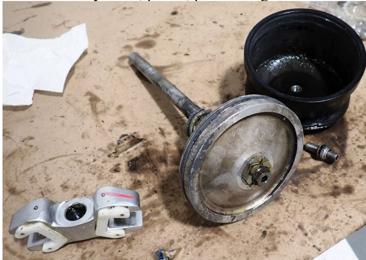
Photo #4 - Cylinder, piston, pitch change rod and fork
