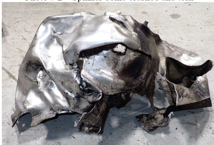
Photo # 2 – Spinner dome crushed and torn
