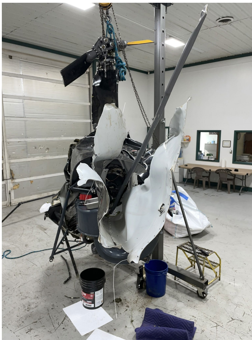
Photograph 6 - View looking forward of severed tail boom and control rod. (NTSB IIC)
