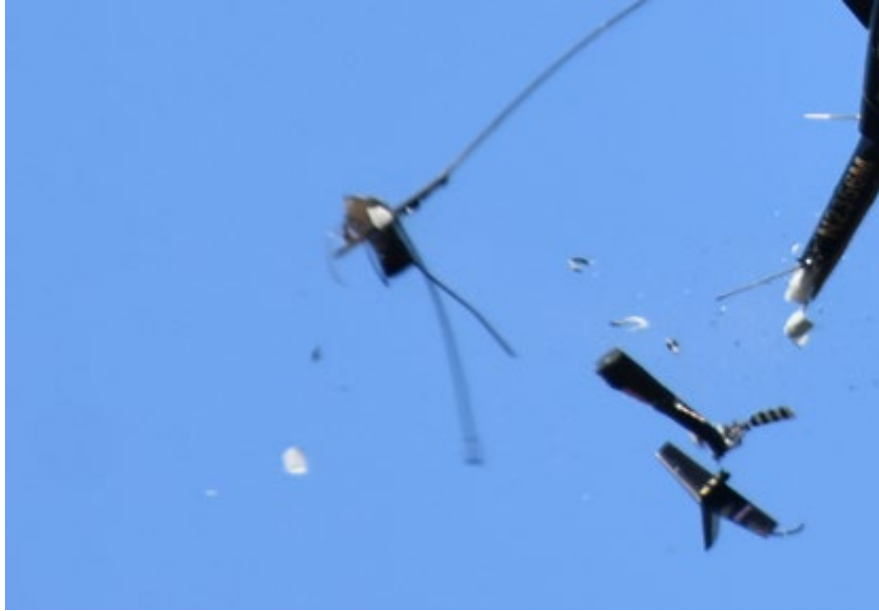
Figure 3 Tail boom severing showing 3 large pieces including the rotor blades and shaft.
