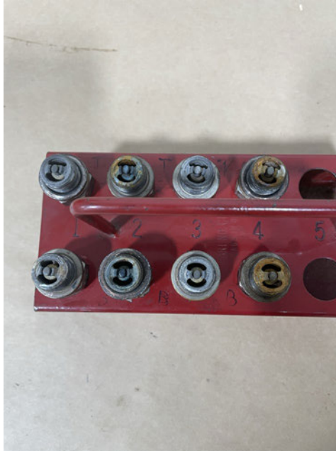
Figure 4 Spark Plugs and blue tint
