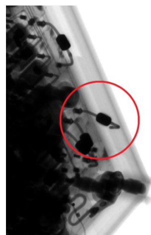
Figure 1 : Partially unsoldered components on ECU_1
