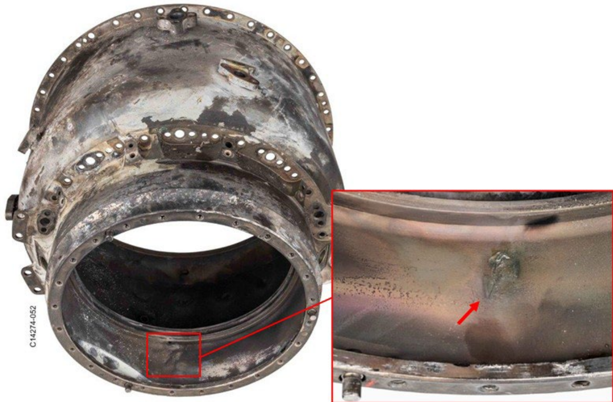
Figure 82. Turbine Case (L), Impact Mark at PT Containment Ring (R) (Figure Courtesy of SafranHE)
