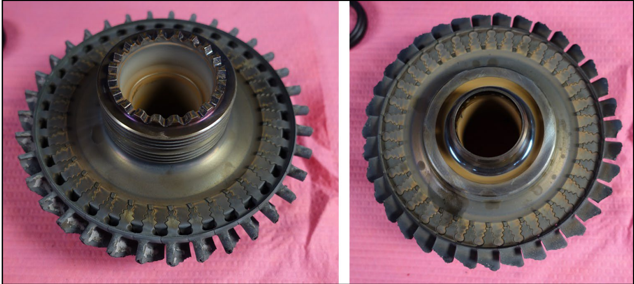
Figure 23. Gas Generator Turbine, Forward Side (L), Aft Side (R)
