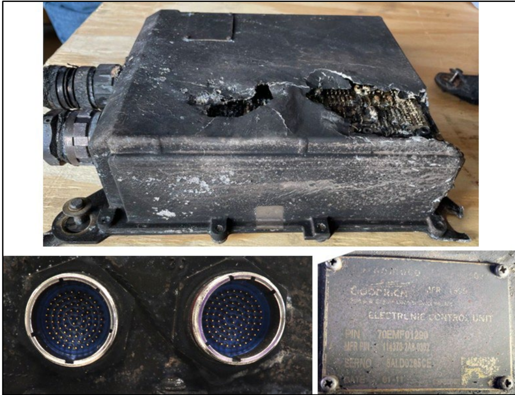
Figure 8. No. 2 Engine EECU - Removed
