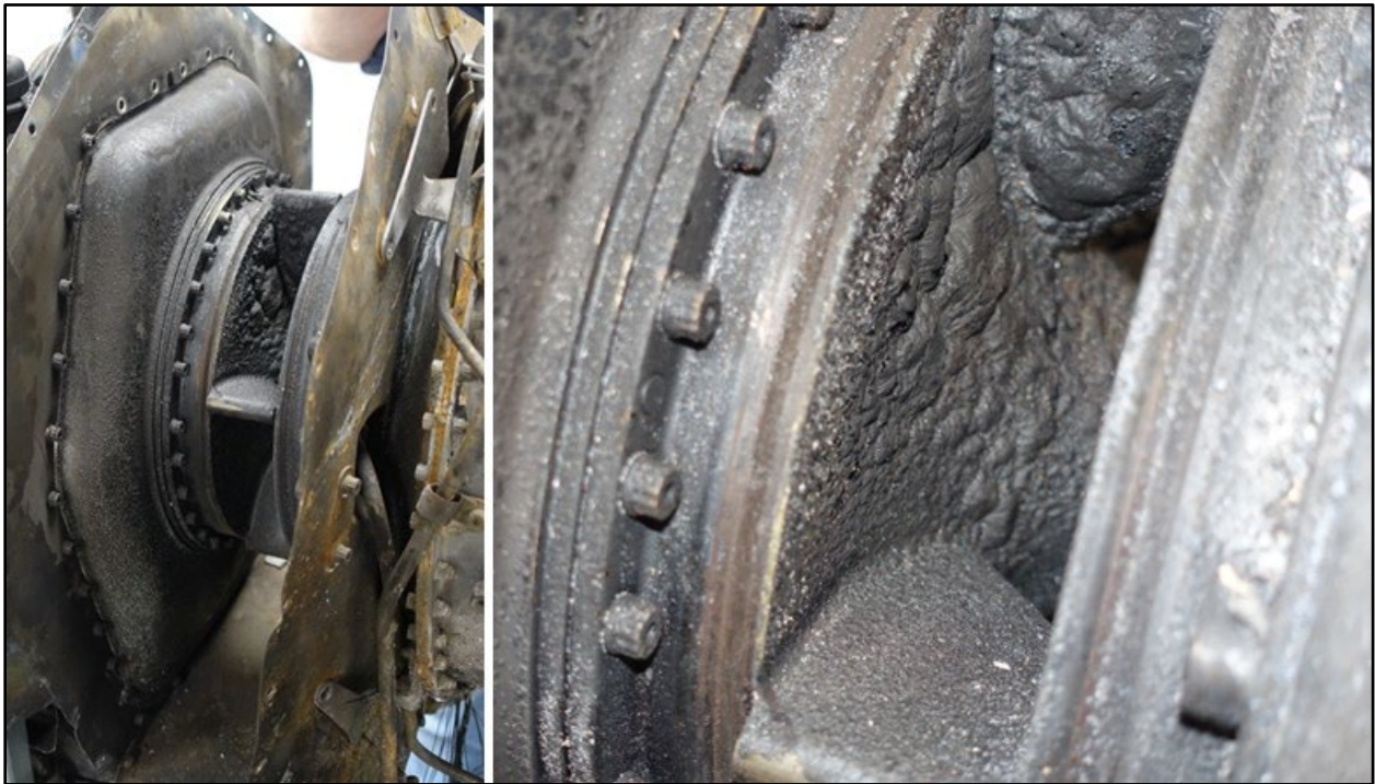
Figure 12. Engine Inlet Residue
