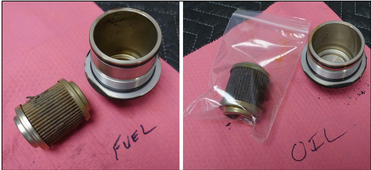
Figure 15. Fuel and Oil Filters **Fuel Filter Damage During Examination
