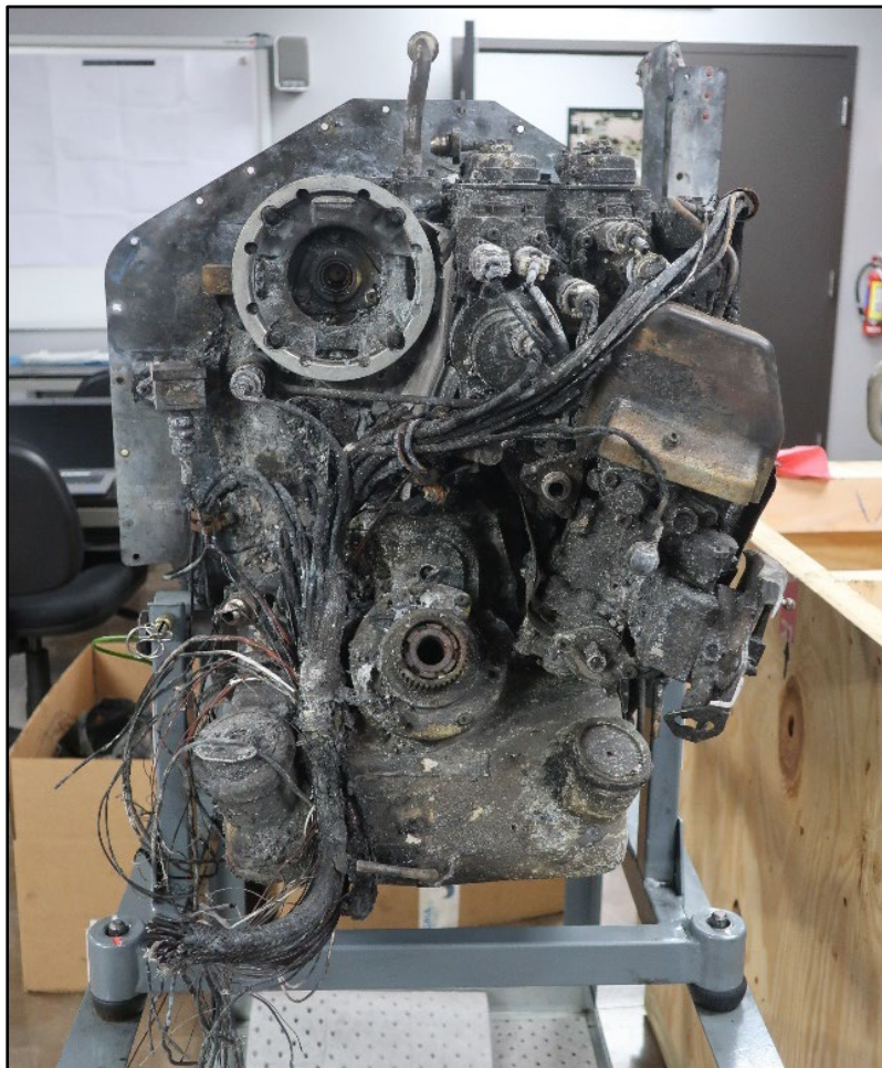
Figure 36. ESN 30182 As Received - Front/Gearbox Side
