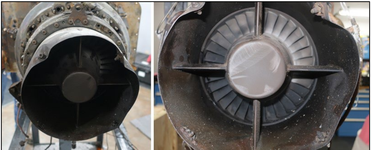
Figure 39. Exhaust Pipe Deformations (L), PT Blades (R)
