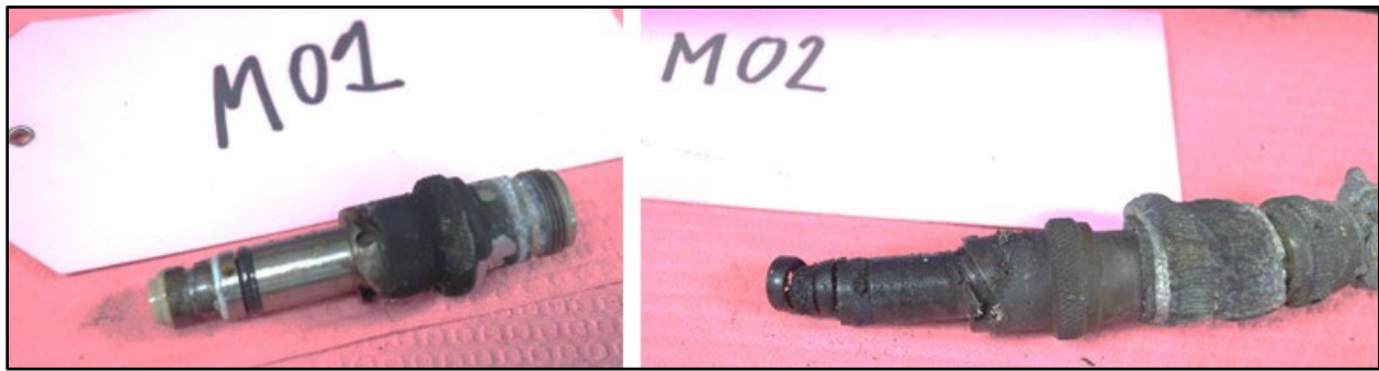
Figure 42. MCDs - (M01) Reduction Gearbox (L), (M02) Rear Bearing (R)
