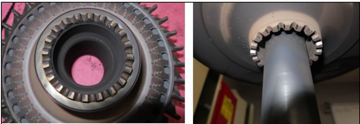
Figure 44. Gas Generator Turbine Disk Curvic Coupling (L), Impeller Curvic Coupling (R)
