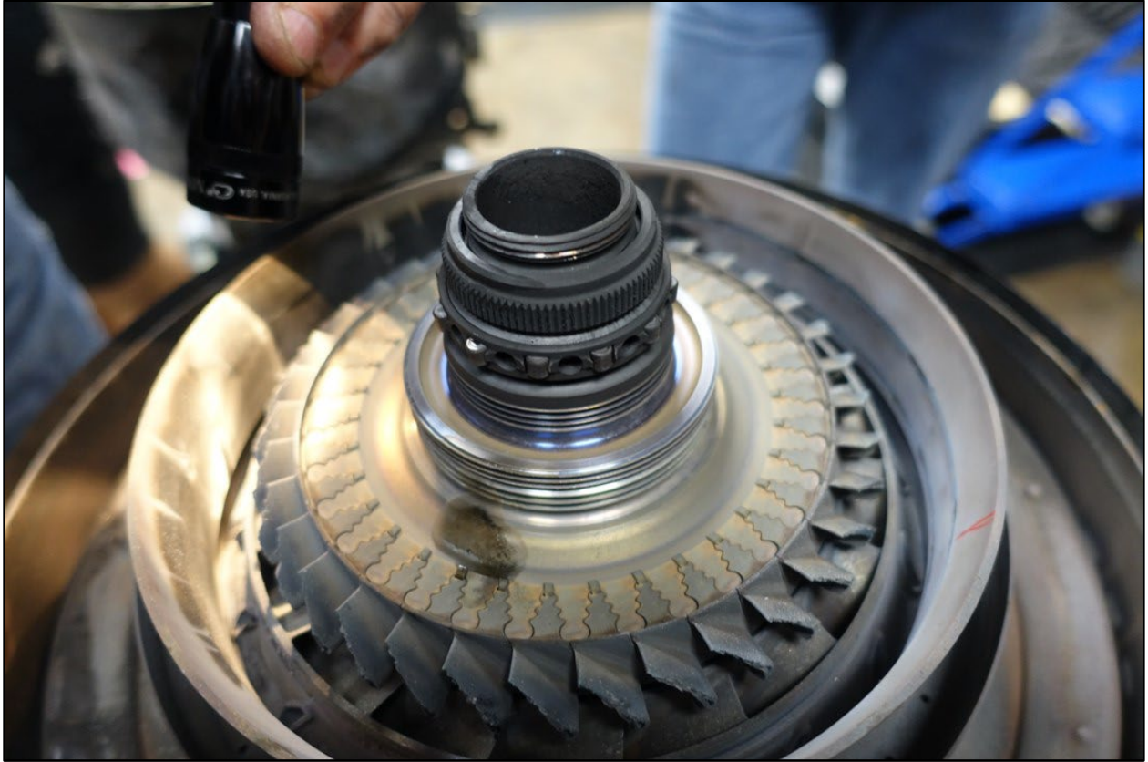
Figure 25. Gas Generator Turbine Rear Bearing
