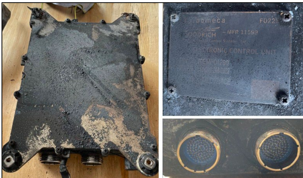
Figure 7. No. 1 Engine EECU - Removed
