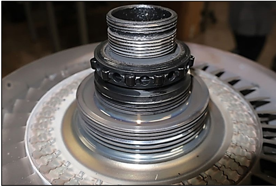
Figure 49. Gas Generator Turbine Rear Bearing
