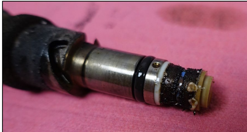
Figure 16. AGB Magnetic Chip Detector Plug Debris
