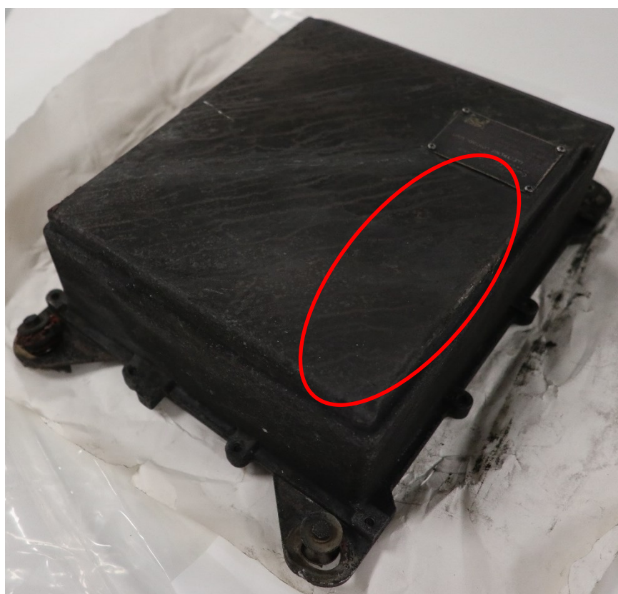
Figure 14 : ECU Highest thermal exposure area deduced from board 5 damages
