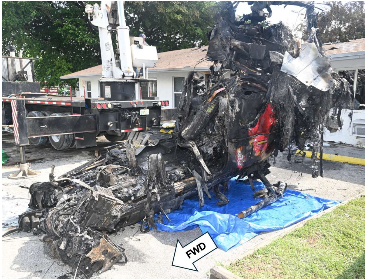
Figure 8. The main fuselage wreckage after removal from the building. (Image courtesy of BSO)
