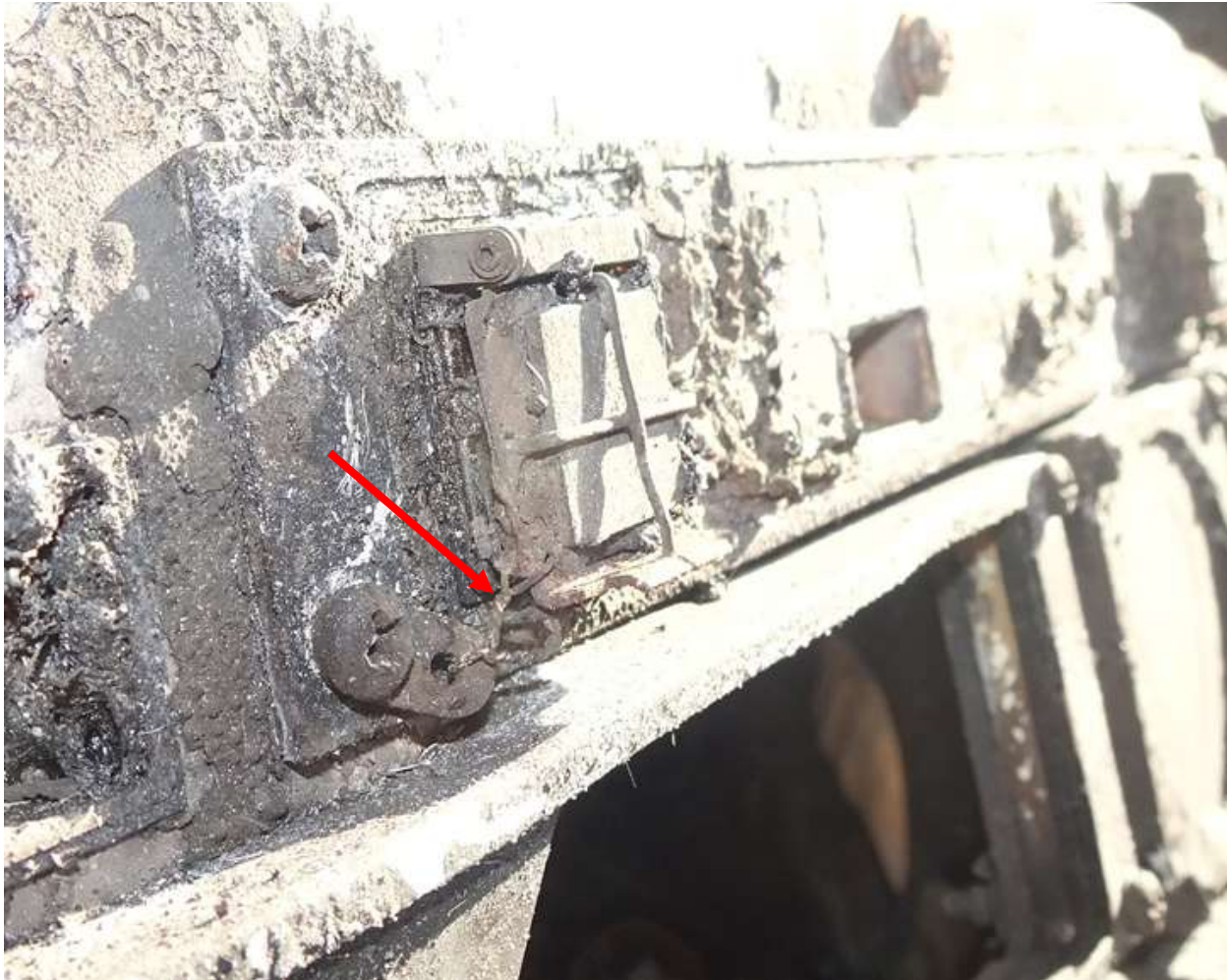
Figure 24. The No. 1 engine fire button showing the breakable wire (red arrow) and the safety guard over the button.
