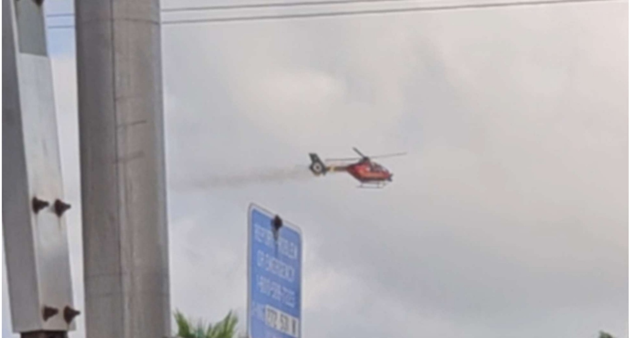
Figure 32. Visible smoke emanating from the accident helicopter. This still frame was captured about 10 seconds from the start of the ground witness video. (Video courtesy of BSO, still image captured by the NTSB)
