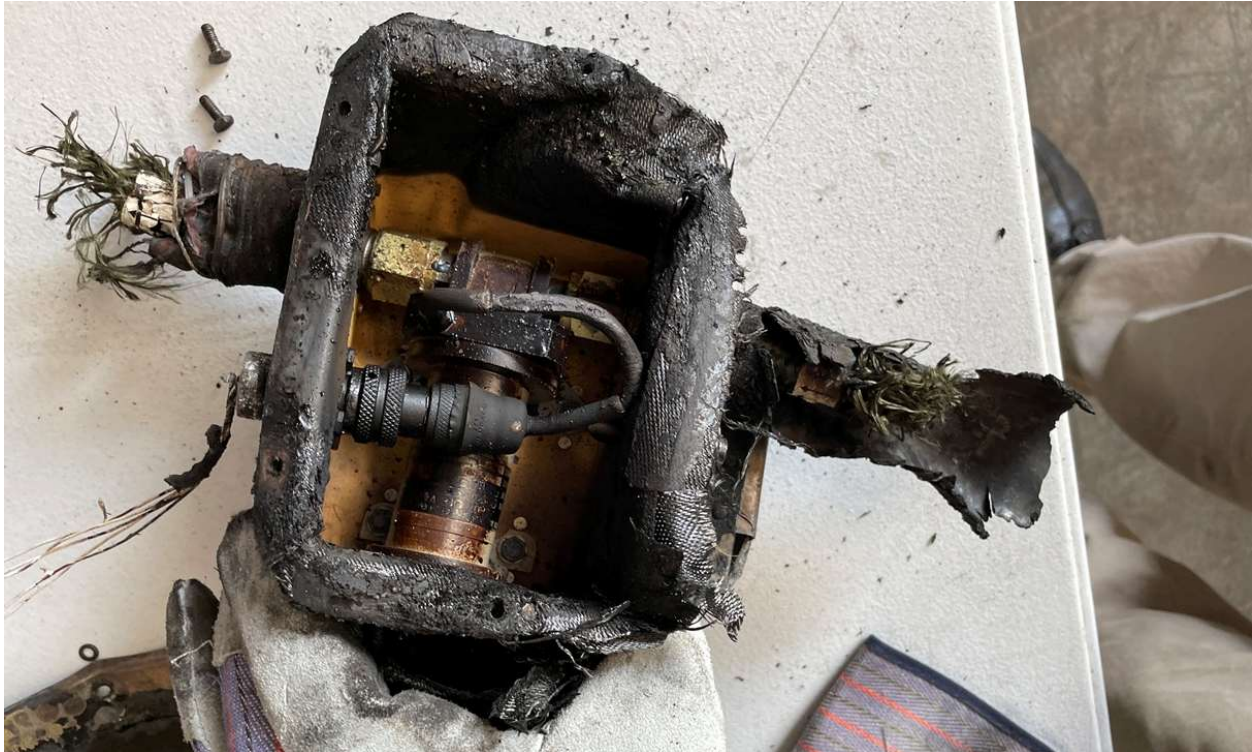
Figure 15. The emergency fuel shutoff valve for the No. 1 engine after removal from the main fuselage wreckage.
