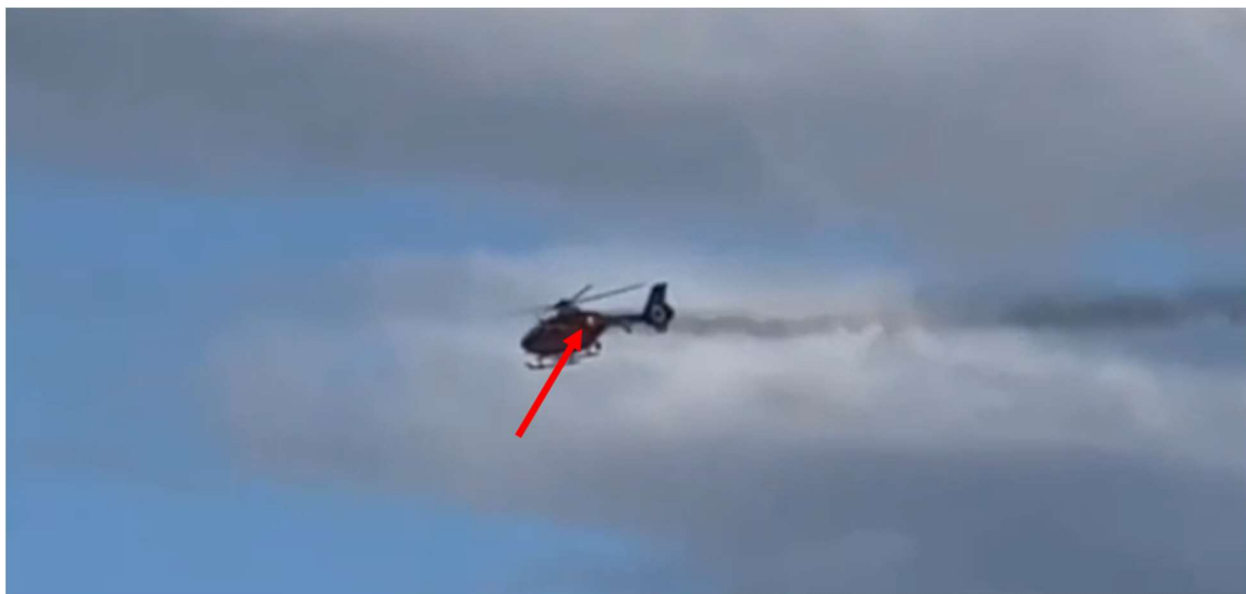
Figure 30. A still image from the start of the ground witness video that showed the accident helicopter with a smoke trail and visible flames (red arrow) emanating from the area of the No. 1 engine exhaust and the air conditioner condenser fans. (Video courtesy of BSO, still image captured and modified by the NTSB)
