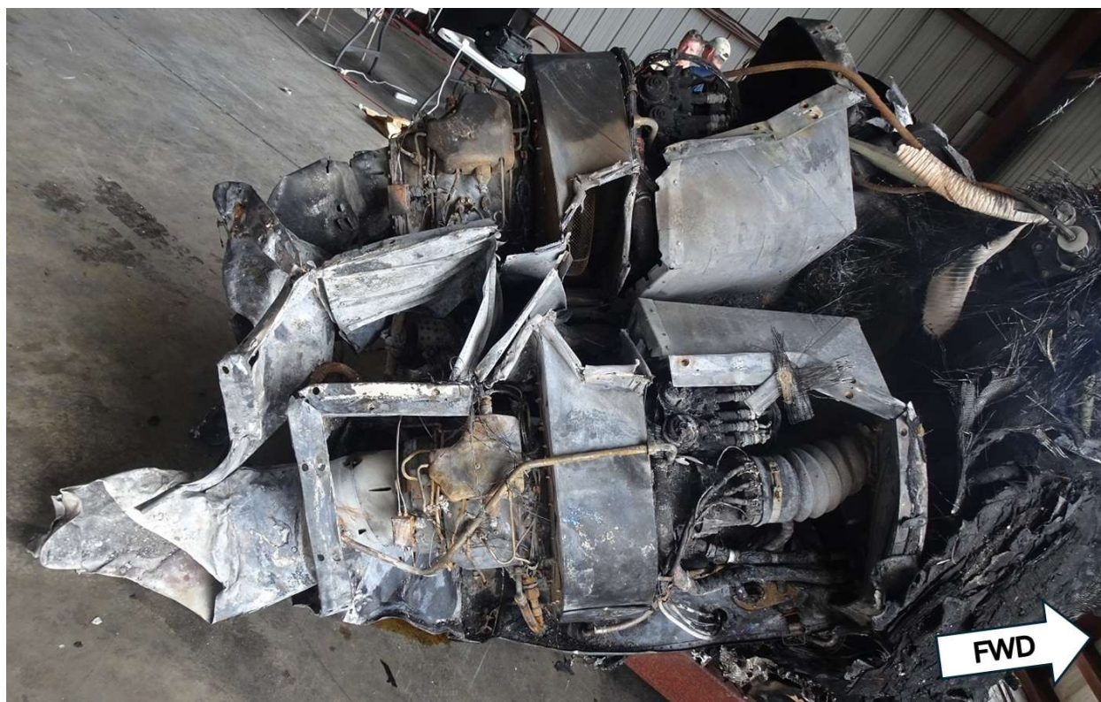
Figure 10. The Nos. 1 and 2 engine firewalls (top looking down).
