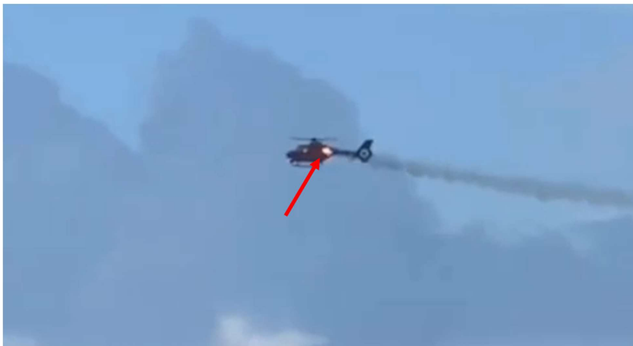
Figure 31. A still image taken about 35 seconds after the start of the 1-minute long ground witness video. The area of the visible flames (red arrow) appears larger than compared to the beginning of the video. (Video courtesy of BSO, still image captured and modified by the NTSB)
