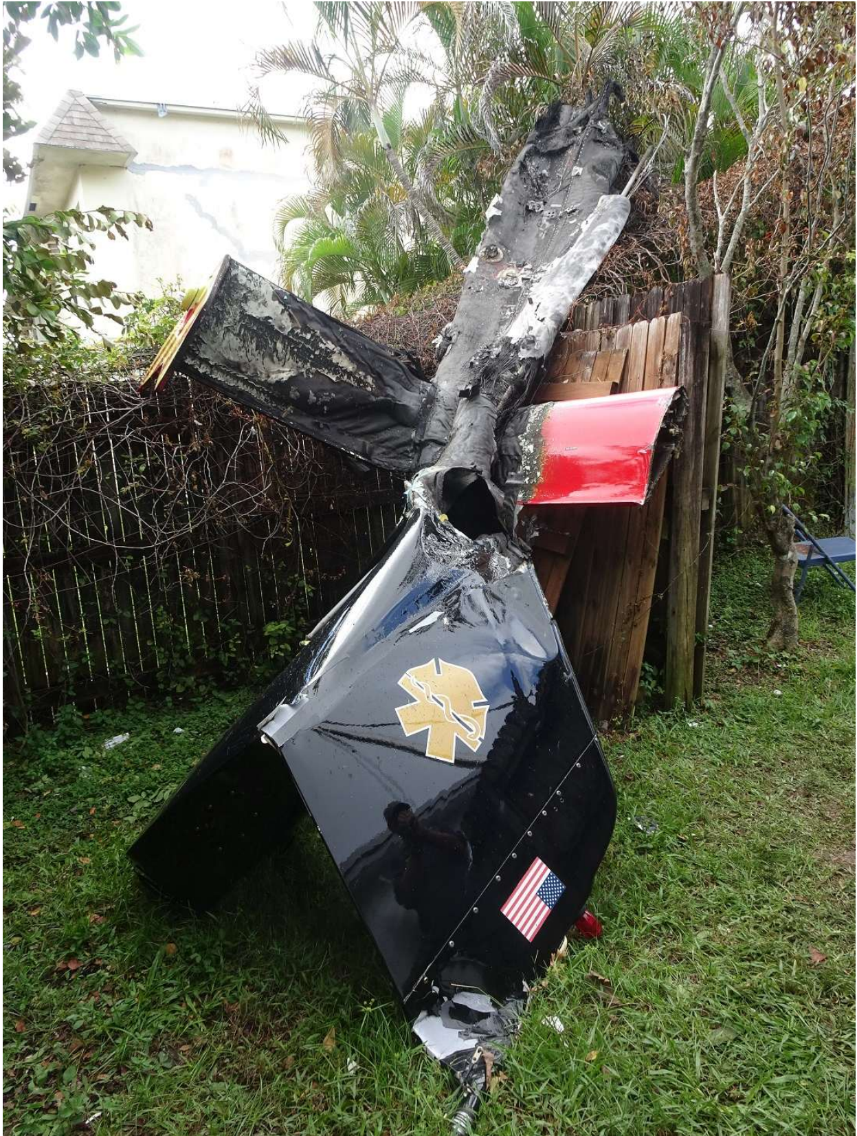
Figure 11. The tail boom, horizontal stabilizer, vertical fin, and fenestron wreckage.
