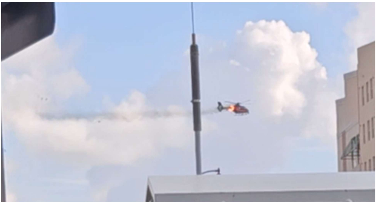
Figure 33. Visible flames emanating from the center tail boom area. This still frame was captured about 20 seconds from the start of the ground witness video, and about 5 seconds before partial separation of the tail boom. (Video courtesy of BSO, still image captured by the NTSB)
