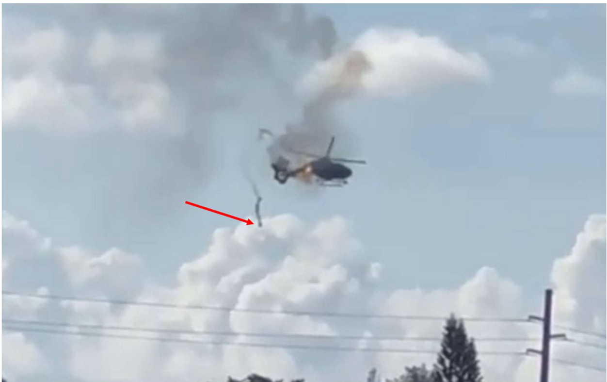
Figure 35. The visible smoke trail of the small object that separated from the helicopter.
