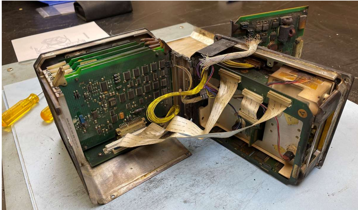
Figure 25. The accident CDS circuit cards upon opening its housing.
