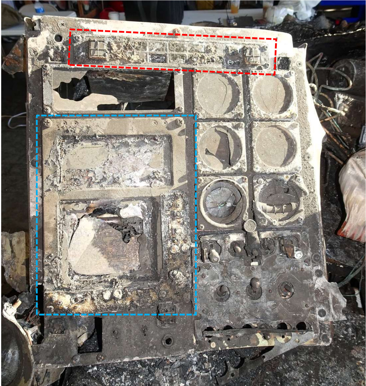
Figure 23. The instrument panel showing the CDS (blue outline) and warning unit (red outline).
