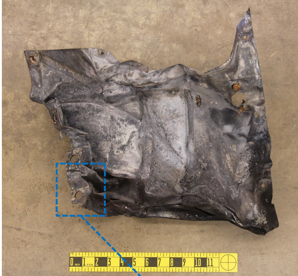
#1 Hot Section Firewall (Lower), Aft
