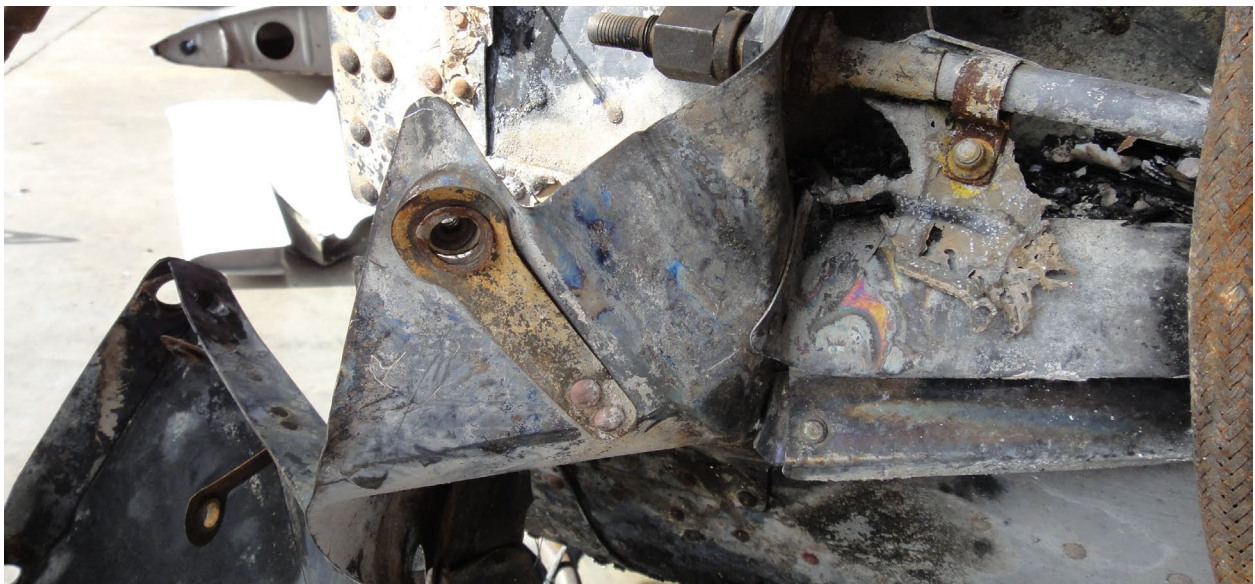
Figure 10. Photograph of thermal discoloration on driveshaft compartment seam.
