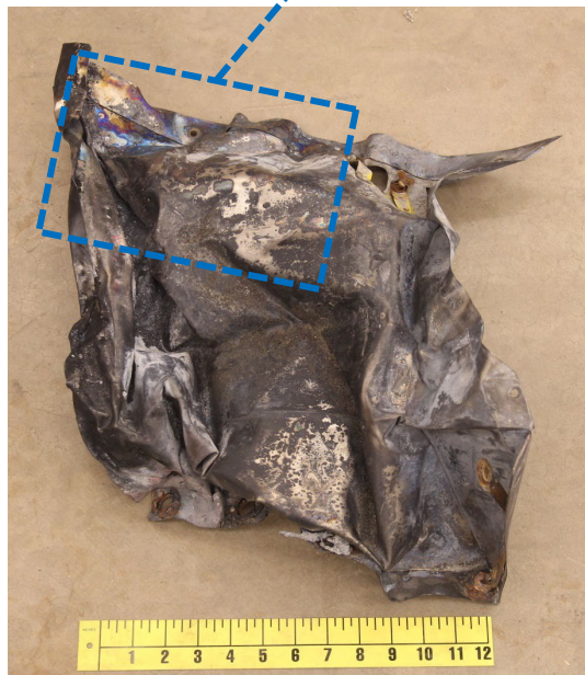
Figure 16. Photograph of thermal discoloration on #1 engine hot section firewall (lower), forward.
