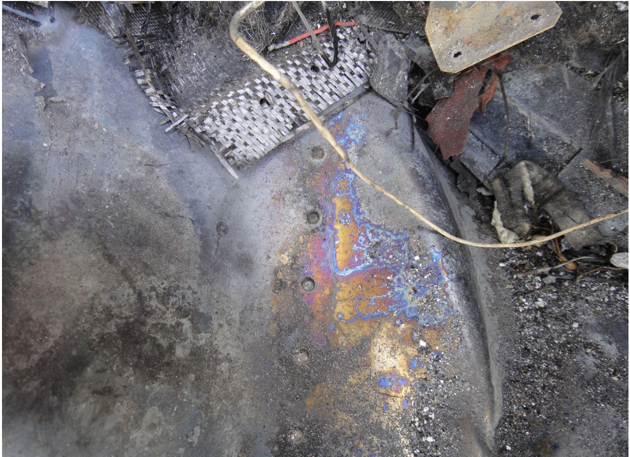
Figure 9. Photograph of thermal discoloration on #1 engine firewall.
