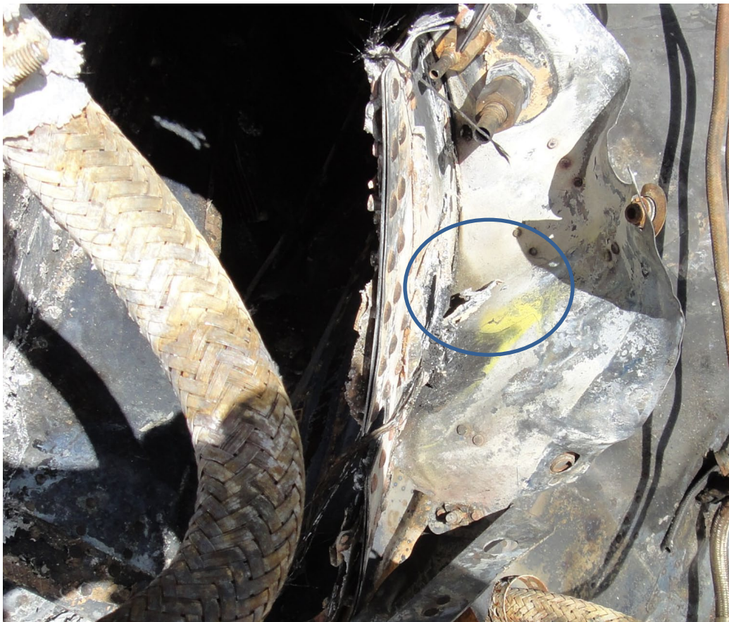
Figure 6. Photograph of yellow residue (circled) on #2 engine firewall.
