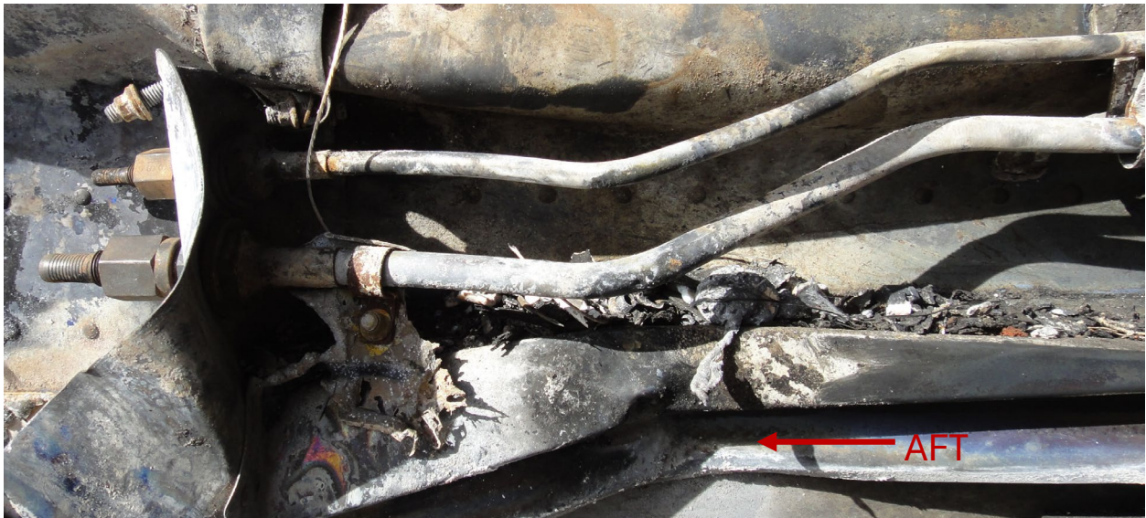
Figure 5. Photograph of white powdery residue on drive shaft.
