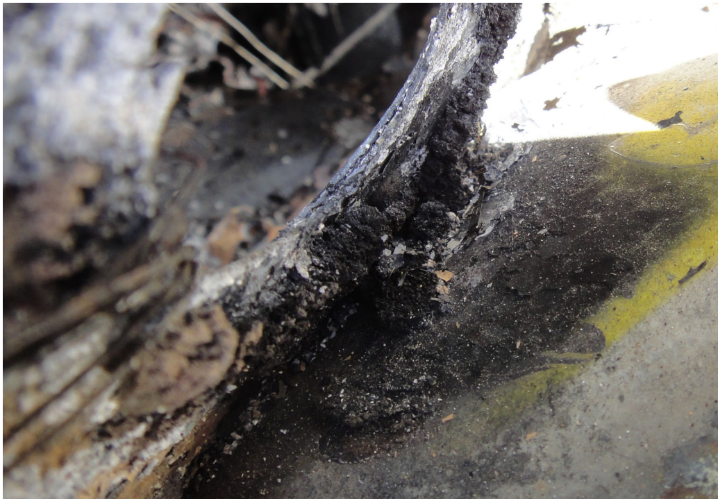
Figure 2. Photograph of area of oily residue was found on the lower firewall, inboard edge #2 engine.
