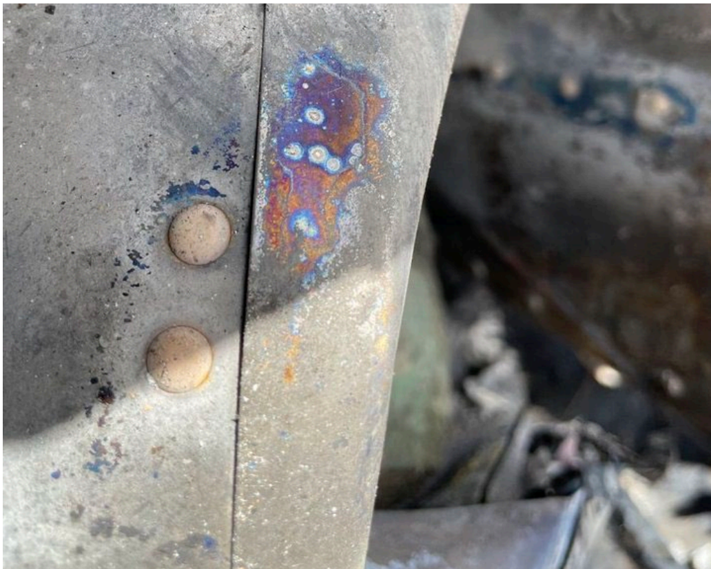
Figure 4. Photograph of blue and brass colored, splatter-shaped thermal patterns on #2 engine firewall.
