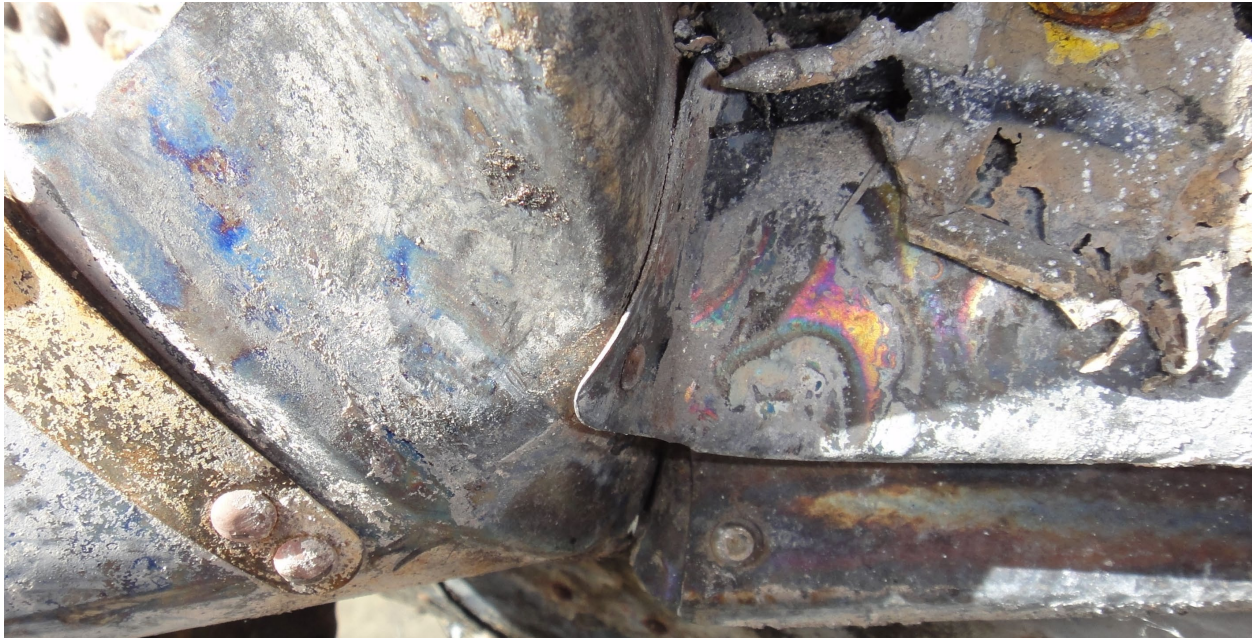
Figure 3. Photograph of discoloration on aft inboard corner of #2 engine compartment.
