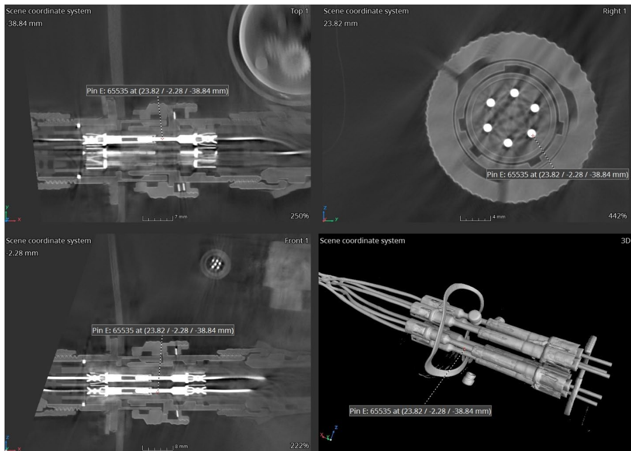
Figure 17. Fuel shut-off valve - electrical connector - pin E. (225 kV)
