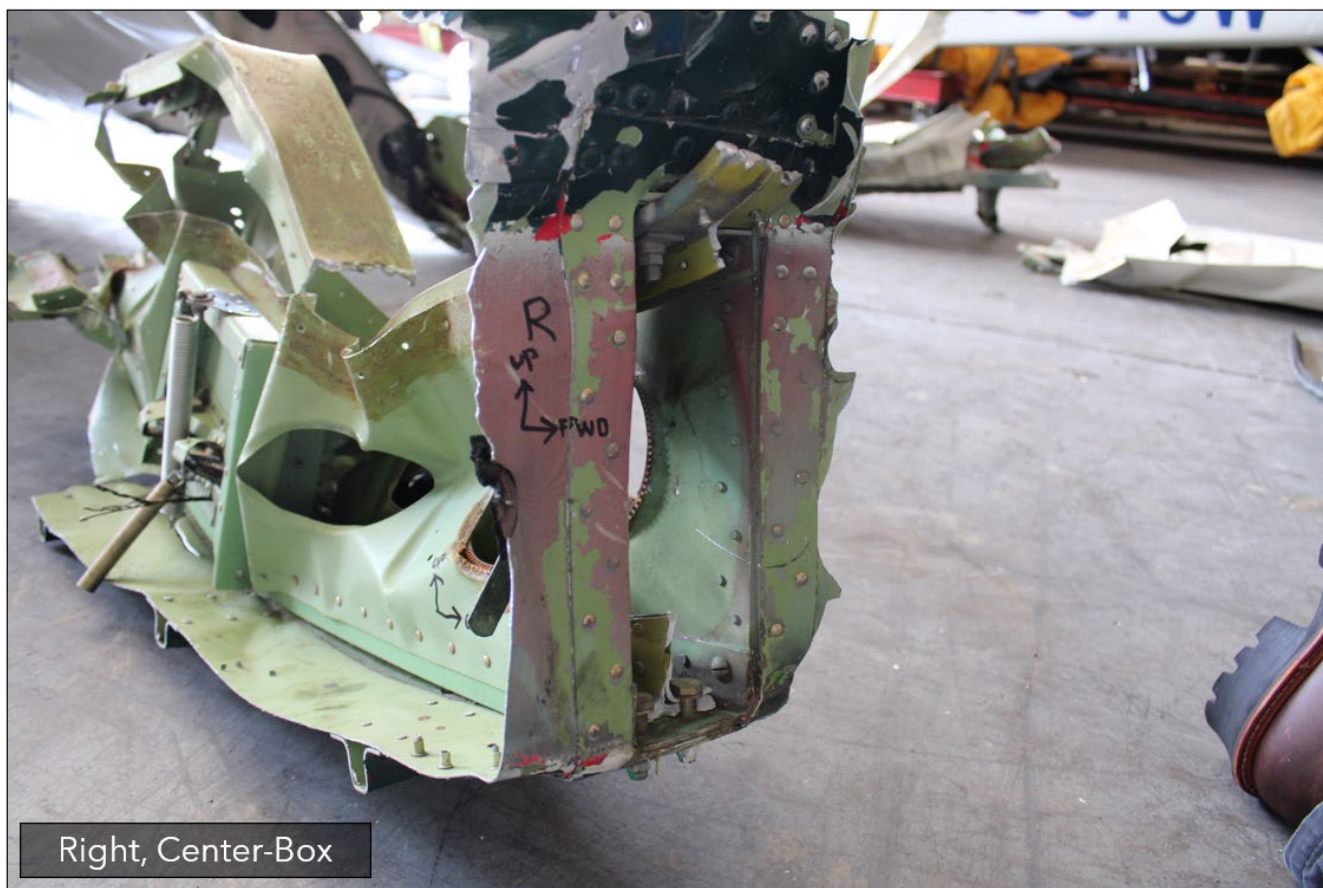
Figure 11: View of the right side of the center spar box.
