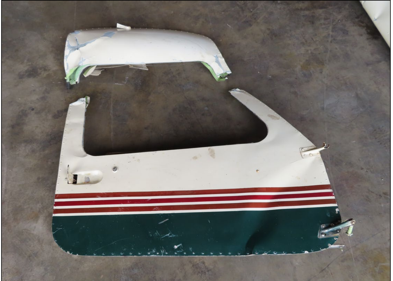
Figure 8: View of the cockpit door which had fragmented into two pieces.
