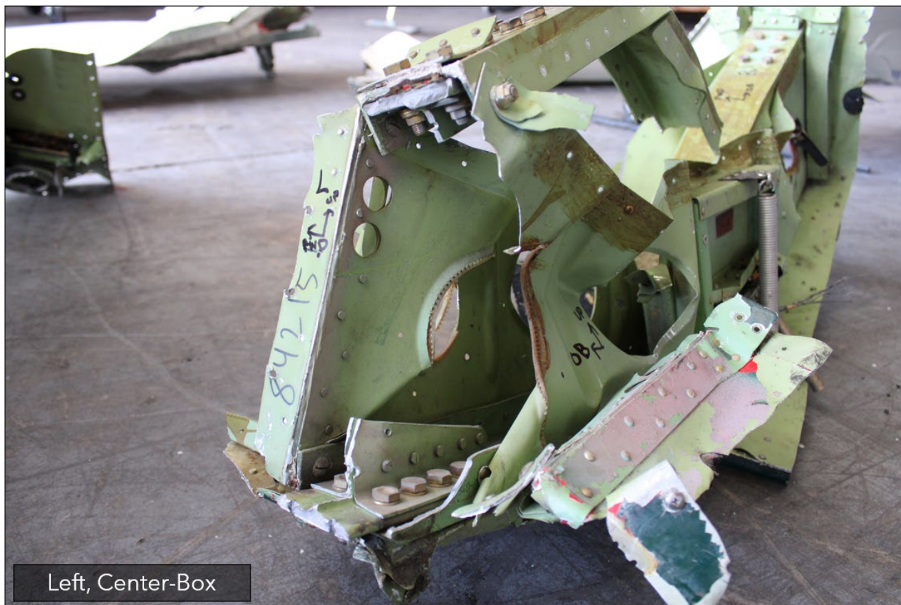
Figure 10: View of the left side of the center spar box.
