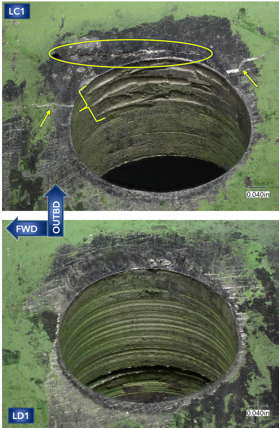
Figure 15. Oblique views of holes LC1 (upper image) and LD1 (lower image). Unlabeled arrows indicate visual crack indications emanating from the lower corner of hole LC1, and the circled crack was opened by lab fracture. A bracket indicates a series of relatively prominent circumferential imprints on the outboard side of the hole bore.
