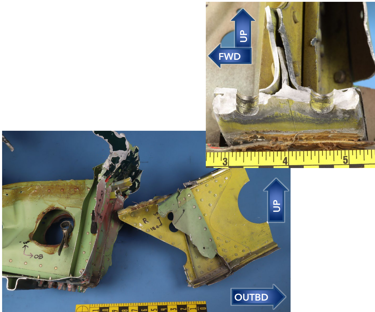
Figure 2. Right wing fracture location as viewed from the aft (lower image) and looking outboard at the outboard side of the right wing spar lower cap fracture (upper right image).
