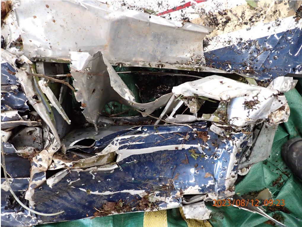
Photo 8: Left side of the horizontal stabilizer box.
