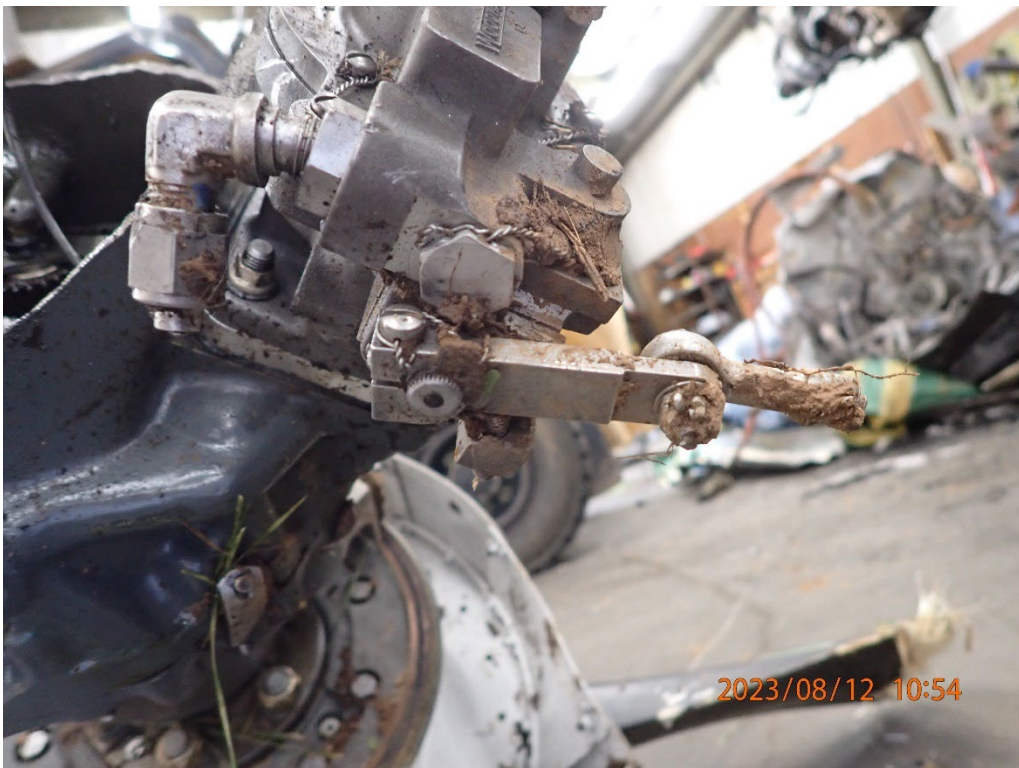
Photo 44: View of the propeller governor control with control arm head attached.
