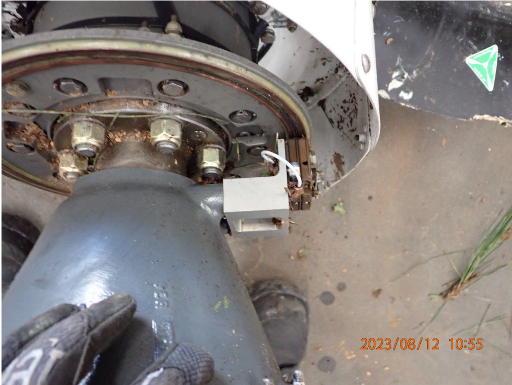
Photo 45: Propeller slip ring and brush block for electrically heated leading edge.
