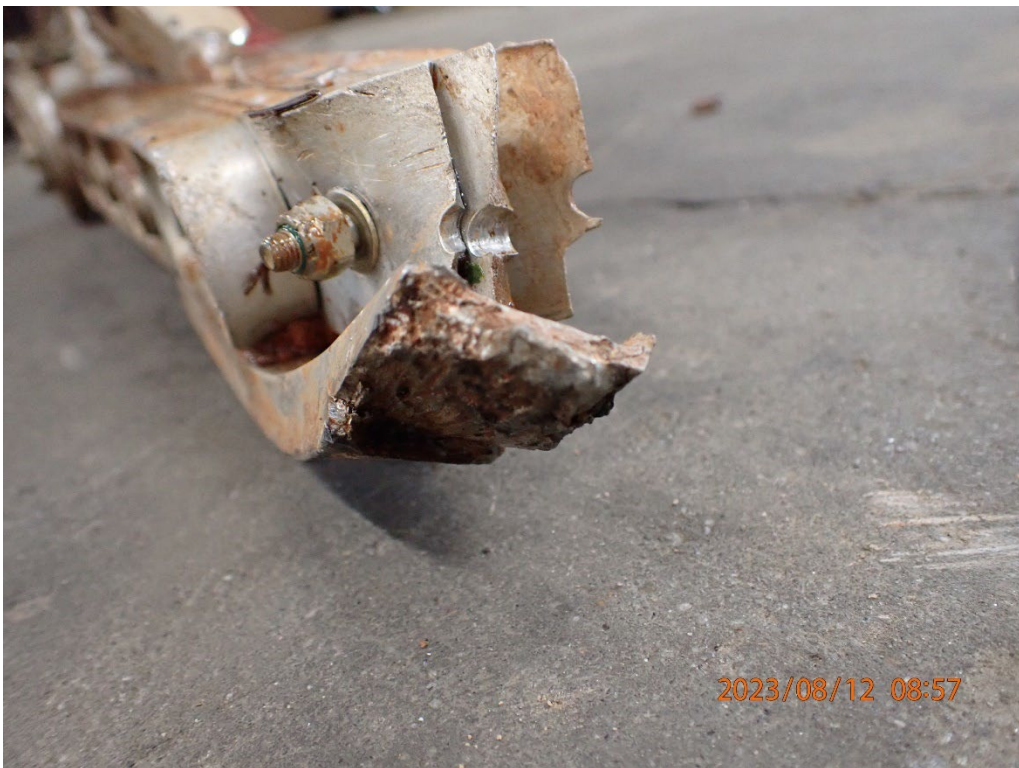
Photo 17: Bottom left wing spar cap fracture surface.
