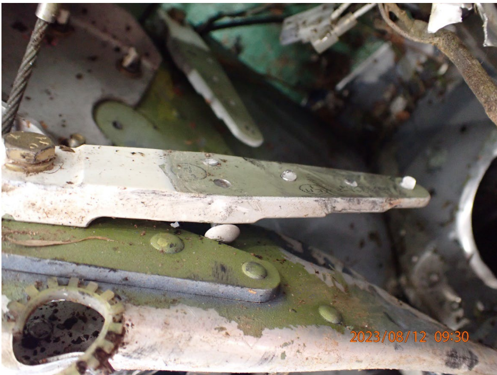
Photo 9: Horizontal stabilizer forward spar attachment points.
