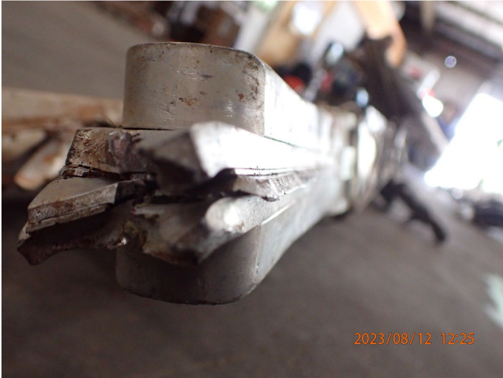
Photo 16: View of the fracture surface of the top of the left wing spar.
