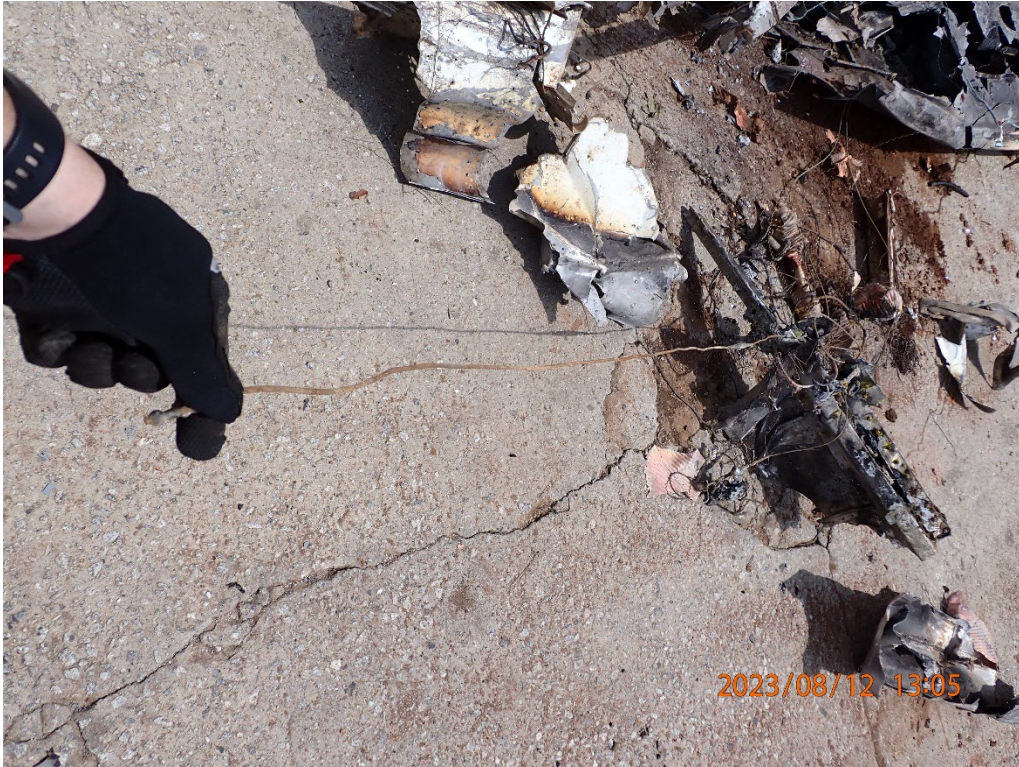
Photo 21: View of the aileron balance cable.
