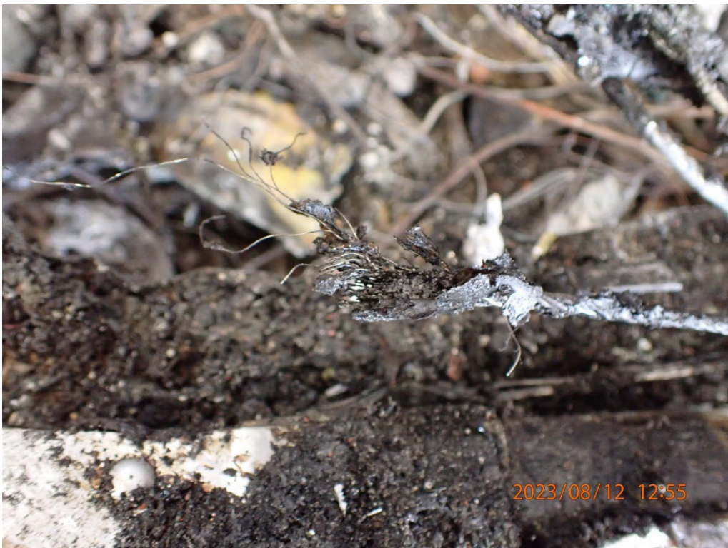
Photo 22: View of the left aileron direct control cable.
