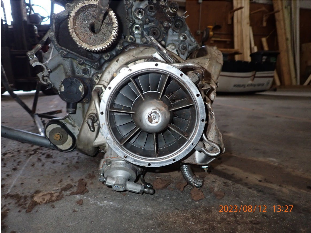
Photo 35: View of engine compressor inlet.
