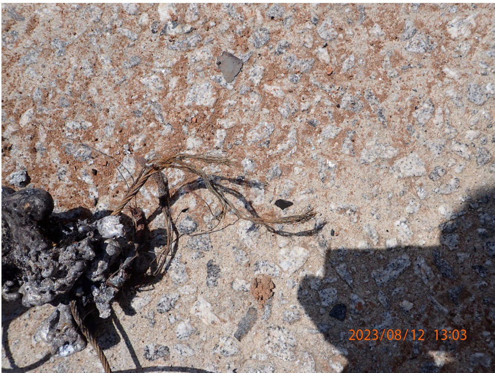
Photo 20: View of the right aileron direct control cable.
