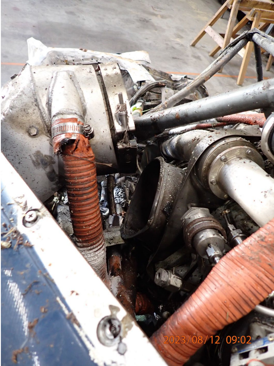
Photo 37: View of the right exhaust pipe held in place by hoses.
