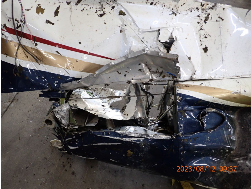
Photo 10: Right side of the horizontal stabilizer box.
