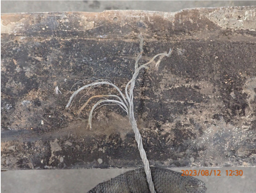
Photo 25: View of flap control cable to left wing.
