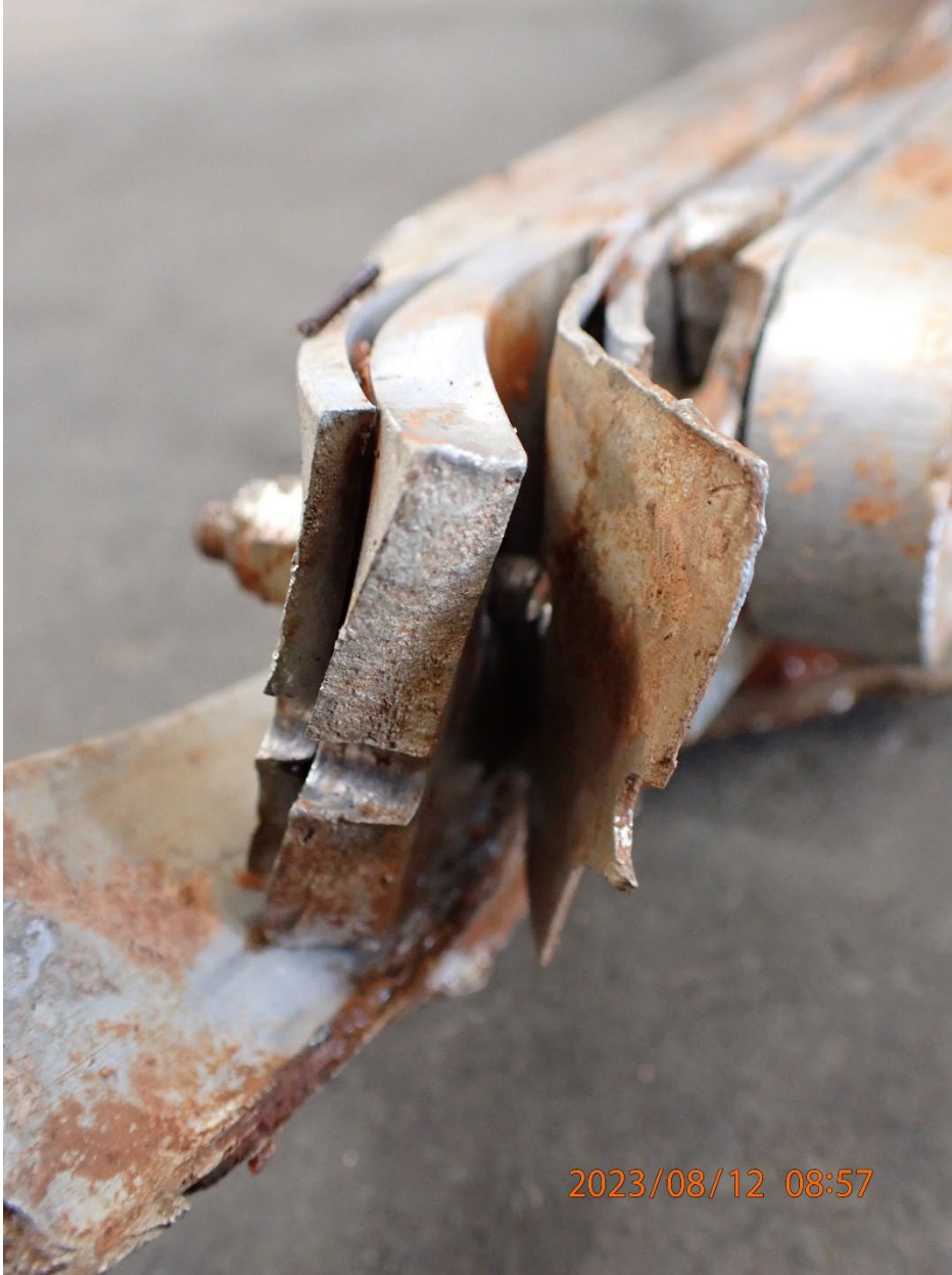
Photo 18: Bottom left wing spar cap fracture surface.
