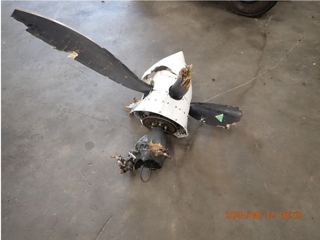
Photo 39: Propeller, propeller gear box, and governor at the recovery facility.
