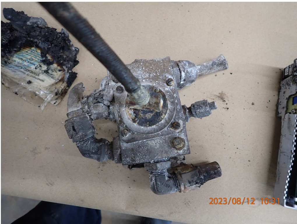
Photo 30: View of the fuel selector.
