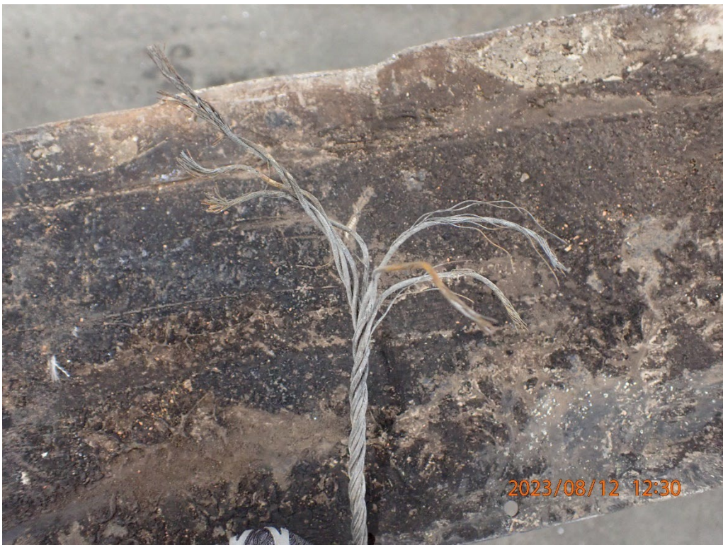
Photo 24: View of flap control cable to left wing.
