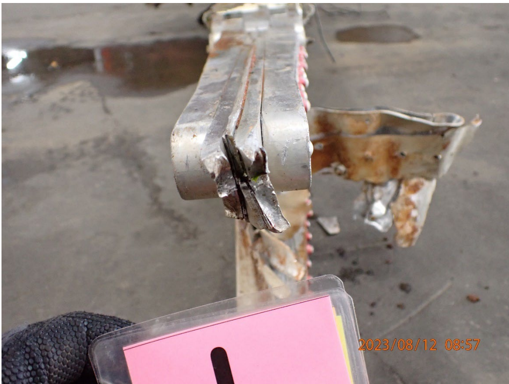
Photo 15: Top left wing spar cap fracture surface.
