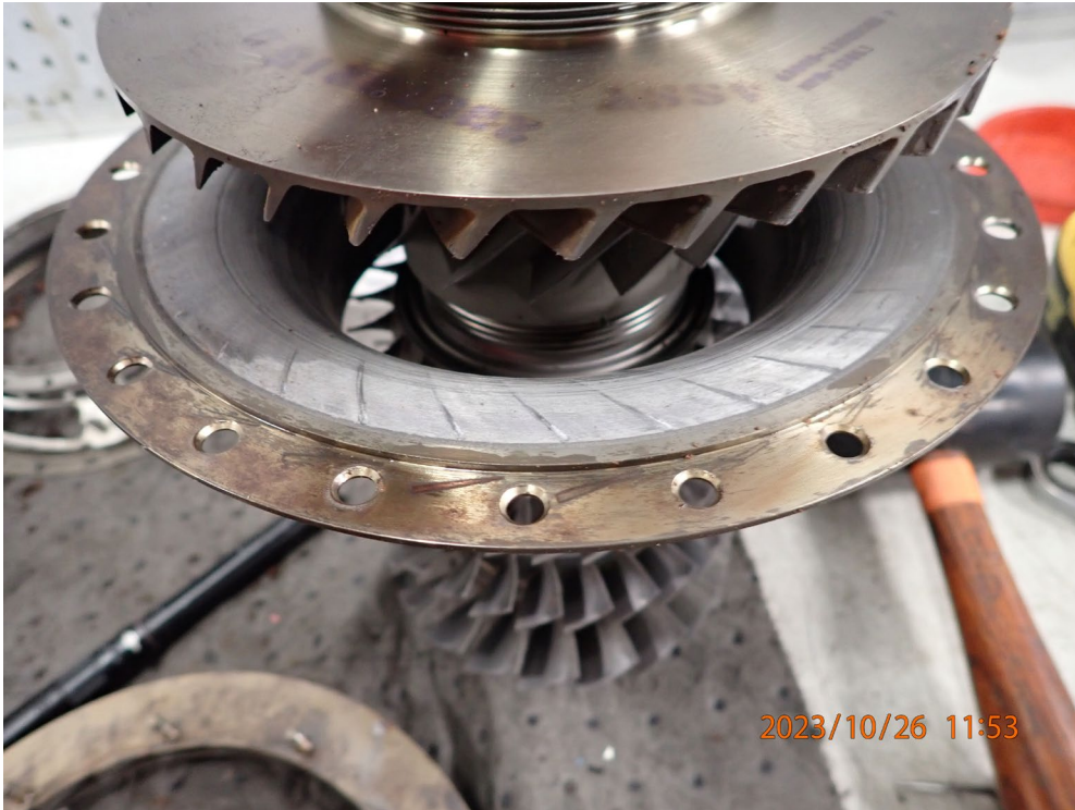
Photo 20: View of the impeller and impact gouges on the impeller shroud.
