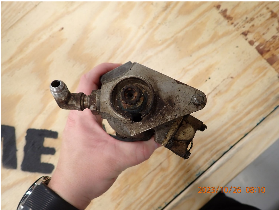
Photo 7: View of the propeller overspeed governor driveshaft.
