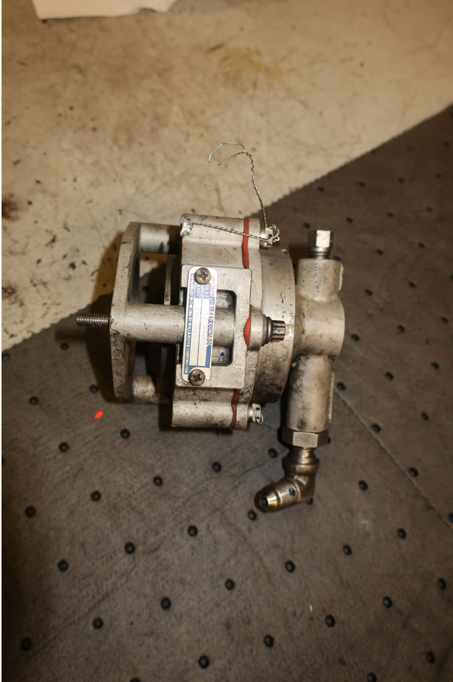
Photo 12: View of the compressor bleed valve. (Photo Courtesy of Rolls Royce)
