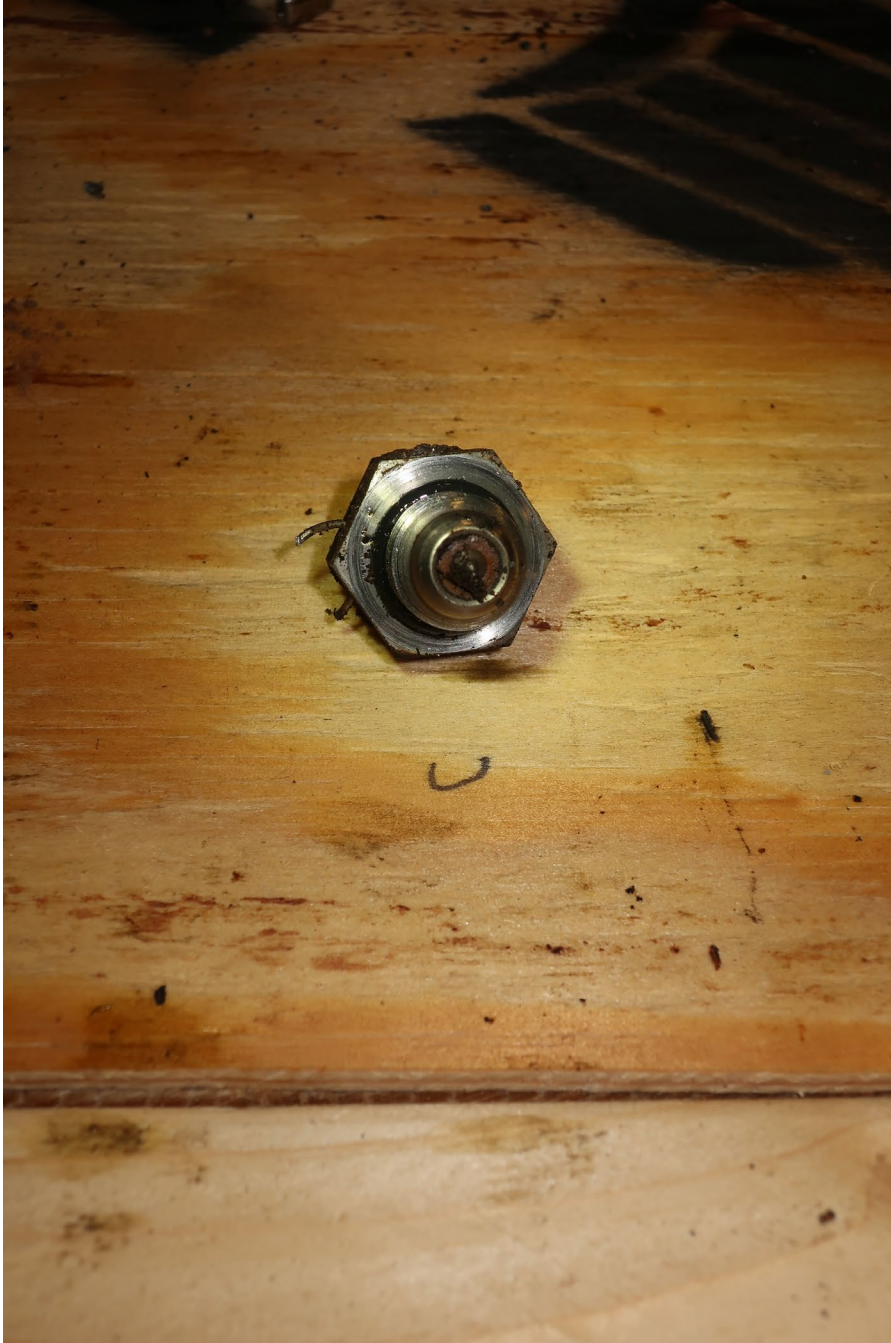
Photo 17: View of the upper MCD. (Photo Courtesy of Rolls Royce)
