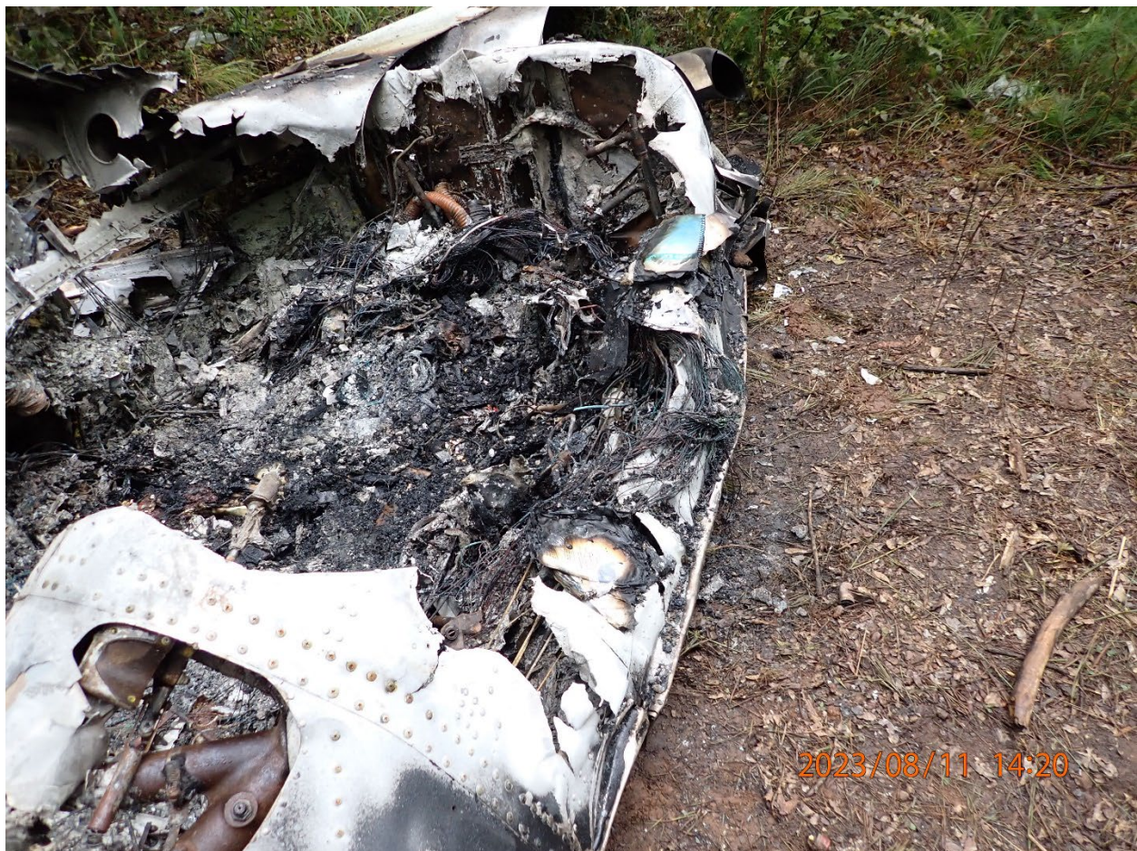
Figure 3. Photo taken from the accident showing the damaged cockpit where the Garmin GTN 750Xi avionics box is housed.
