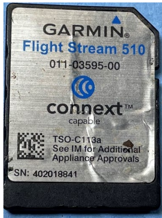
Figure 2. Undamaged Garmin Flight Stream 510 SD card containing no flight data.
