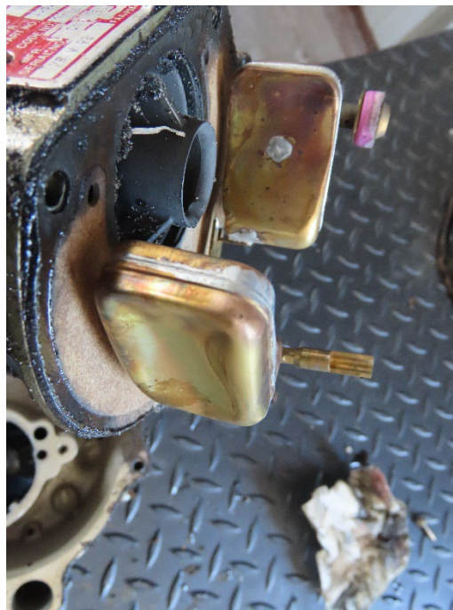
Figure 5 Fuel floats showing evidence of fluid deformation; The opposing side showed the same type of deformation.
