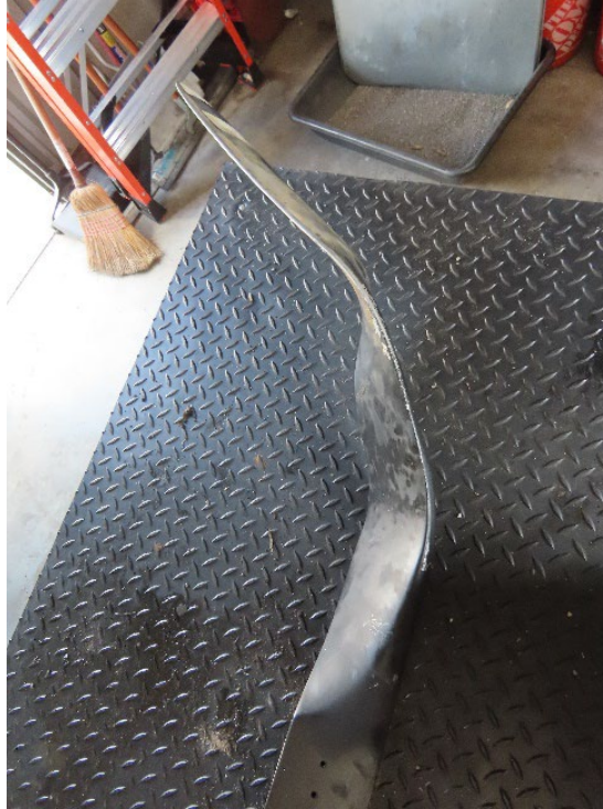
Figure 7 McCauley propeller exhibiting signs of s bending and polishing.
