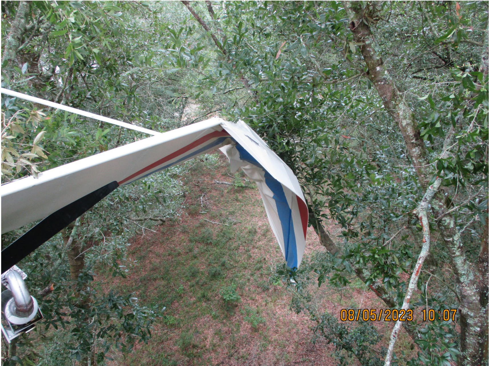
Photo 3 – left wing tip damaged
