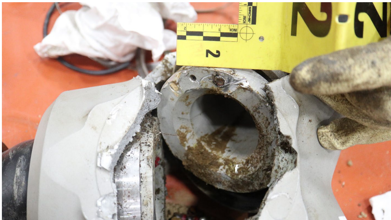
Photo 9: View of the root of blade 2. (McCauley Photo)
