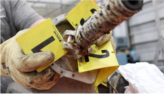
Photo 3: View of broken actuator links. (McCauley Photos)
