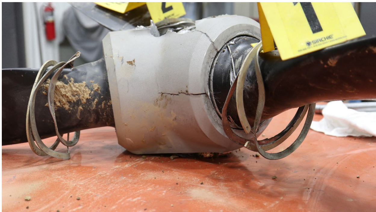
Photo 5: View of fractures to the No. 1 blade socket. (McCauley Photo)
