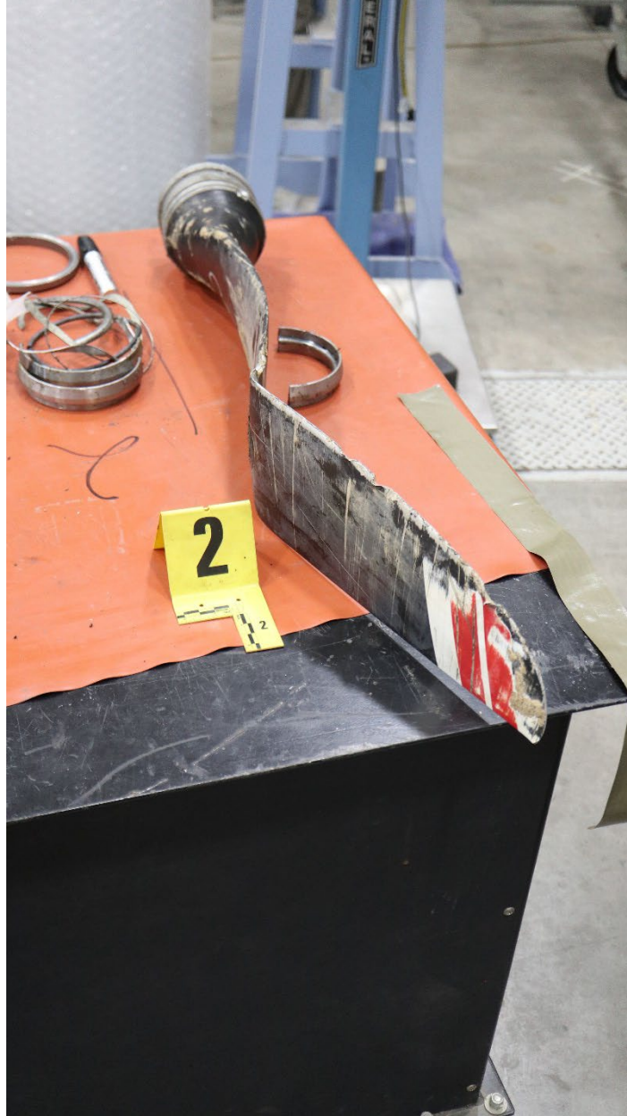
Photo 13: View of the leading edge of blade 2. (McCauley Photo)
