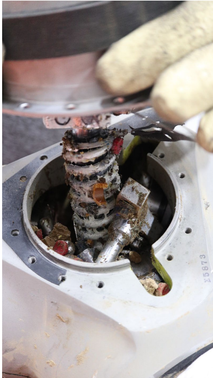
Photo 2: Removal of the blade actuation piston and spring assembly. (McCauley Photo)
