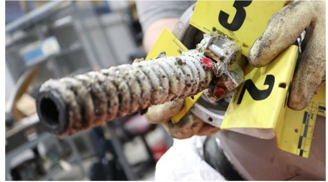
Photo 3: View of broken actuator links. (McCauley Photos)
