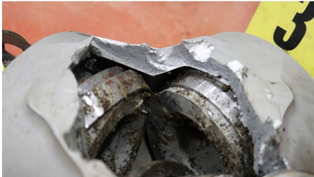
Photo 7: View of rear hub fracture surfaces. (McCauley Photos)
