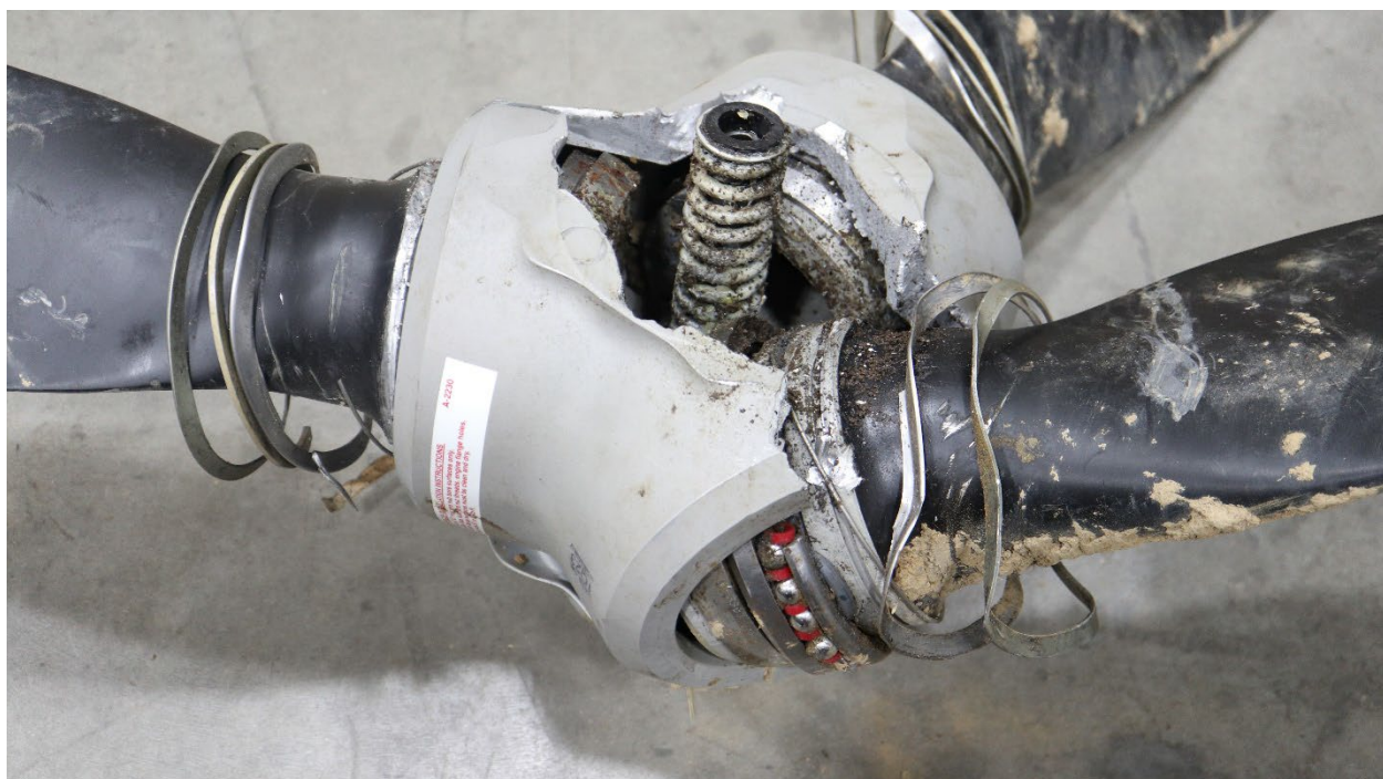
Photo 6: View of the rear hub and missing rear quarter of blade socket No. 2. (McCauley Photo)
