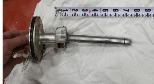
Photo 4: View of deformations to the actuator piston rod. (McCauley Photos)
