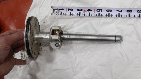
Photo 4: View of deformations to the actuator piston rod. (McCauley Photos)
