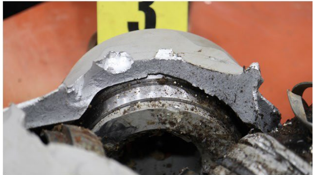
Photo 7: View of rear hub fracture surfaces. (McCauley Photos)
