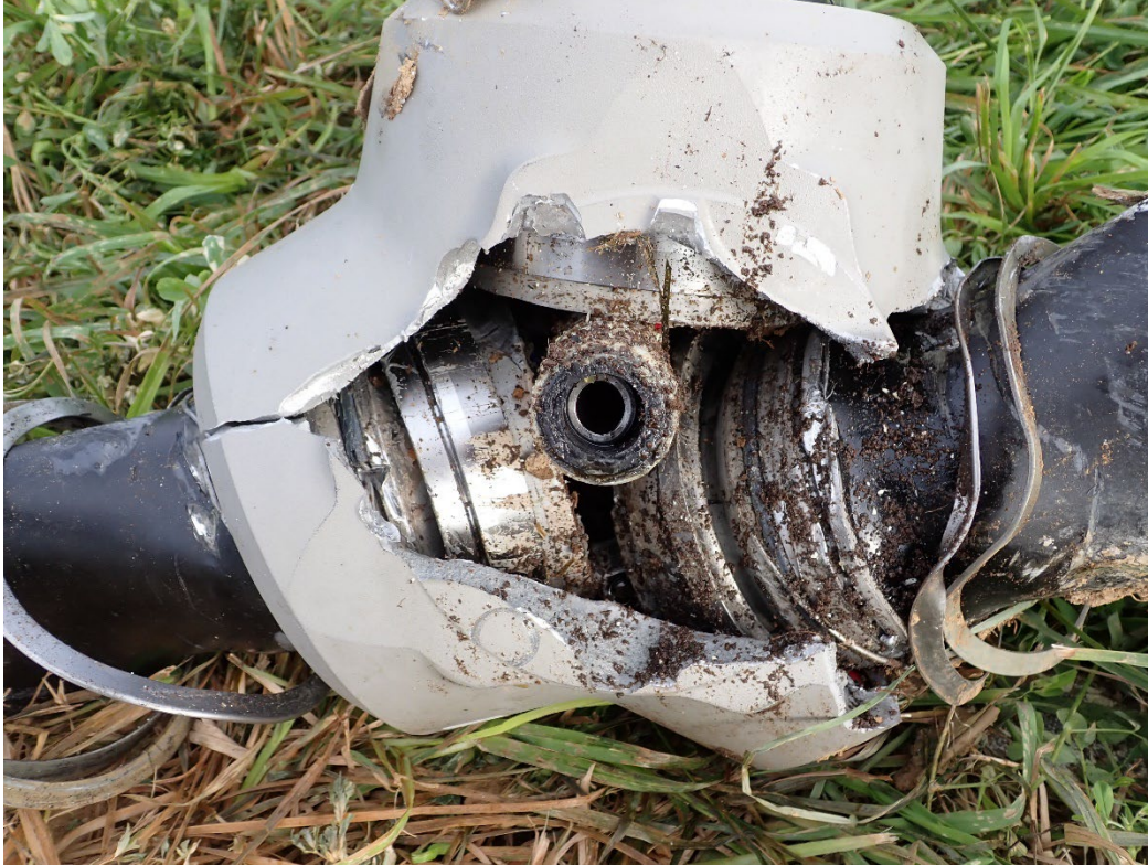
Photo 42: View of damage to the propeller hub.
