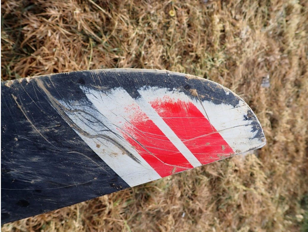
Photo 45: Blade "A" leading edge gouging, chordwise scratching, and polishing. Blade A
