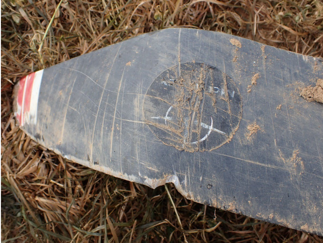
Photo 51: Blade "C" leading edge gouging and chordwise scratching.
