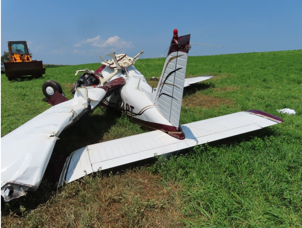
Photo 9: View of crush damage to the leading edge of the left wing. (Piper Photo)
