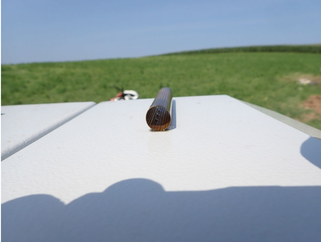
Photo 38: Oil suction screen.
