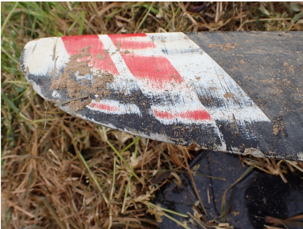
Photo 48: View of leading edge gouging and chordwise scratching, blade "B."
