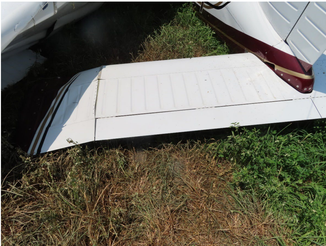
Photo 7: View of damage to the left stabilator tip. (Piper Photo)
