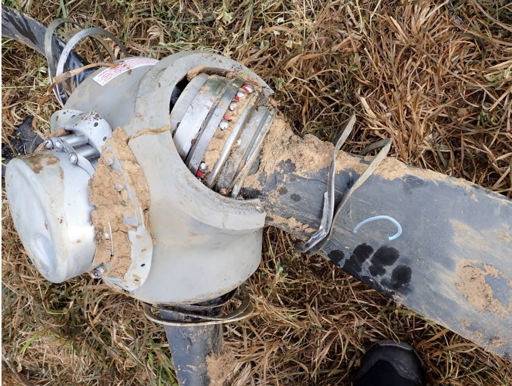
Photo 49: Damage to the propeller hub, blade "C."
