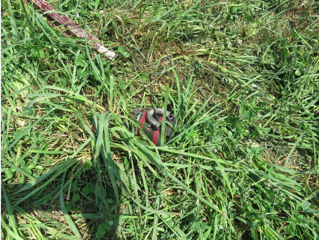
Photo 39: View of the vacuum pump impact separated from the engine. (Lycoming Photo)
