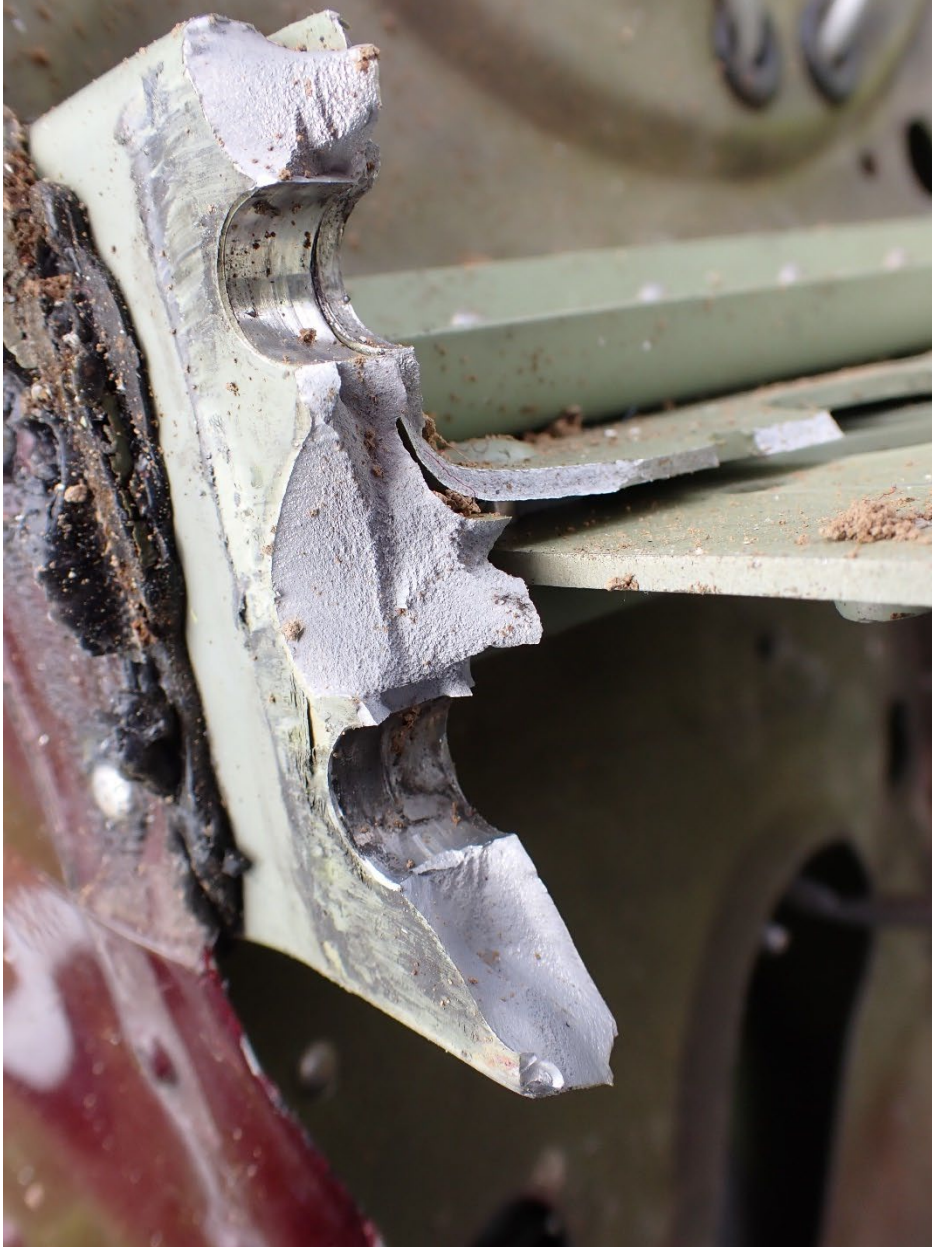
Photo 11: Left main spar fracture.
