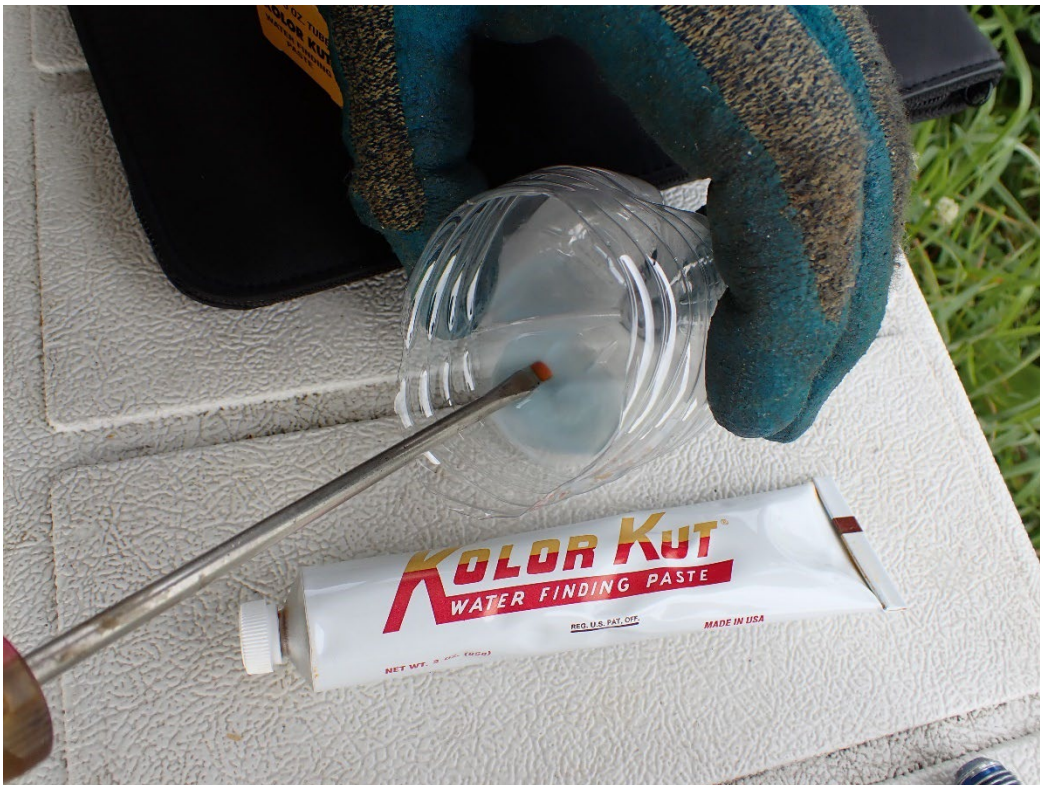
Photo 24: Fuel being tested with water finding paste.
