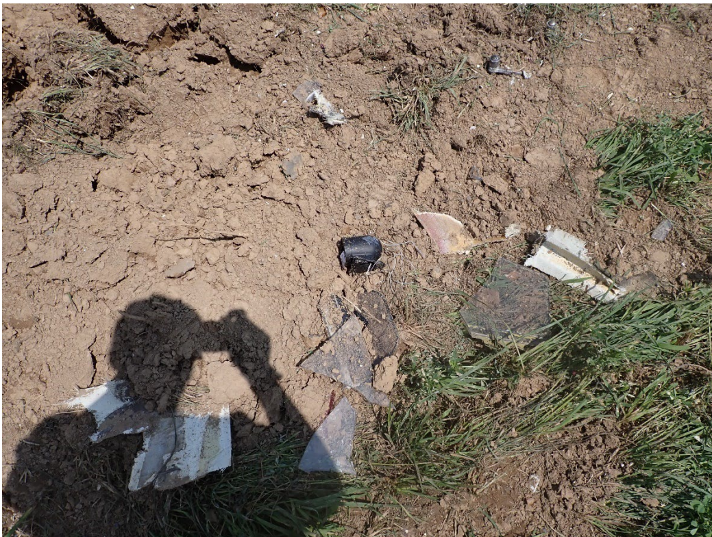
Photo 21: View of the magnetic compass impact separated from the glareshield.
