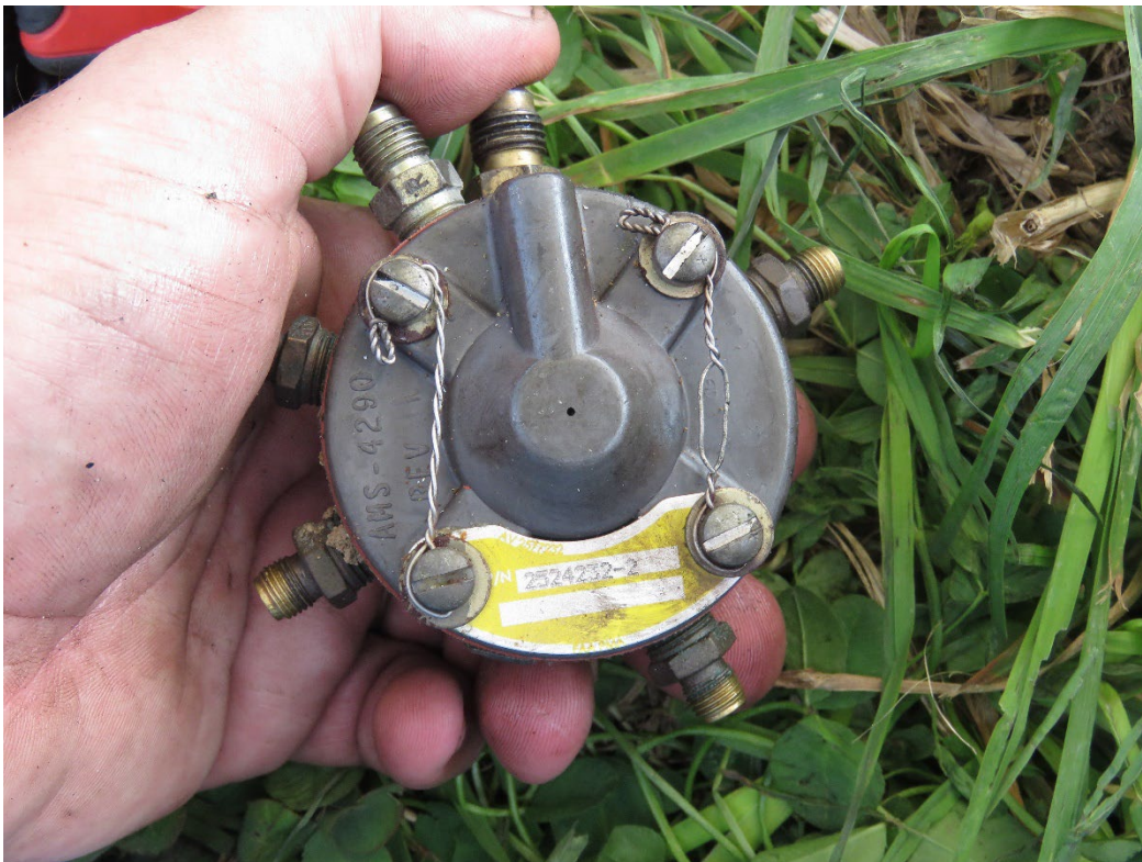
Photo 36: View of the flow divider. (Lycoming Photo)
