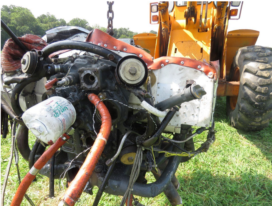
Photo 37: View of the oil filter attached to the accessory case. (Lycoming Photo)
