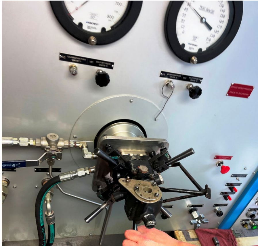
Photo 8: View of the governor installed on the test stand. (Hartzell Photo)
