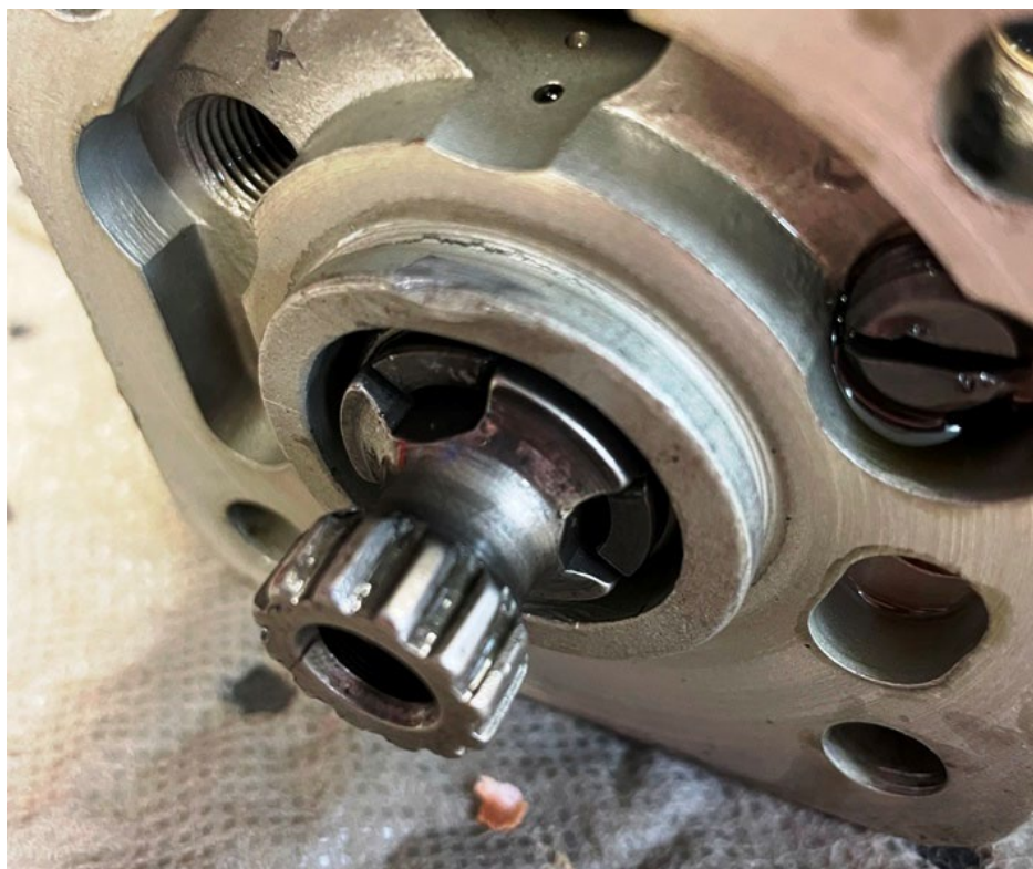
Photo 4: View of impact damage to the governor pilot flange. (Hartzell Photo)
