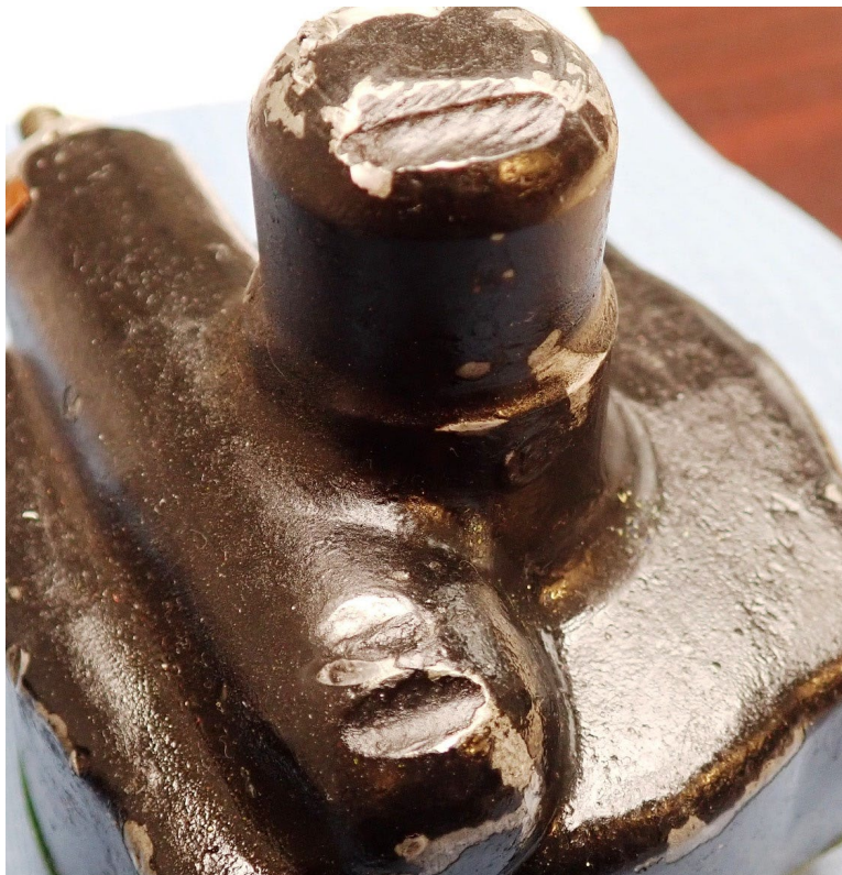
Photo 3: Gouging/wear on the governor head. (Hartzell Photo)
