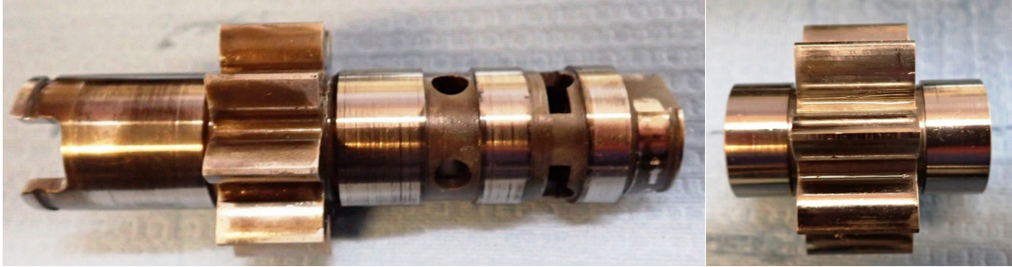
Photo 15: Governor oil pump gears. (Hartzell Photo)
