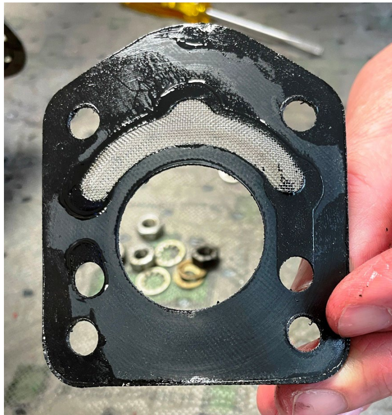
Photo 6: Base and gasket/screen as received. (Hartzell Photo)
