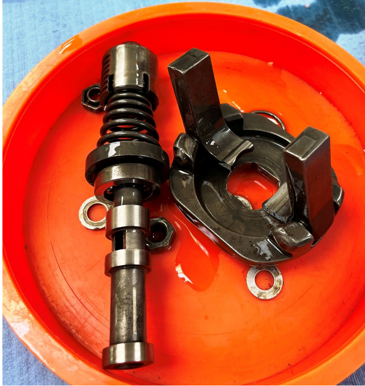
Photo 13: Governor spool, speeder spring, and flyweight unit components. (Hartzell Photo)
