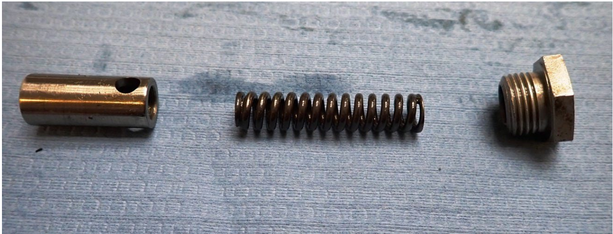
Photo 14: Pressure relief valve components. (Hartzell Photo)
