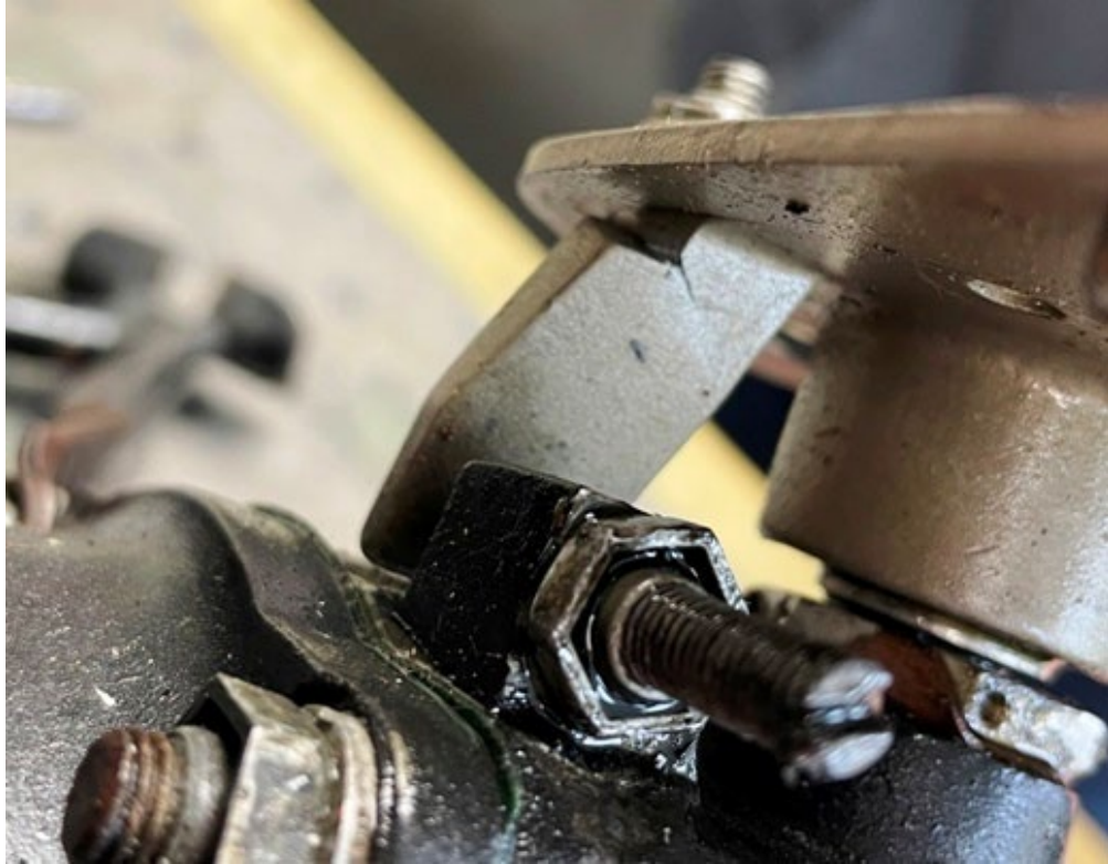
Photo 2: View of bent/fractured high RPM stop post. (Hartzell Photo)
