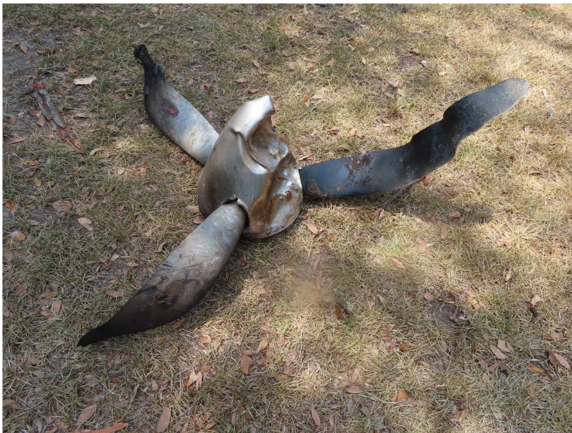
Photograph 5 - View of damaged three-bladed propeller.
