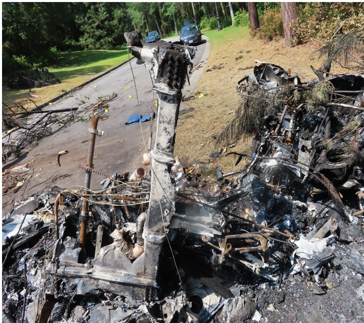
Photograph 3 - View of fire damaged fuselage.
