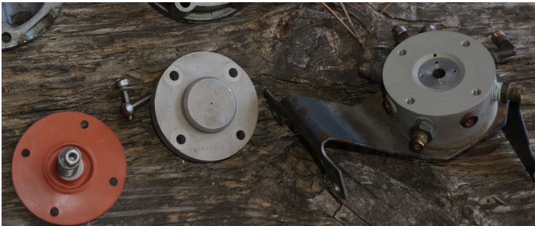
Photograph 21 - Left Engine Fuel Manifold
