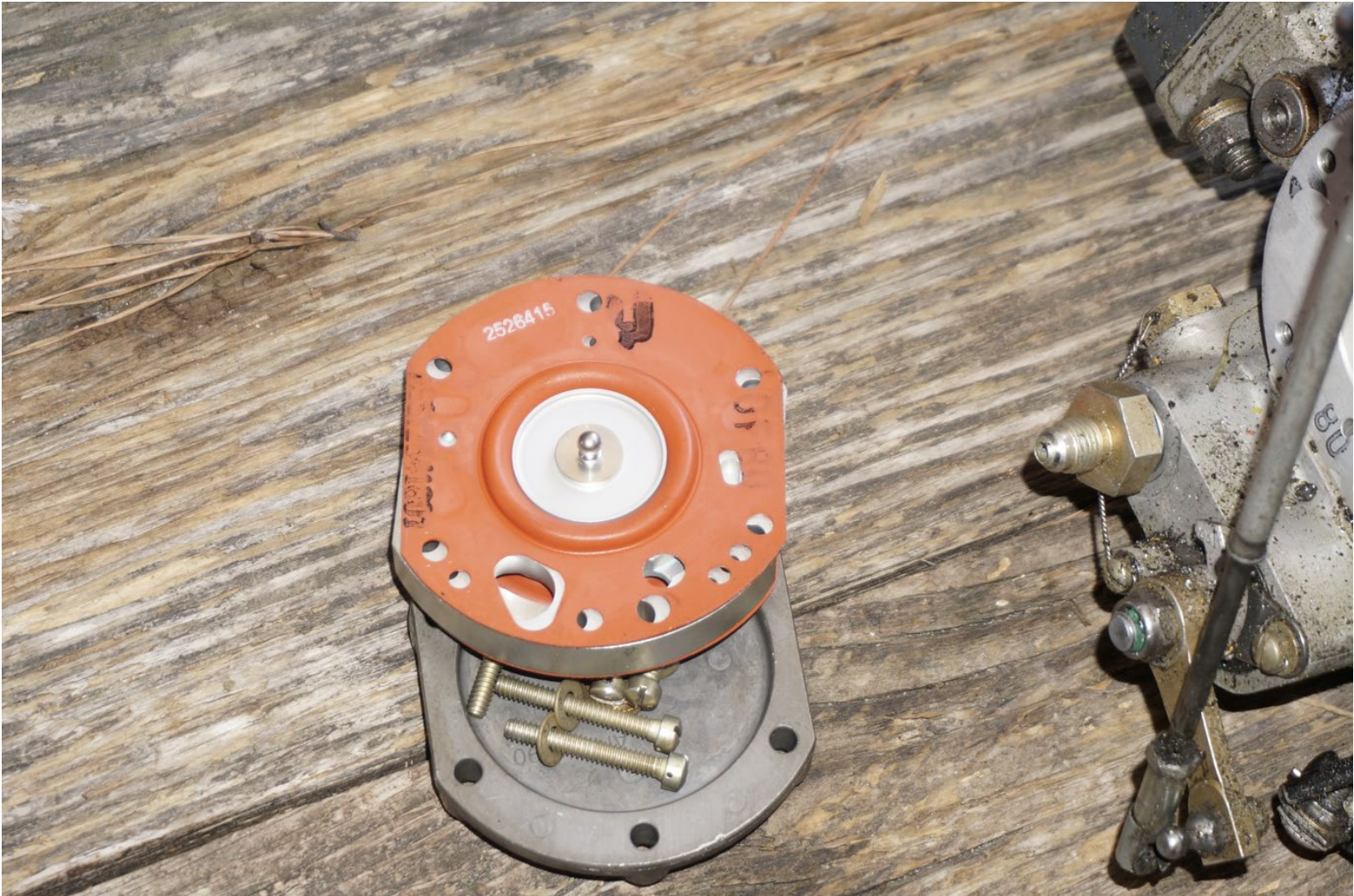
Photograph 20 - Left Engine Fuel Servo Diaphragm
