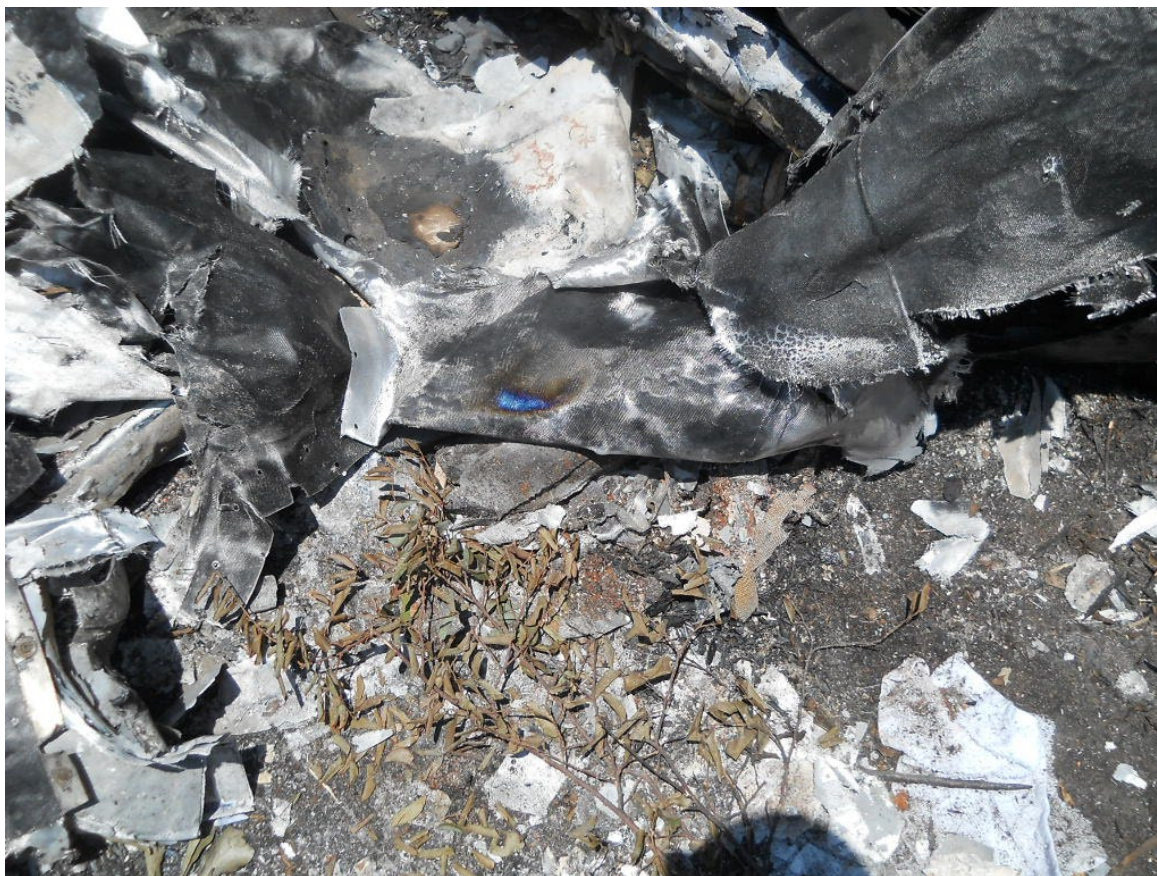
Photograph 7 - Blue Staining Below Engine
