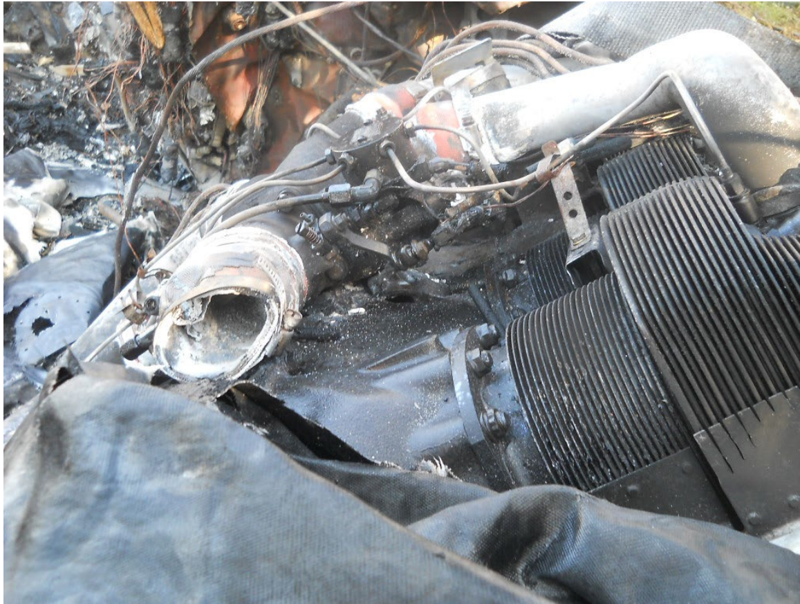
Photograph 5 - Hole in Top of Crankcase
