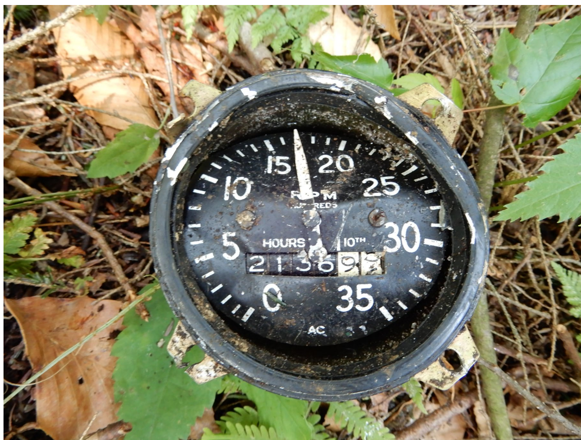
Photograph 10 - Engine Tachometer (NTSB Photo)
